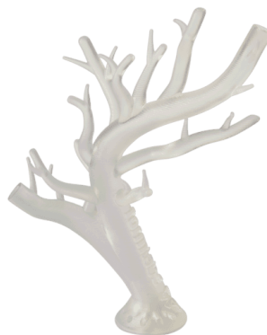
Figure 9: An artery model printed from Formlabs Elastic 50A Resin [24], [25]
