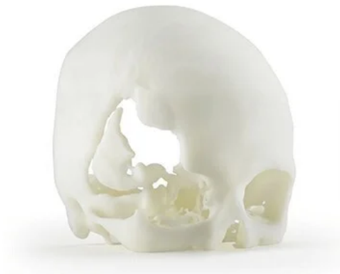
Figure 8: Human skull fragment printed from Stratasys ABS M30i Resin ( i indicates the biocompatible version of the material) [23]
