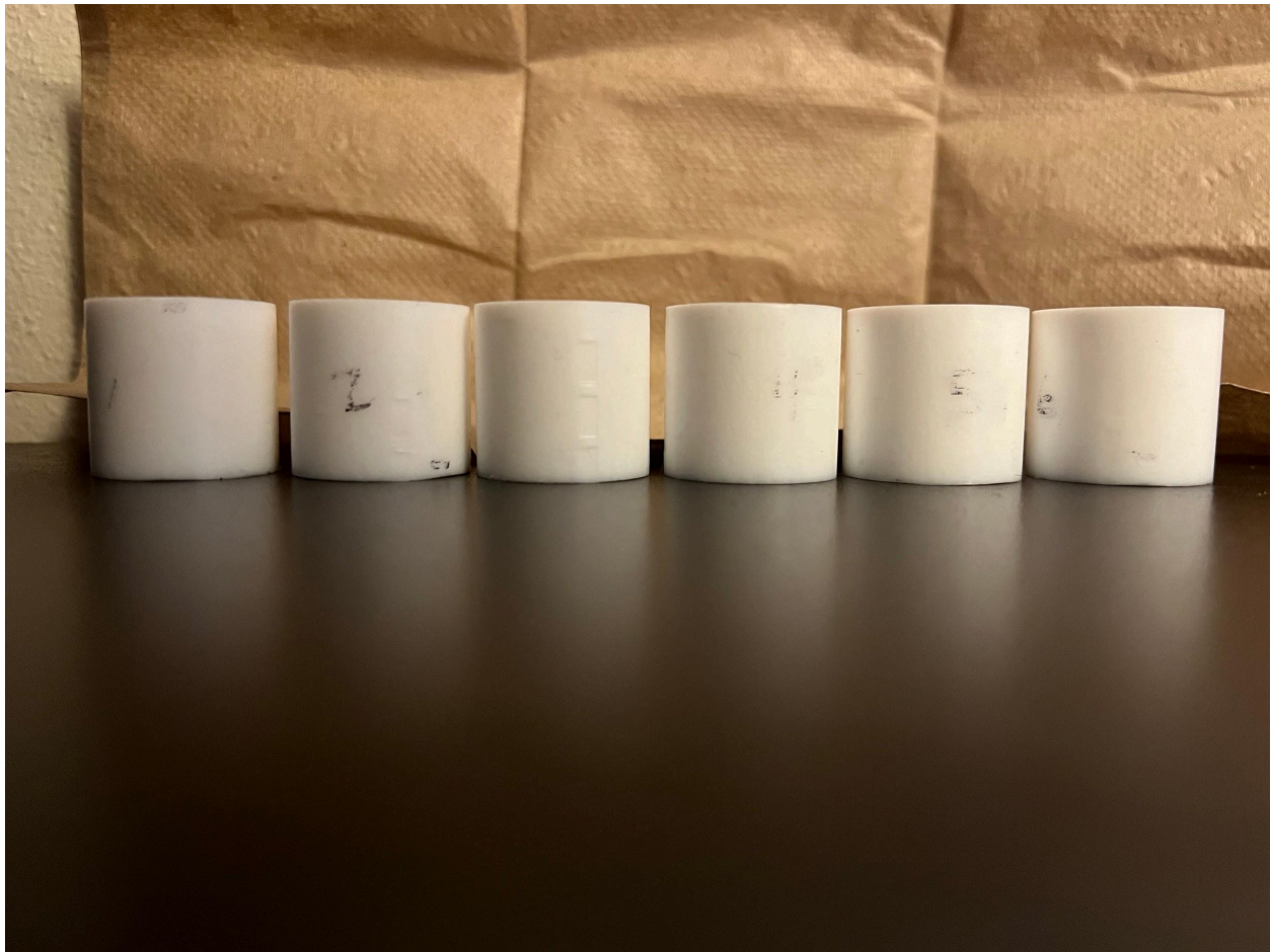
Figure 2: All six PTFE pillars after cutting and drilling side-by-side to visualize their height similarity.
