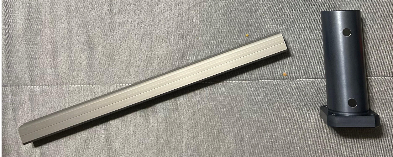
Figure 1: 0.33m of 20mm square hard-anodized aluminum shaft and Drylin Q square twin flange bearing (twice the height of what is required).
