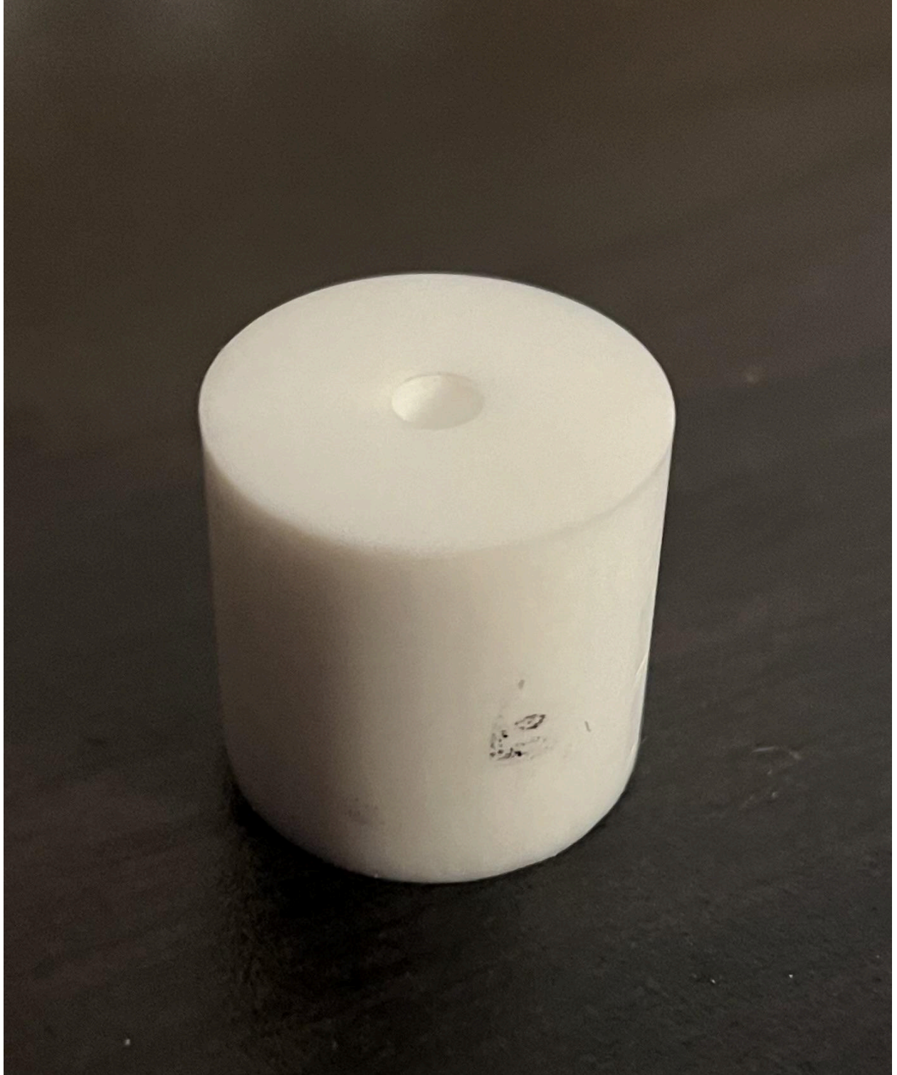
Figure 2: One individual PTFE pillar with the M5 hole shown.
