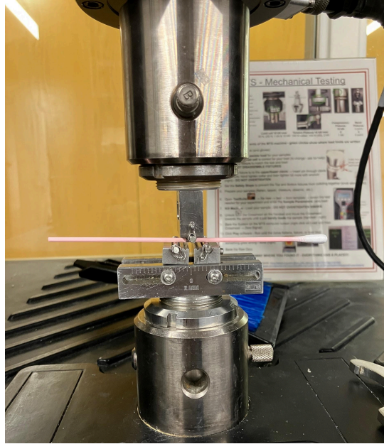
Figure 14: The pink swab placed in the MTS machine in the three point bend configuration.
