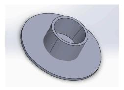
This component is a base to house the Aptima tube while the patient conducts the test.
