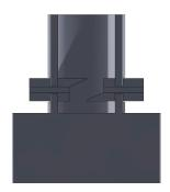
This design is a potential solution to breaking the swabs. There are two edges that actuate to apply pressure and bend the swab. If enough force is applied to the swab it will break at the already perforated section.
