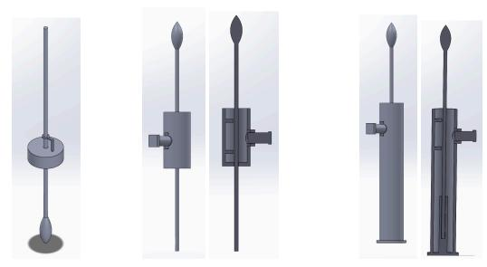
The leftmost design simply attaches to the Aptima tube over the threads, then the patient applies pressure to snap the swab and break the small support, which allows for the snapping of the swab to be contained within the tube.
