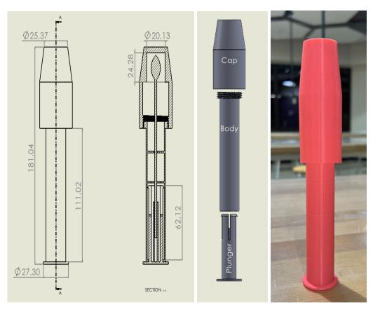
The current design was developed last semester and includes a plunger, body and cap. The prototype was 3D-printed and assembled with the plunger being inserted into the bottom of the body, and the cap screws onto the top of the body. A swab is inserted through the body and into the plunger.
