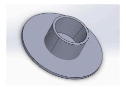
This component is a base to house the Aptima tube while the patient conducts the test.
