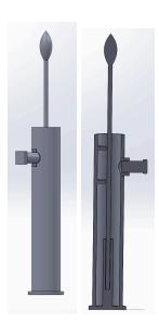
The left design utilizes 3-point bending to break the swab and uses a button to apply a central force at the swab perforation.
