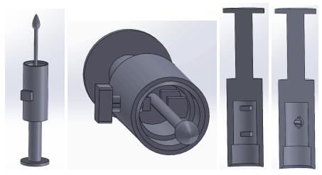
This design uses a 3-point bending mechanism to break the swab. When the patient is done swabbing, they press the device onto the uncapped Aptima tube and push the button to break the
