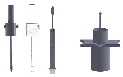
We came up with some new designs to overcome the obstacle of the media tube. These involve a handle for the swab and a mechanism to cleave the swab at the perforation that is modeled after a cigar cutter. These images are a few different preliminary ideas for how this could look.
