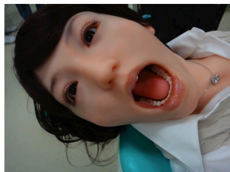
Figure 1. The Showa Hanko 2 robotic dental test dummy.
