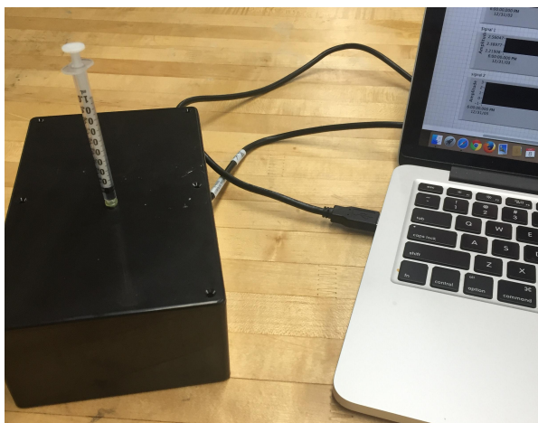
Figure 15: Final box enclosure. Syringe attaches at top of box and sends a diluted blood sample through tubing and the microchannel
