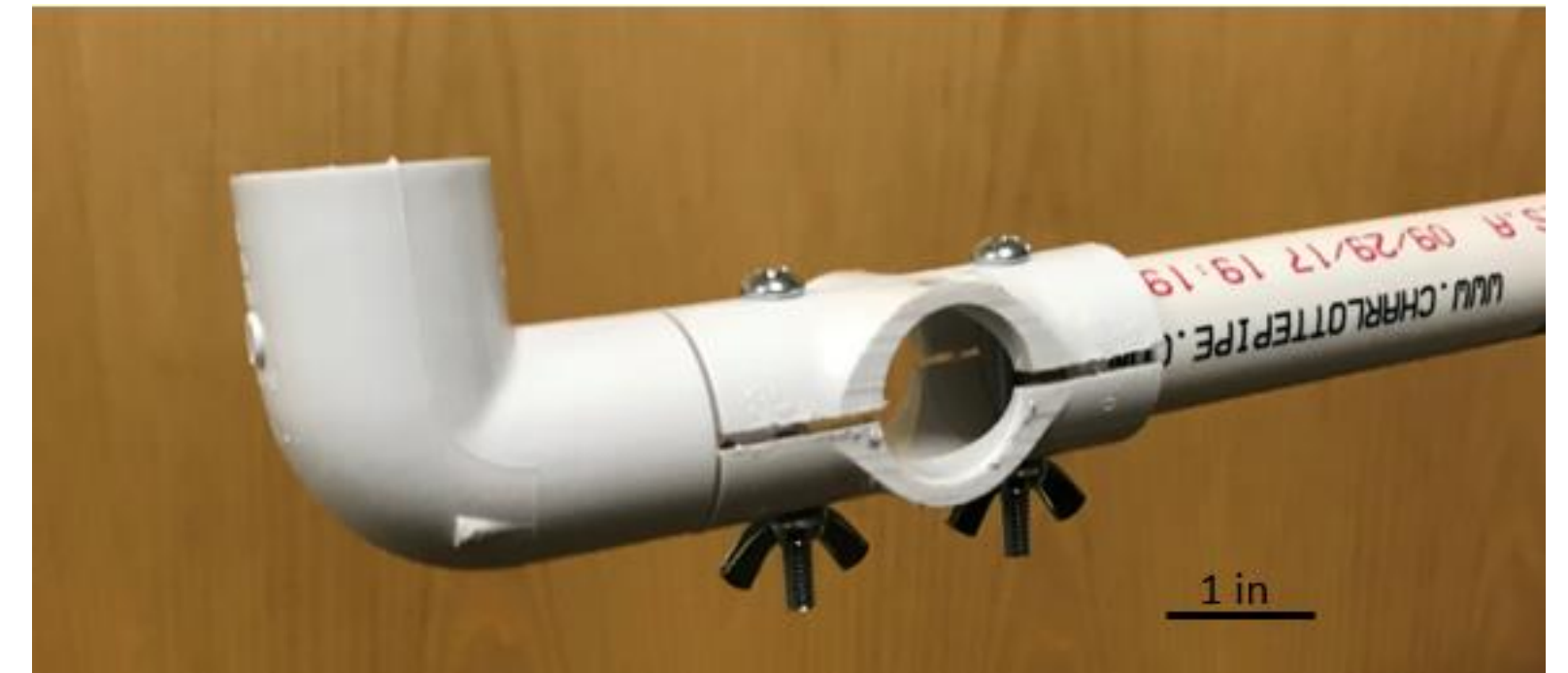
Figure 6. The attachment part that attaches the device to the wheelchair
