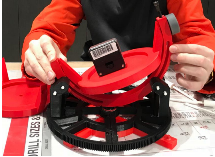
Figure 2: Past UW Madison BME design team's solution; presents 3 degrees of rotational freedom but limited internal translational freedom; extensive gearing prevents facile sterilizability; prototype 3D printed [5]
