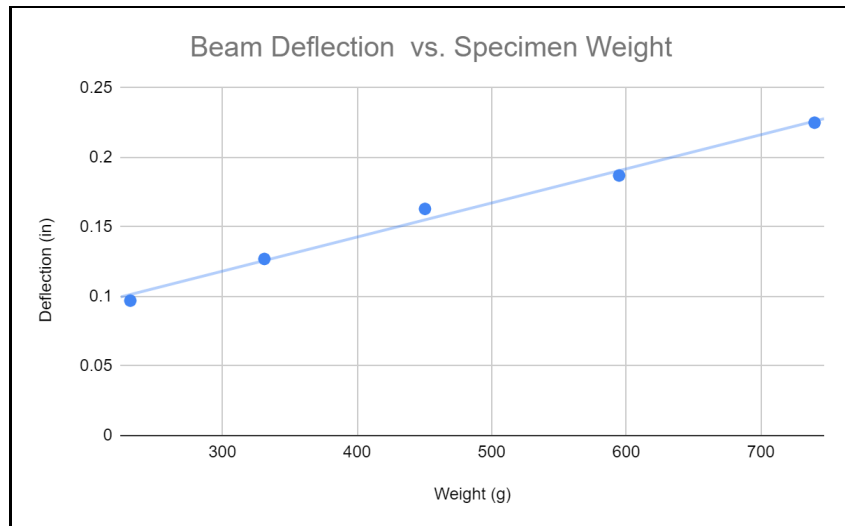
Figure 10: 10 inch (25.4 cm) translational rod deflection under various loads; deflection in inches plotted against weight loading the universal stage; universal stage positioned 5 inches from the base of the rods.
