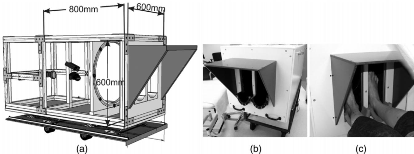
**Fig. 2** The experimental setup for foot scanning: (a) the schematic of the experimental setup with two cameras installed, which are the thermal camera (upper) and the RGB camera (lower). (b) The appearance of the experimental set and (c) positioning of patients' feet during measurement.
