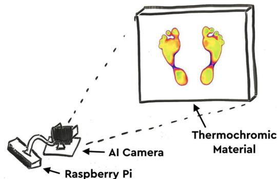
*Figure 2. Design 1, depicting thermochromic mat and AI camera + raspberry pi*
