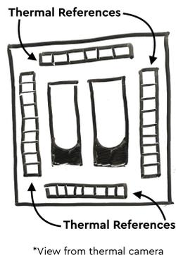
*Figure 4. Camera view showing the thermal references*
