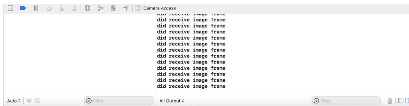
Figure 21. The testing results of outputting the frame. The message pop up at the same time the application is opened on the iPhone, which means the delay for getting the frame is minimal
