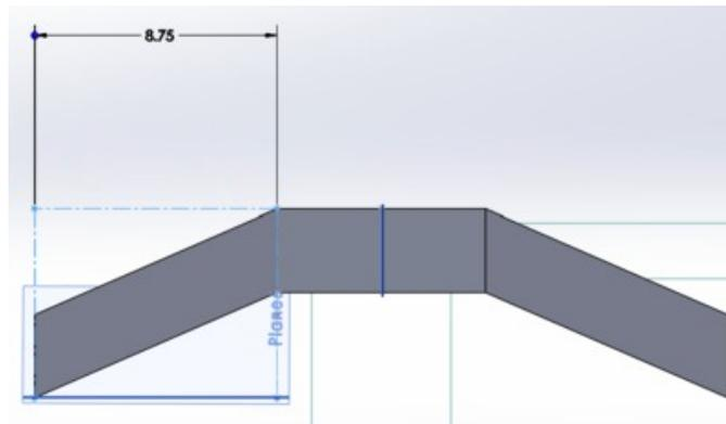
EPPERhinge5.png(28.7 KB) - [download](#) Figure 10: Front view of the hinge showing arm dimensions
