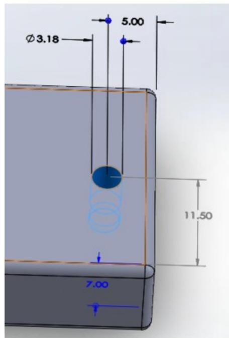
EPPERhandle5.png(40 KB) - [download](#) Figure 5: Top-side view of the handle showing the dimensions of the hole for the screw.
