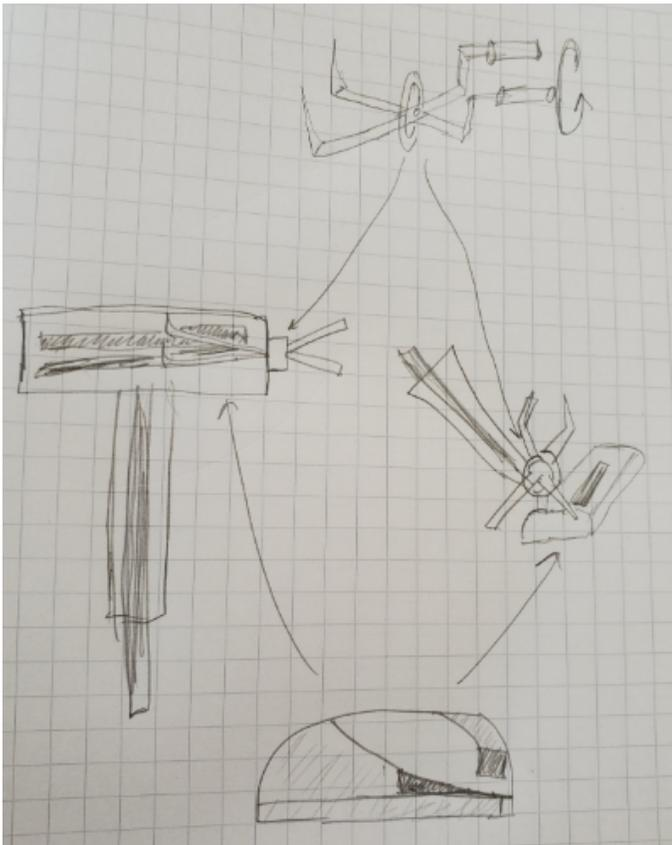
The design has a handle for grip, a blade area with safety guards, and a clamp crank to hold the skin and increase the tension. As the epidermis is cut, the clamp rolls the loose skin so tension can still be applied.
