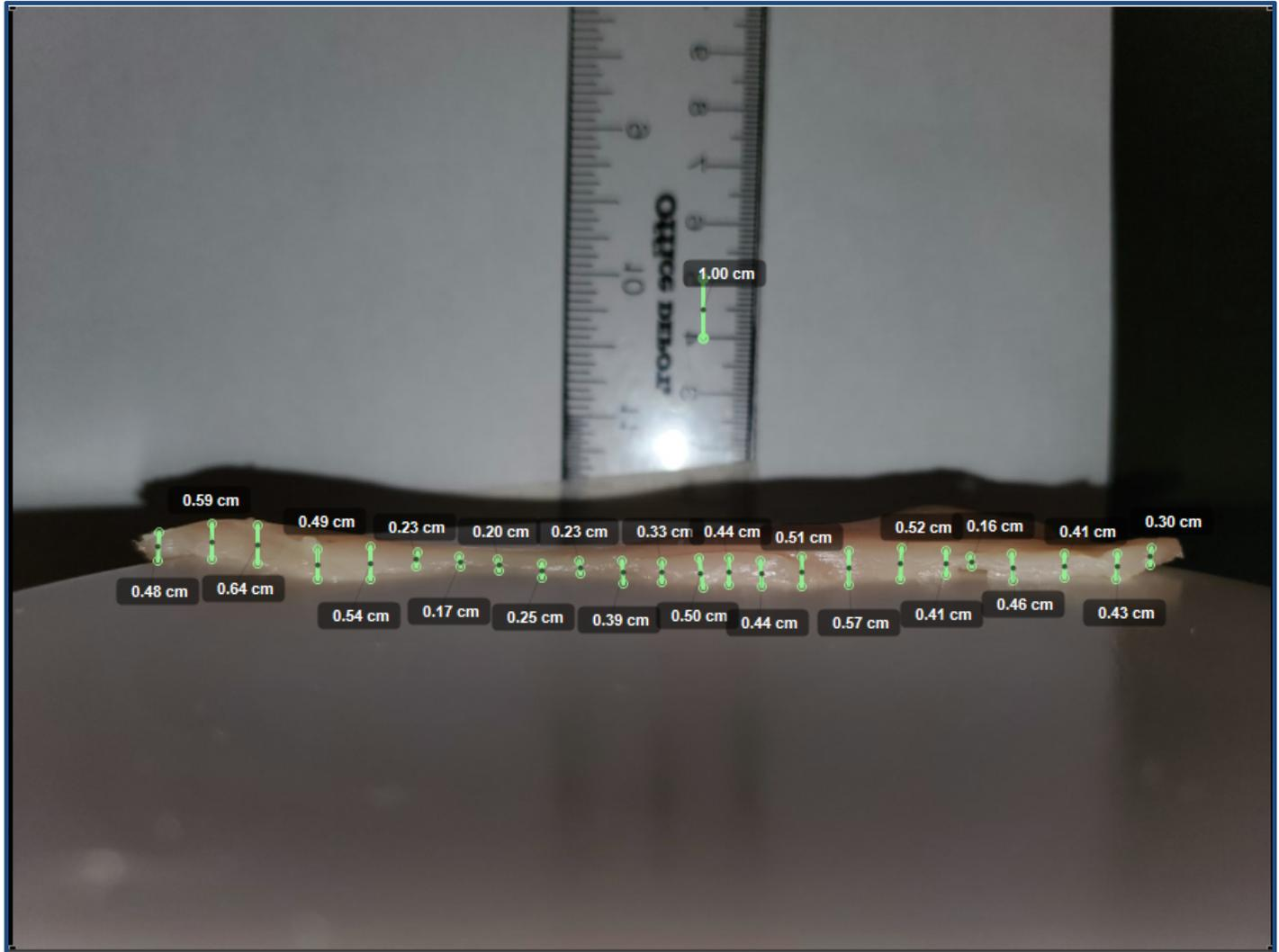
Figure 5 (above): Kinovea analyzed strip of cut chicken. 24 cut depth data points were collected from the cut of chicken shown in the testing page using Kinovea's calibration tool
