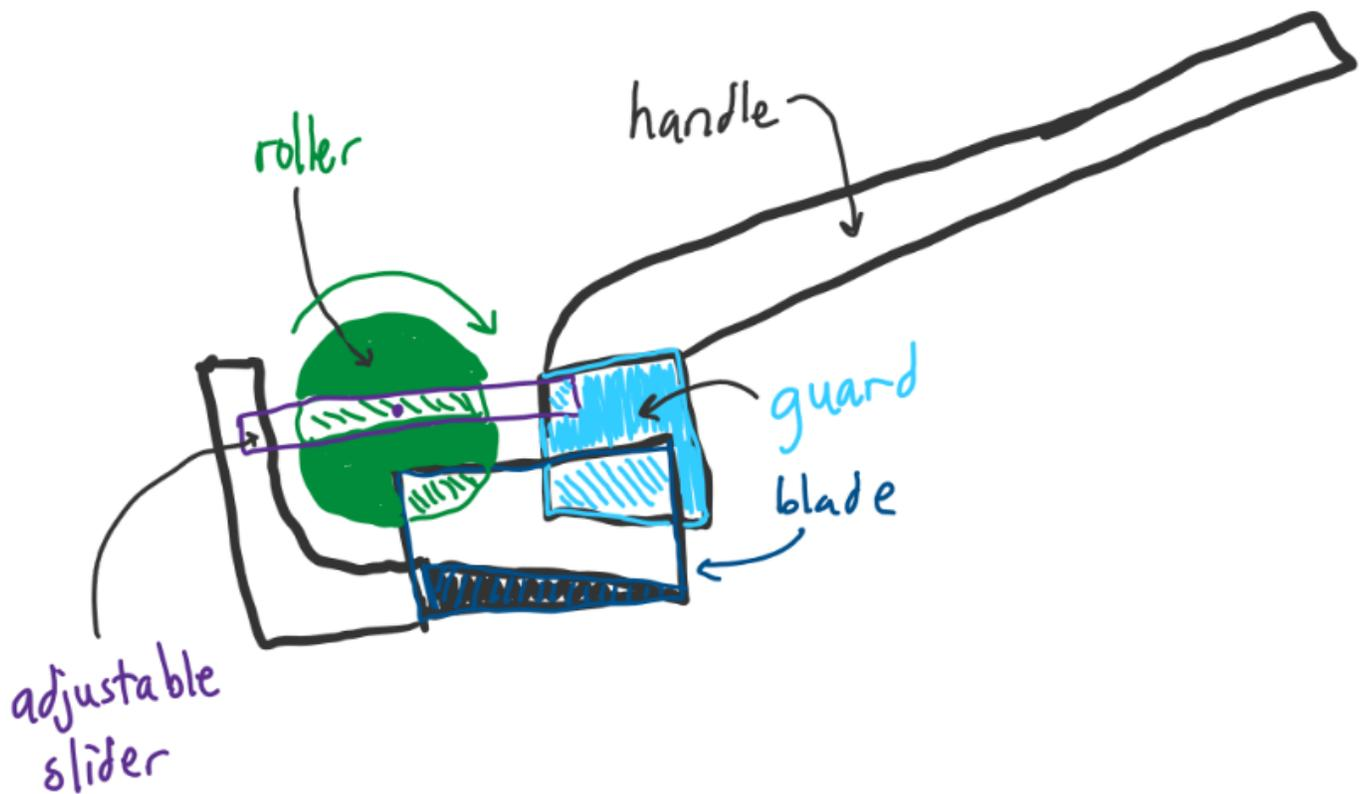
Above is a design combining the shovel design idea from Noah and the roller design from Michael. It has the same structure as the shovel but an added roller in top for increased tension on the loose skin. There will be an adjustable slide for the roller depending on the thickness of the skin needed to cut off. This was drawn in OneNote
