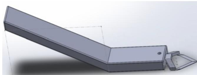
**EPPERboth2.1.png(150.7 KB) - download** Figure 3: The modified EpiCut with the blades added to the hinge part
