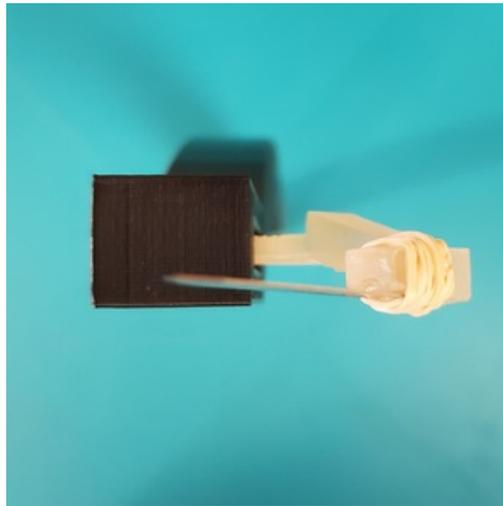
**20201202\_124957.jpg(912 KB) - download** Figure 4: The High Temp prototype with one of the arms with the blade attached to it, inserted into the handle. This is a front view with the blade pointing out of the picture. The position of the blade shows that the prototype cannot be used for testing because the blade is above the bottom of the handle.
