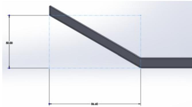
**EPPERhandle2.png(86.5 KB) - download** Figure 2: Side view of the handle showing the measurements of the angled portion
