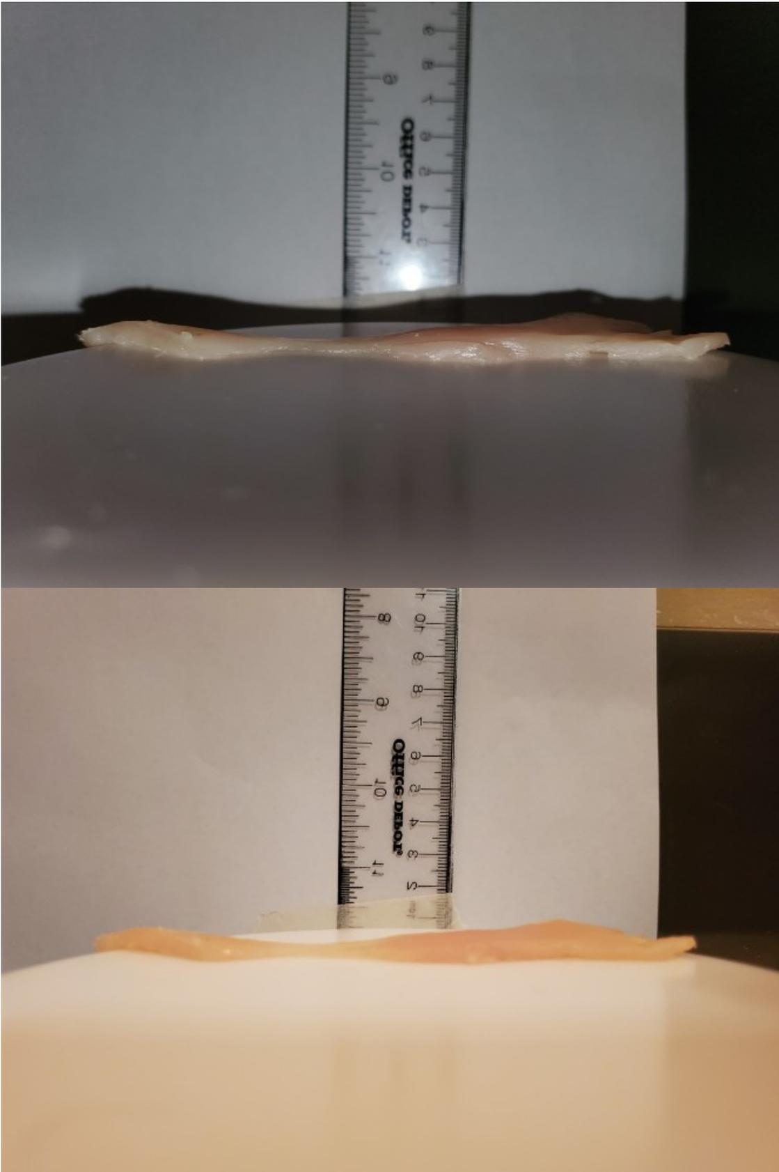
**Figure 1:** These are the same sample of chicken breast that was analyzed in Kinovea to test for cut depth.
