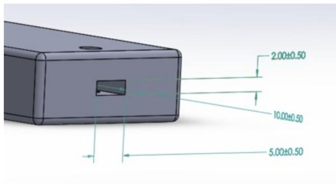
**EPPERhandle4.png(31.6 KB) - download** Figure 4: An oblique front view to show the hole and the dimensions where the hinge part of the modified Epicut will go in
