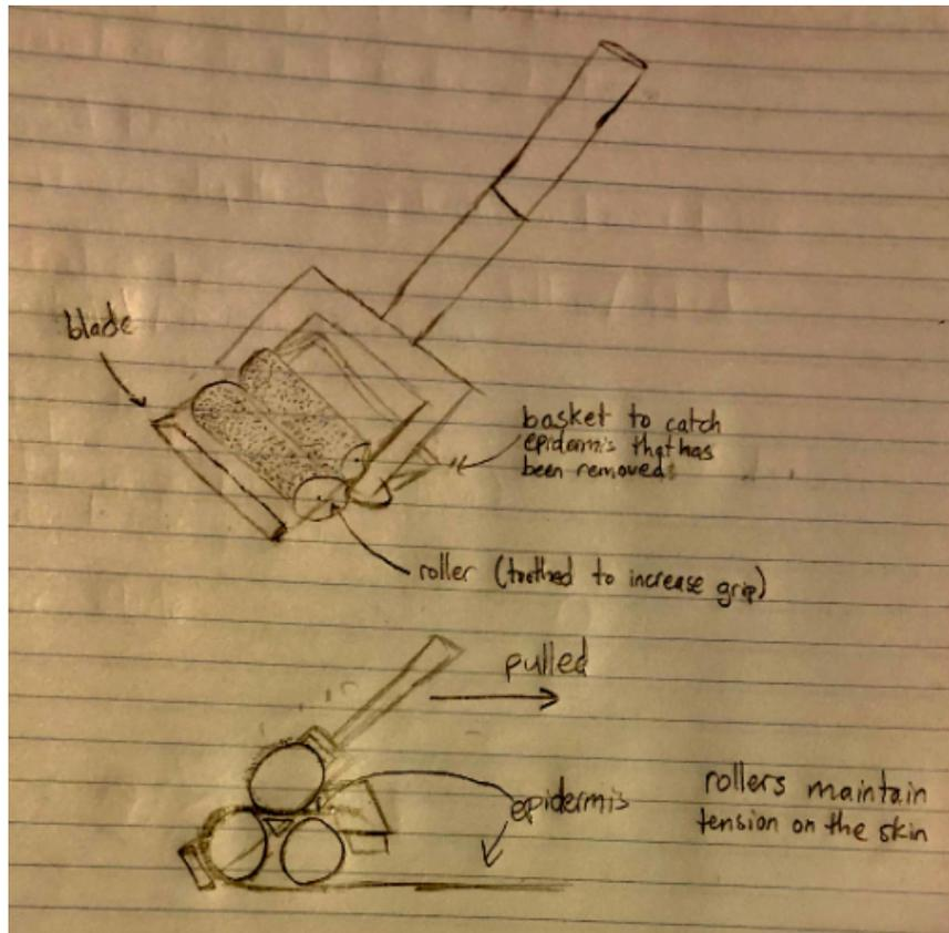
This design consists of three rolling cylinders. As the device is pulled backwards on the surface of the skin, the rollers will pull the epidermis taught as the blade separates the epidermis from the dermis.
