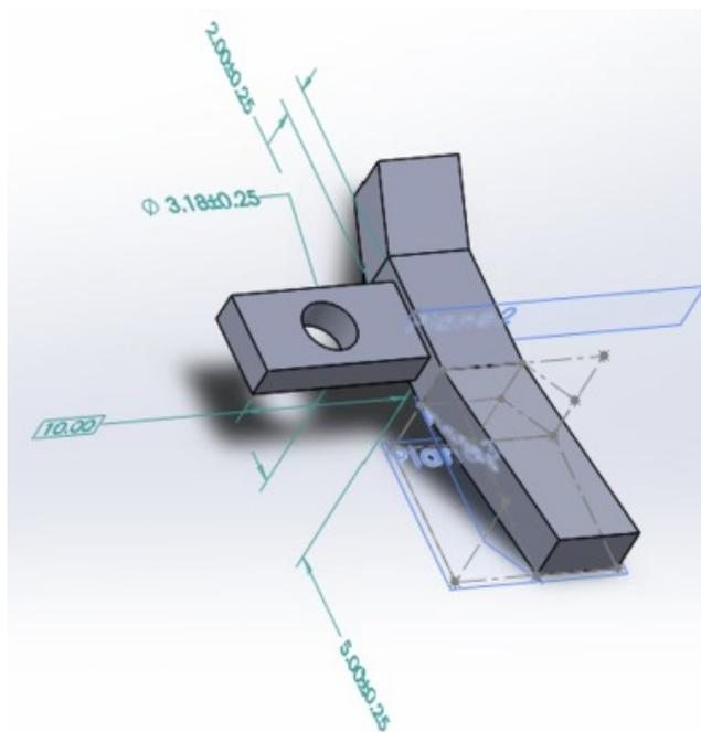
EPPERhinge1.png(82.6 KB) - [download](#) Figure 6: An oblique view of the hinge part of the modified EpiCut showing the dimensions of the part that will slide into the handle part.
