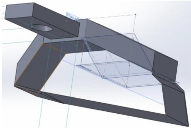
**EPPERhinge2.1.png(136.1 KB) - download** Figure 1: A bottom view of the hinge part with the blades to show how they are oriented and which direction it is facing
