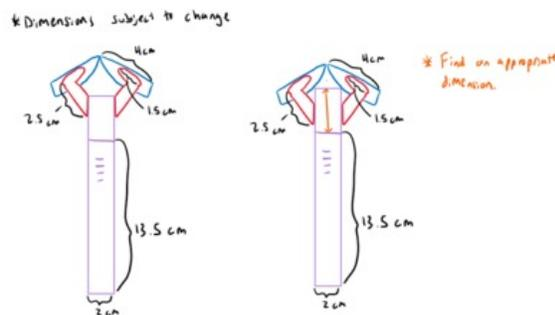
**Design\_revision.png(76.6 KB) - download** Figure 1: Attachment of the arms could be moved backwards to help accommodate the curvature in breast tissue. The length of the bottom surface of the handle should be determined with the same consideration in mind.
