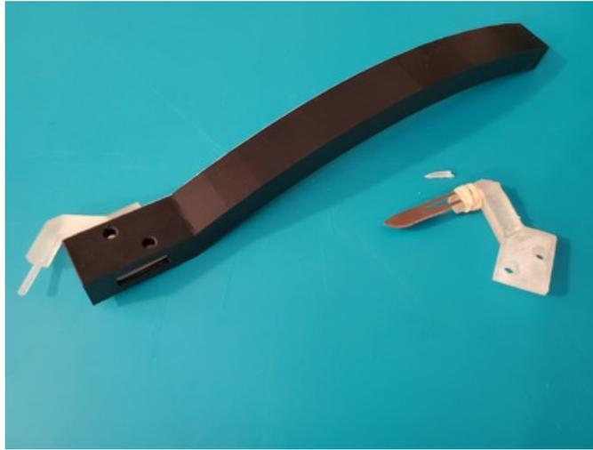
20201202\_122259.jpg(4.1 MB) - [download](#) Figure 2: A 3D printed prototype using Formlabs High Temp resin. Only the right arm is inserted due to an error in printing. The scalpel blade is attached with a rubber band as a result of inaccurate printing.
