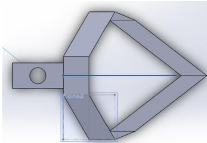
**EPPERhinge2.2.png(151.8 KB) - download** Figure 2: Top view of the hinge part with the blades
