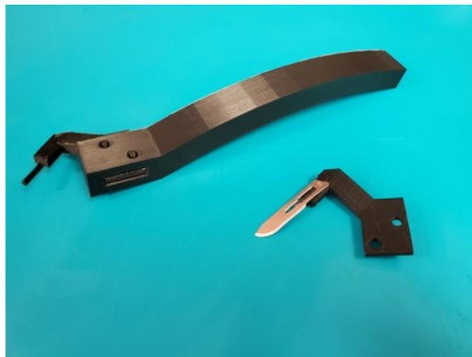
20201202\_123909.jpg(3.8 MB) - [download](#) Figure 1: A 3D printed prototype using Ultimaker Tough PLA. The right arm was the only arm that was able to be inserted due to inaccuracies during printing of the device. The left arm is shown with an attached scalpel blade.
