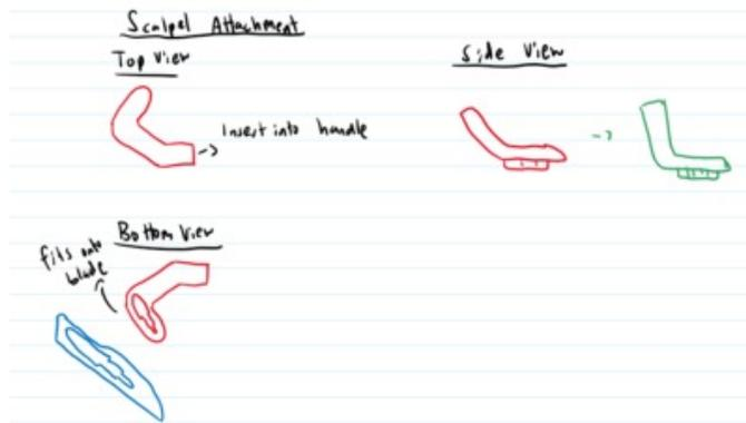
Modified\_scalpel\_attachment.png(57.5 KB) - [download](#) Figure 2: A side arm attachment for #10 scalpels. Different versions of this attachment could be made to allow for different depths of epithelial tissue to be removed.
