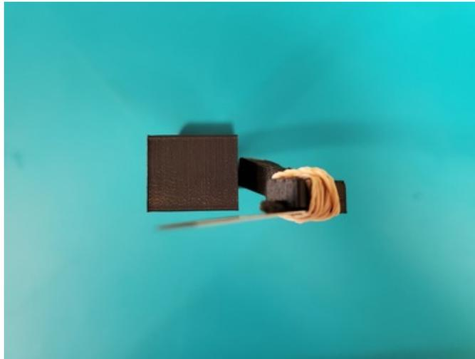
20201202\_125038.jpg(4.4 MB) - [download](#) Figure 3: The tough PLA prototype with one of the arms with the blade attached to it, inserted into the handle. This is a front view with the blade pointing out of the picture. The position of the blade shows that the prototype can be used for testing because the blade is below the bottom of the handle.
