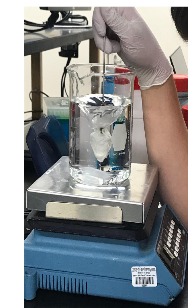
Figure 8.2 Alginate powder being stirred
