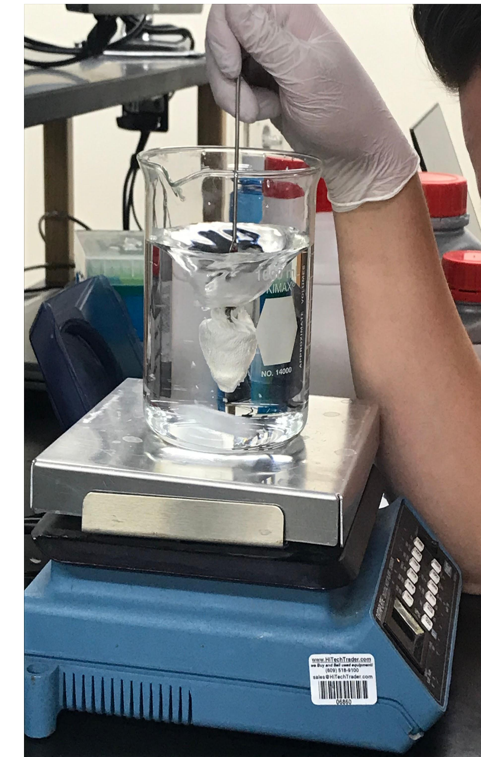
Figure 2.2 Alginate powder being stirred
