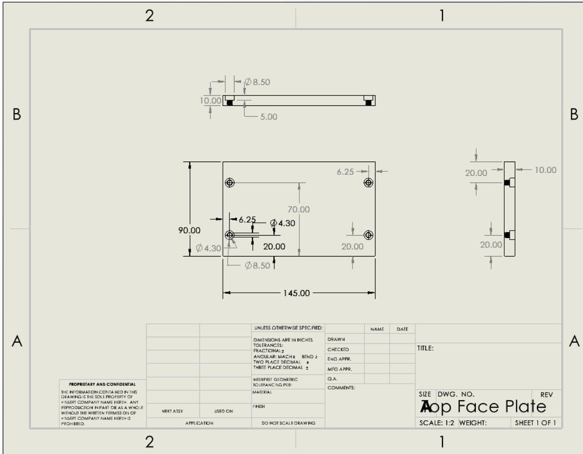
Figure 6: Top face plate drawing
