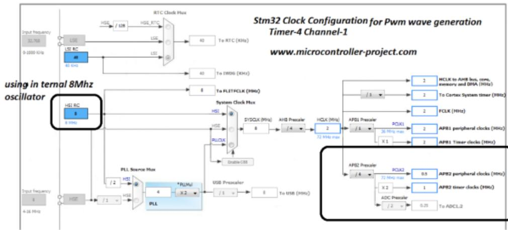
Figure: This figure shows the settings configuration for the stm32 clock for timer 4 channel 1 in stm32cubemx.
