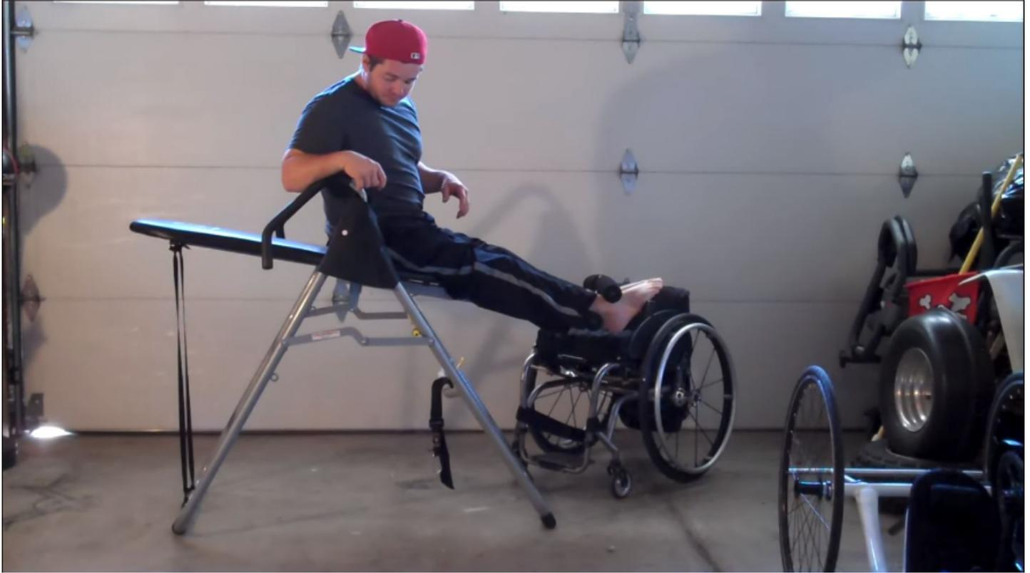
**Figure 3: Adapted inversion table at rest with user secured in the restraints**
