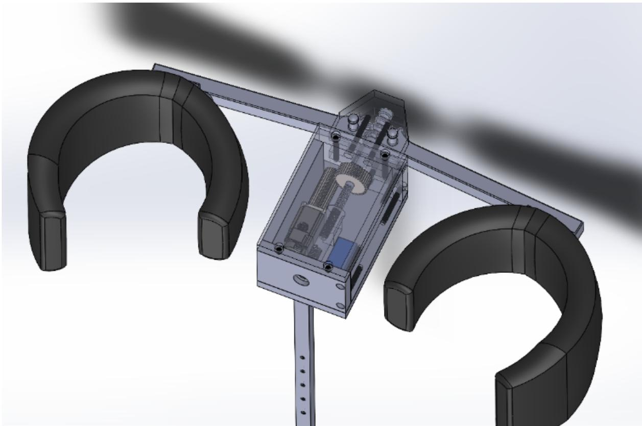
Here is a image of the completed leg support model. There are a number of components that interact with each other for the device to operate correctly. The servo motor drives the gear system, that in turn unthreads or threads the threaded bolt, and the support arms are rotated as a result. The leg support should be able to be far enough out of the way in the retracted position that the client may be able to enter and exit their wheelchair without issue.
