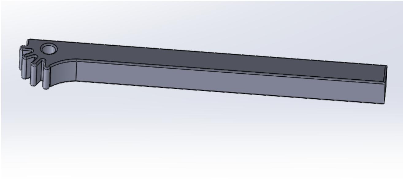
The support arm holds the leg pad itself and is rotated by the threaded bolt. It acts as the pinion in the rack and pinion system.
