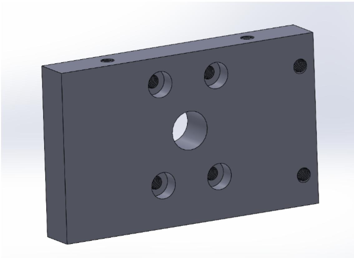
Here is the front face plate, which has a number of threaded holes incorporated into it. The four threaded holes in view that are counterbored are for the front holder plates, the components that secure the support arms to the device.
