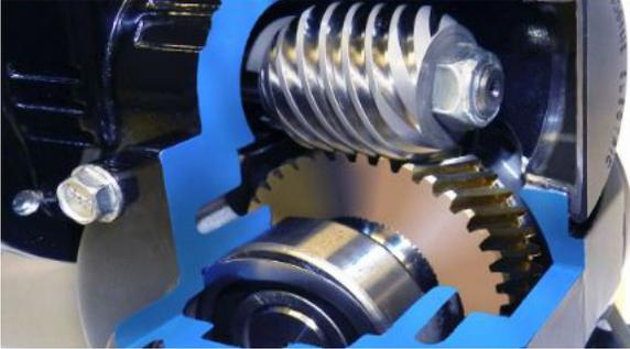
composed of a worm and a worm gear [1]
