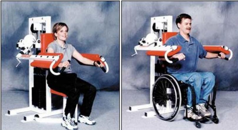
**Figure 1:** Equalizer Exercise Machine in Lateral Deltoid configuration for both a non-disabled user and a wheelchair user
