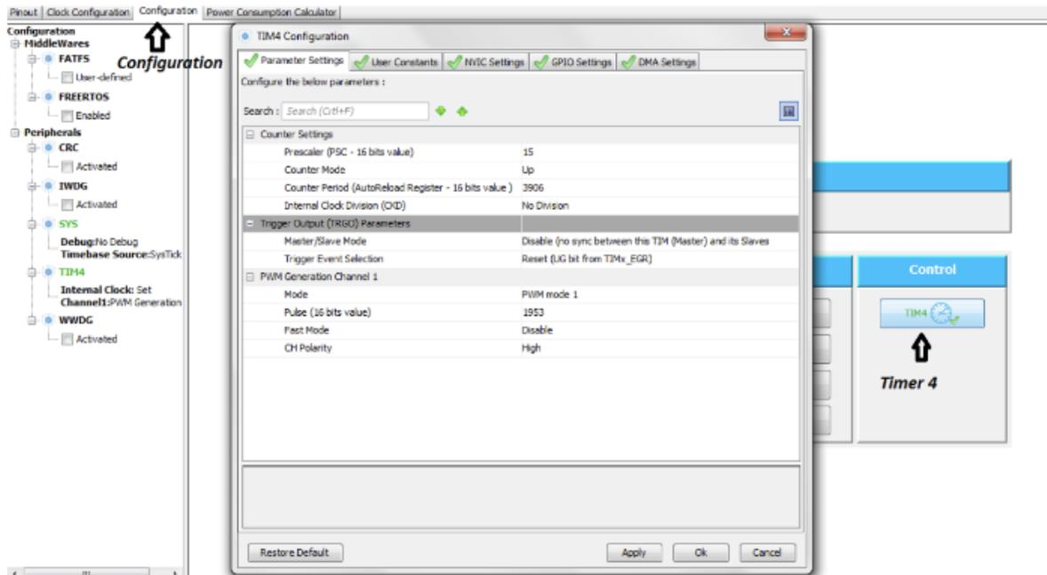
**Figure:** Inputting the calculated values into the timer 4 configuration.
