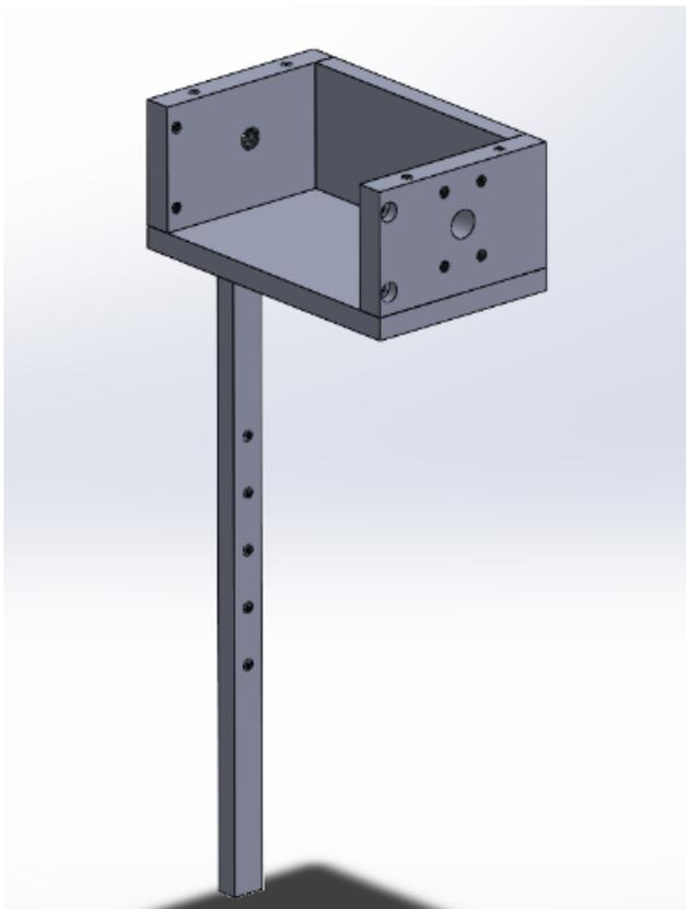
The components welded together look like this, with the top and one side remaining non-permanent attachment points. The detachability of the top and the side are helpful in alleviating the hassle of accessing the device components for maintenance.
