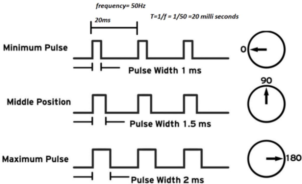
Servo motor pwm duty cycle and frequency requirement
