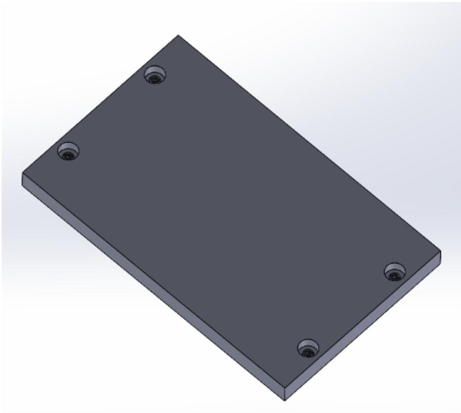
The top plate threads into the front and back plates to secure the plate to the top of the device. The plate can be easily removed to allow for access to the components for maintenance
