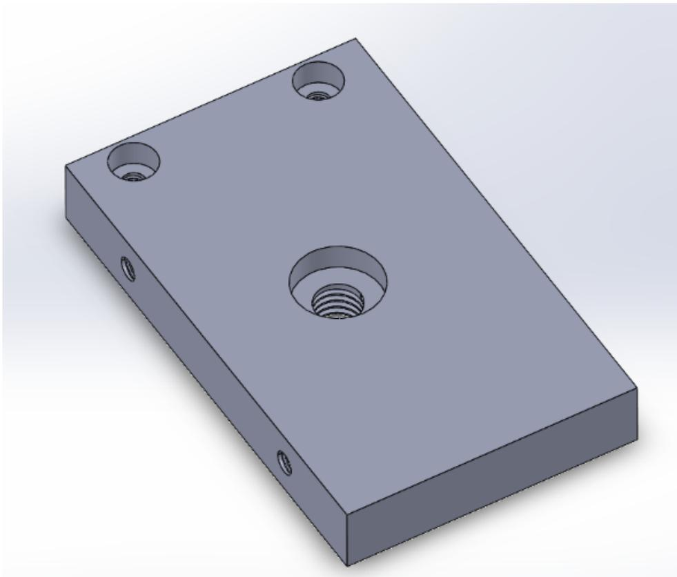
Above is the back face plate which has the large center threaded hole. The hole allows a bolt to be fed through into the back of the threaded support, where it threads in and secures the support.
