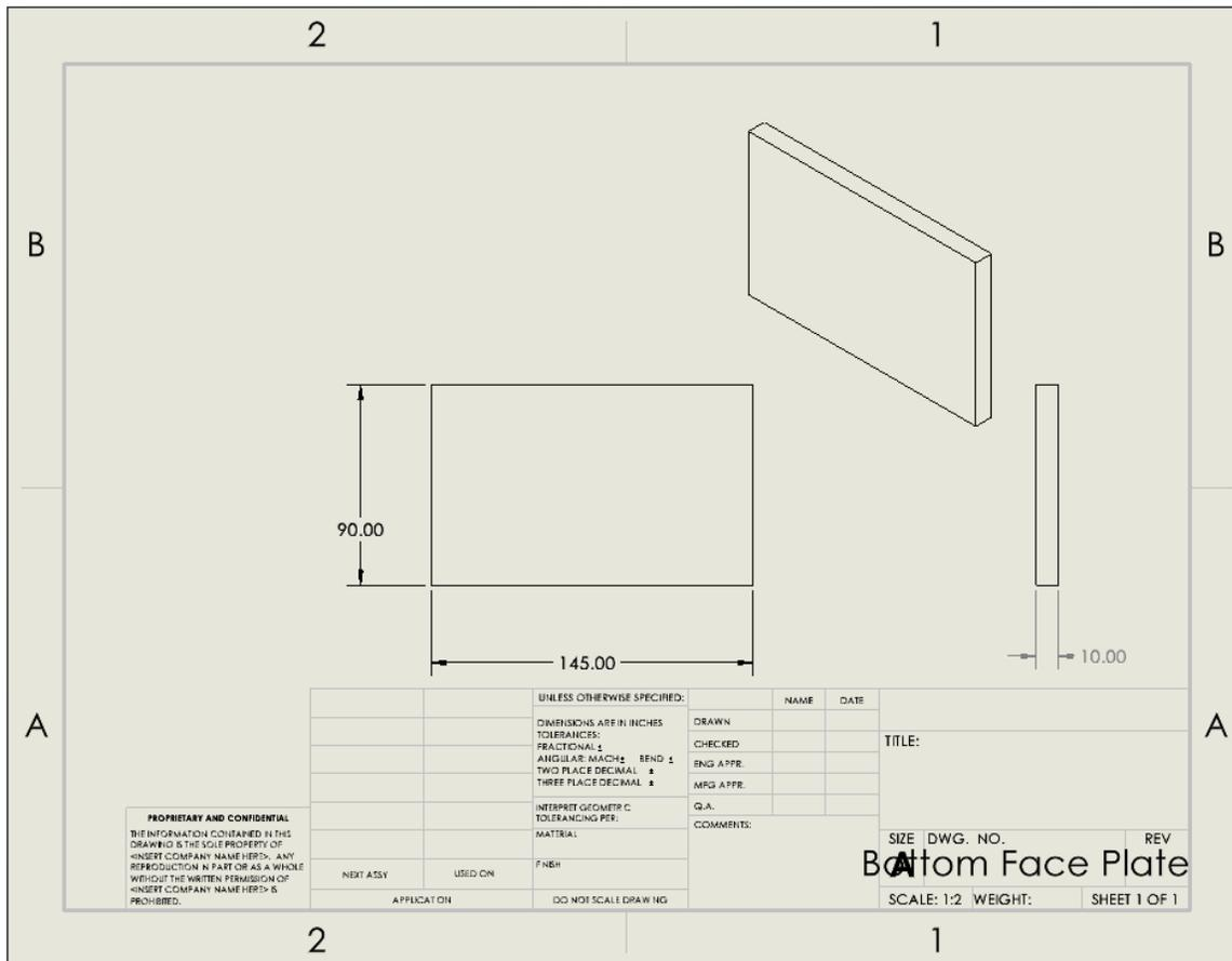
Figure 5: Bottom face plate drawing
