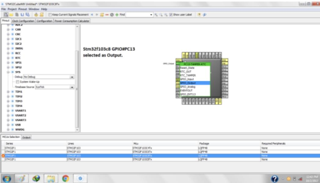
Figure: Next, a window will appear that contains an mcu diagram. Click on pin #13 and set the GPIO as output.
