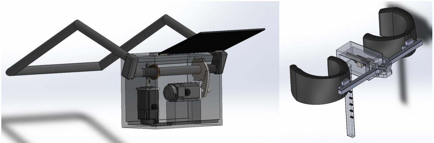
Figure 1: SolidWorks drawing of the chest restraint (left) and leg restraint (right) with their components displayed.
