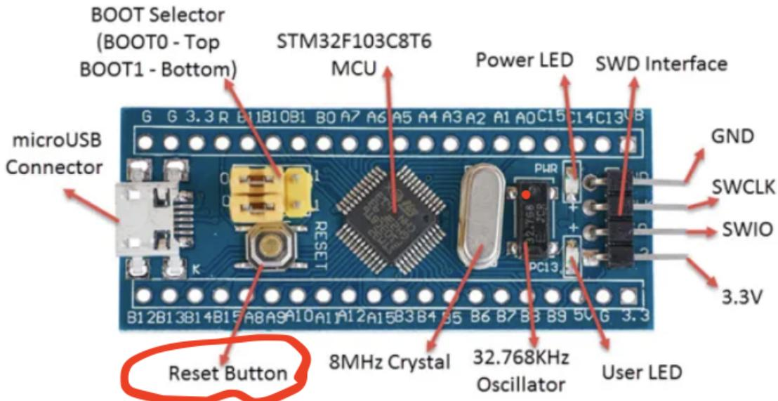
**Figure:** This figure shows where the reset button is located on the Stm-32 microcontroller (and other labeled parts of the board).
