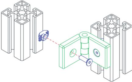
**Figure 10:** Details on how to attach hinge
