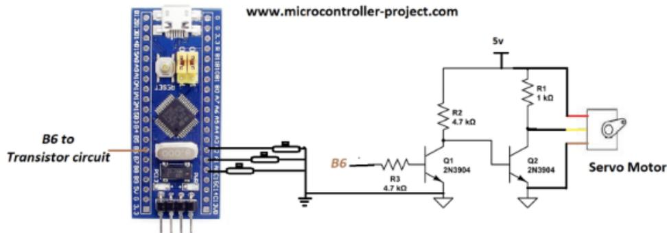
**Figure:** This figure depicts the stm32f103 microcontroller, the pin locations on the microcontroller, and the circuit used to alter the voltage so that it is compatible with the power source of the servo motor. The grounds of both motor and microcontroller should be common.
