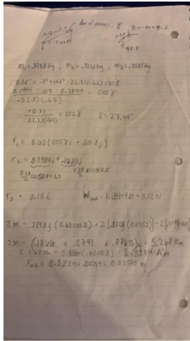
Friction\_and\_torque\_due\_to\_friction\_at\_pin\_leg\_restraint\_.jpeg(2.9 MB) - download
