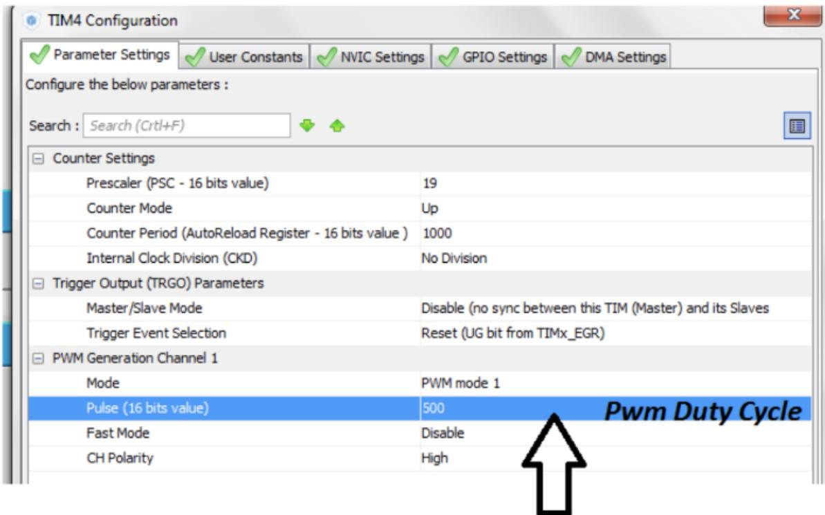
Figure: The timer-4 configuration settings; this shows the setting of pwm counter period and duty cycle
