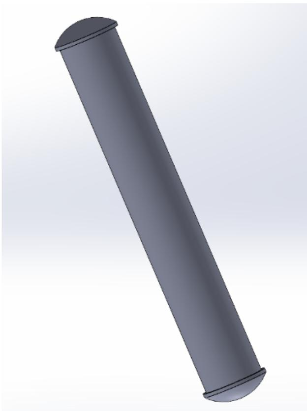
The mounting pin is used to secure the support arm to the leg support box while still allowing rotation to occur.
