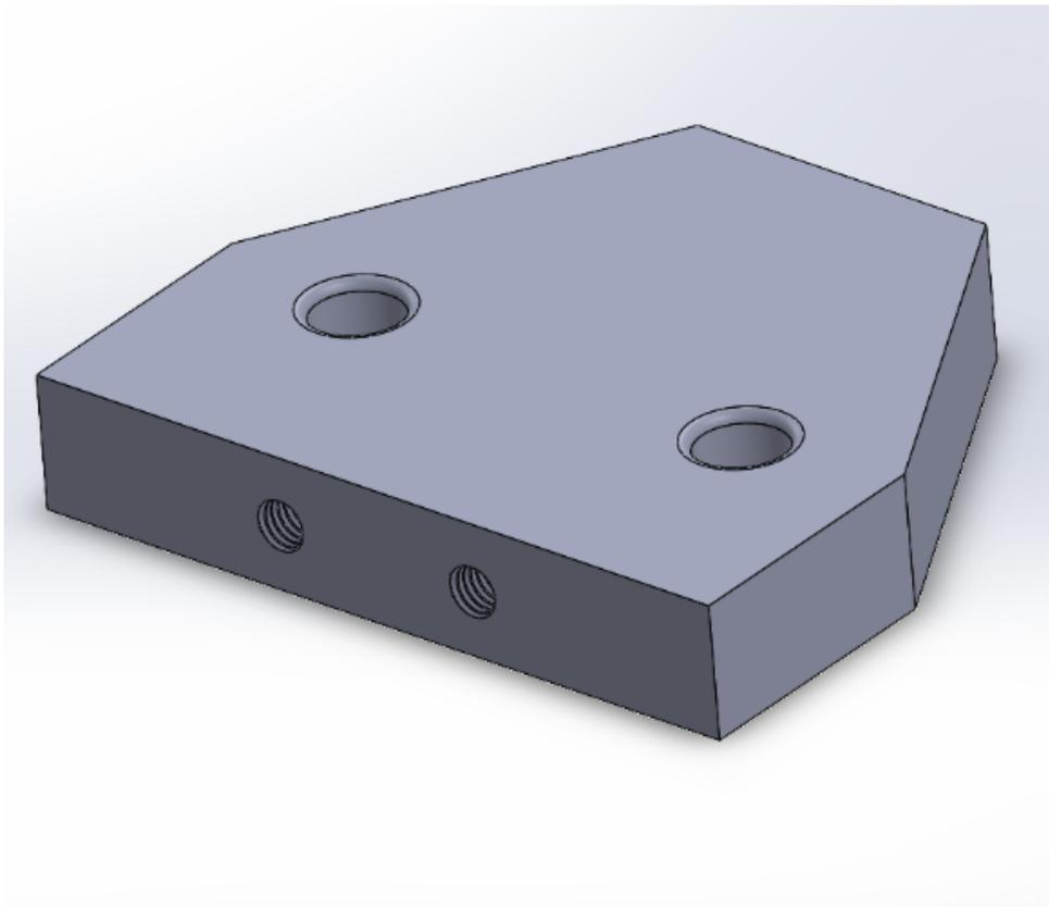
The front holder pieces are mounted to the front of the support through the front plate. The front holder secures the support arms to the device by having nut and bolt pass through the through-hole with the support arm between the two plates.
