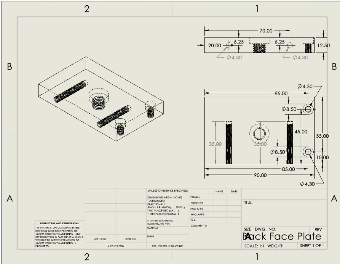
Figure 1: Back face plate drawing
