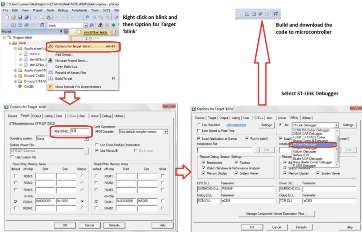
**Figure:** The development board has no on build programmer, so the author used an external stlink programmer to upload the code onto the board. To do this properly, the correct settings in kiel must be used. Follow above steps to upload the code.
