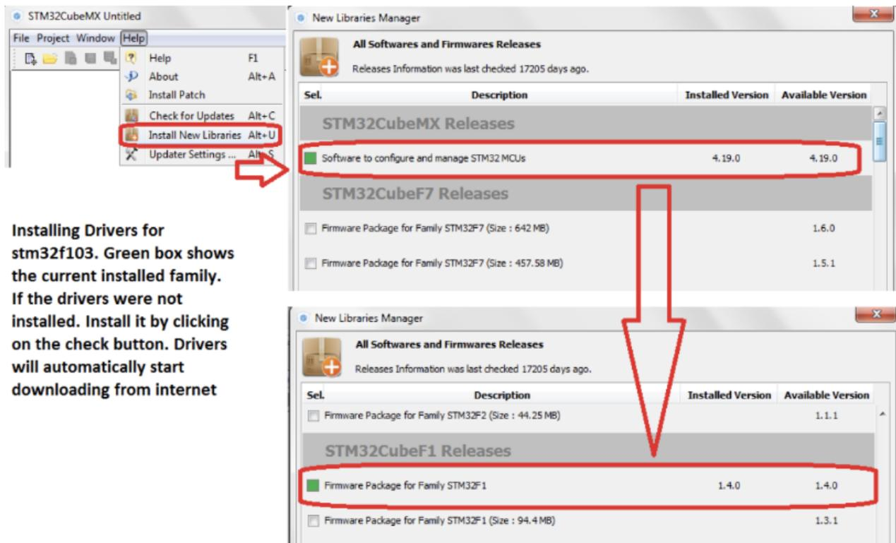
**Installing Drivers for stm32f103. Green box shows the current installed family. If the drivers were not installed. Install it by clicking on the check button. Drivers will automatically start downloading from internet**
