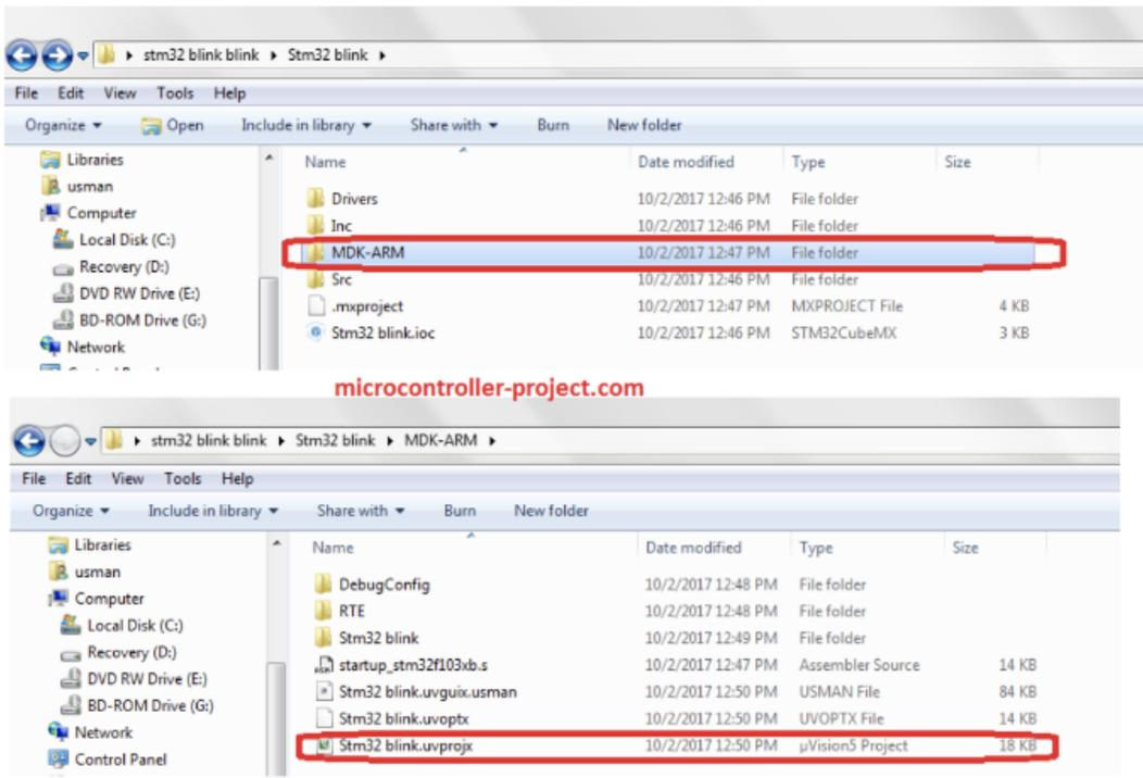
**Figure:** After clicking Ok, the code will be generated at the selected Project location. Four folders will appear in the selected location (top screenshot). The MDK-ARM folder contains the Keil IDE code. The StmCubeMx project file is the .ioc file (stm32cubeMX file). Inside the MDK-ARM folder (bottom screenshot), there is a .uvprojx file that is the Keil IDE file. Now, this file can be opened to make changes to the code.
