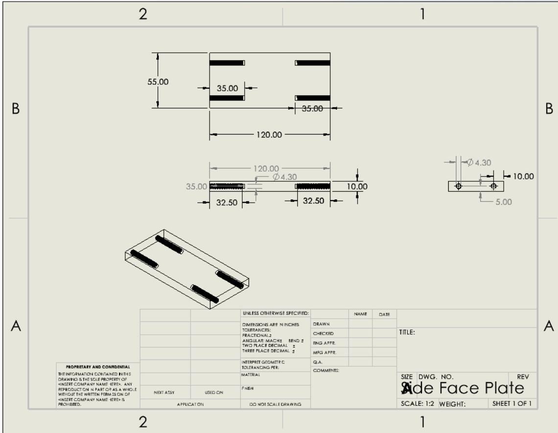
Figure 4: Threaded side plate drawing
