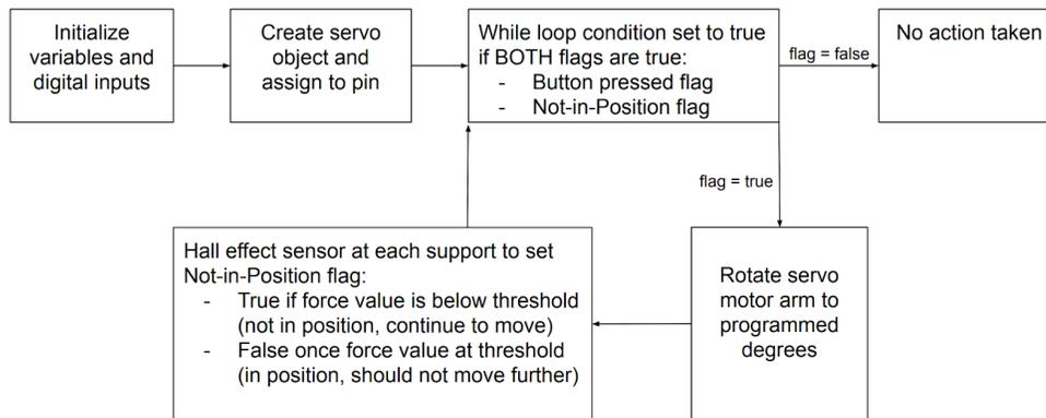
**Figure:** This code flowchart gives an overview of the steps taken in the code.
