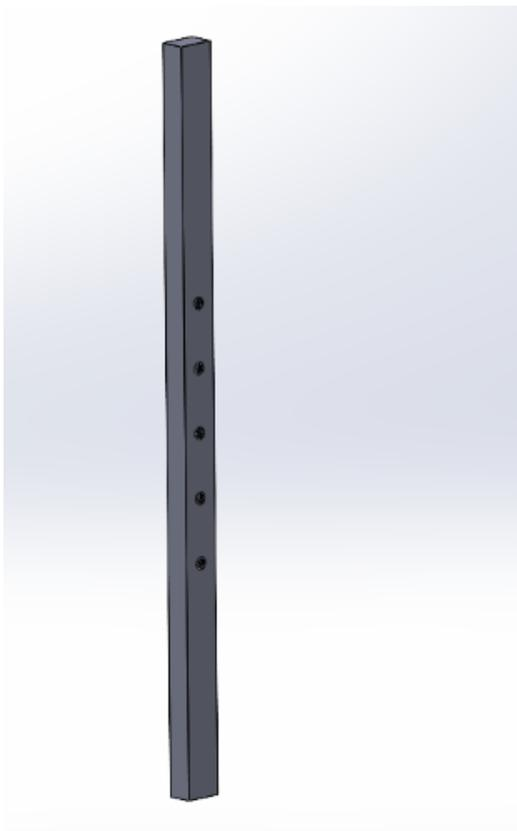
The support bar allows for the height of the leg support to be adjusted while positioned on the wheelchair, and it also allows the support to secure into the mounting place already present on the wheelchair.
