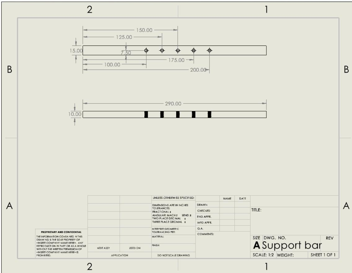
Figure 7: Support rod drawing
