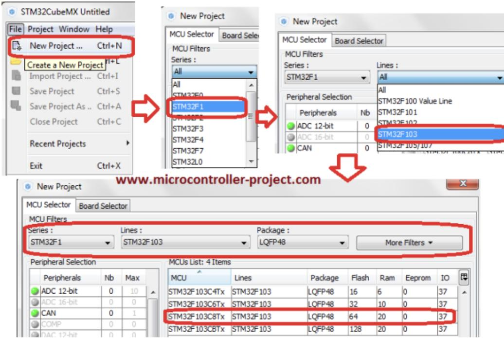
Figure: To create a new project, go to File --> New Project; A window appears that asks you to select microcontroller series, series lines and package. After selecting package, you can click on the microcontroller that is being used for the project. (This case uses STM32f103C8Tx)
