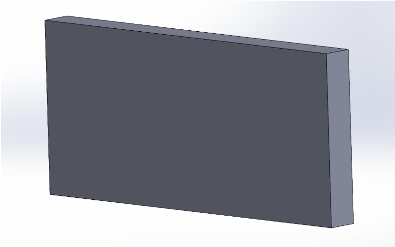
The non threaded side plate does not have any additional holes or modifications to it. It is welded in place on the bottom face plate and is welded to the front and back plate.
