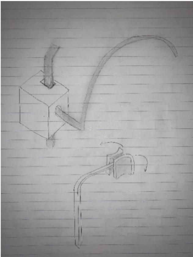
**Figure 1:** Preliminary drawing of the chest restraint (upper left) and leg restraint (lower right)
