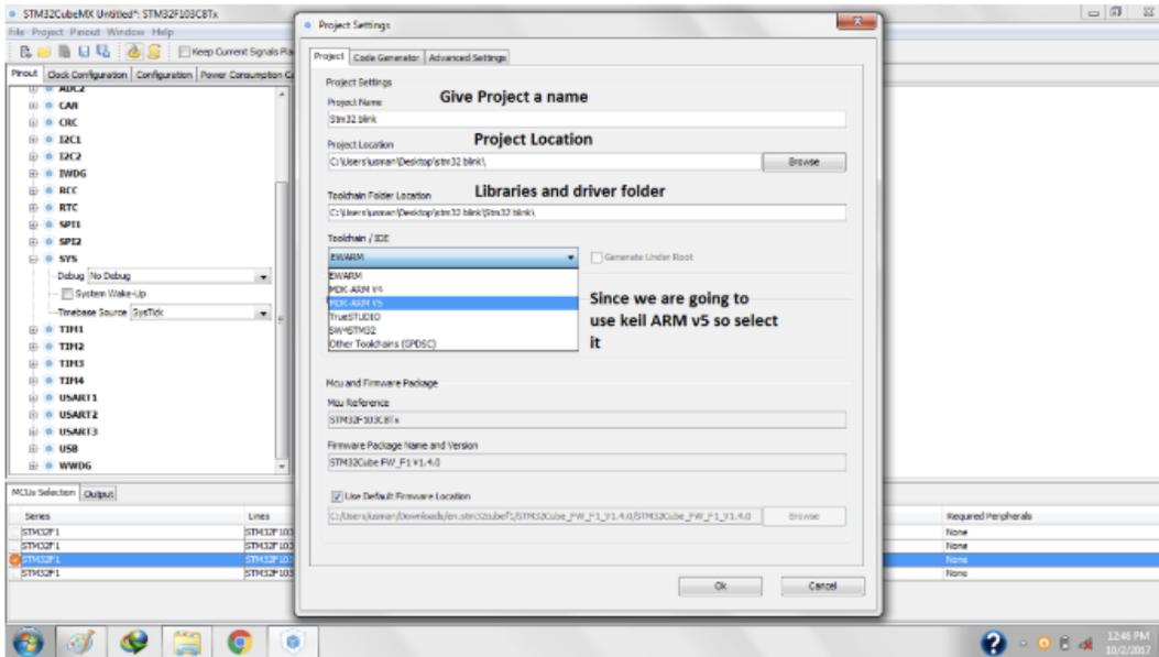
**Figure:** This window appears after clicking gear icon; Now, fill out the Project name and select Project location. This example uses MDK-Arm V5, so select MDK-ARM V5 under the Toolchain/IDE drop down. Click Ok to generate code.
