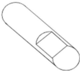
**Figure 3:** Mill flat onto shaft
