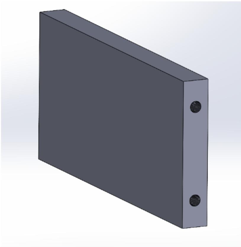
The side plate is threaded into the front and back plates, similar to the top plate, to allow the device to be disassembled. Having the side piece as well as the top piece removable, allow the components located inside to be easily removable and replacable if needed.
