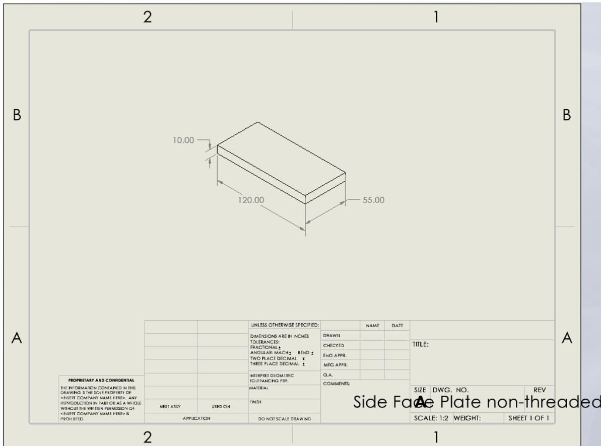
Figure 3: Non-threaded side plate drawing
