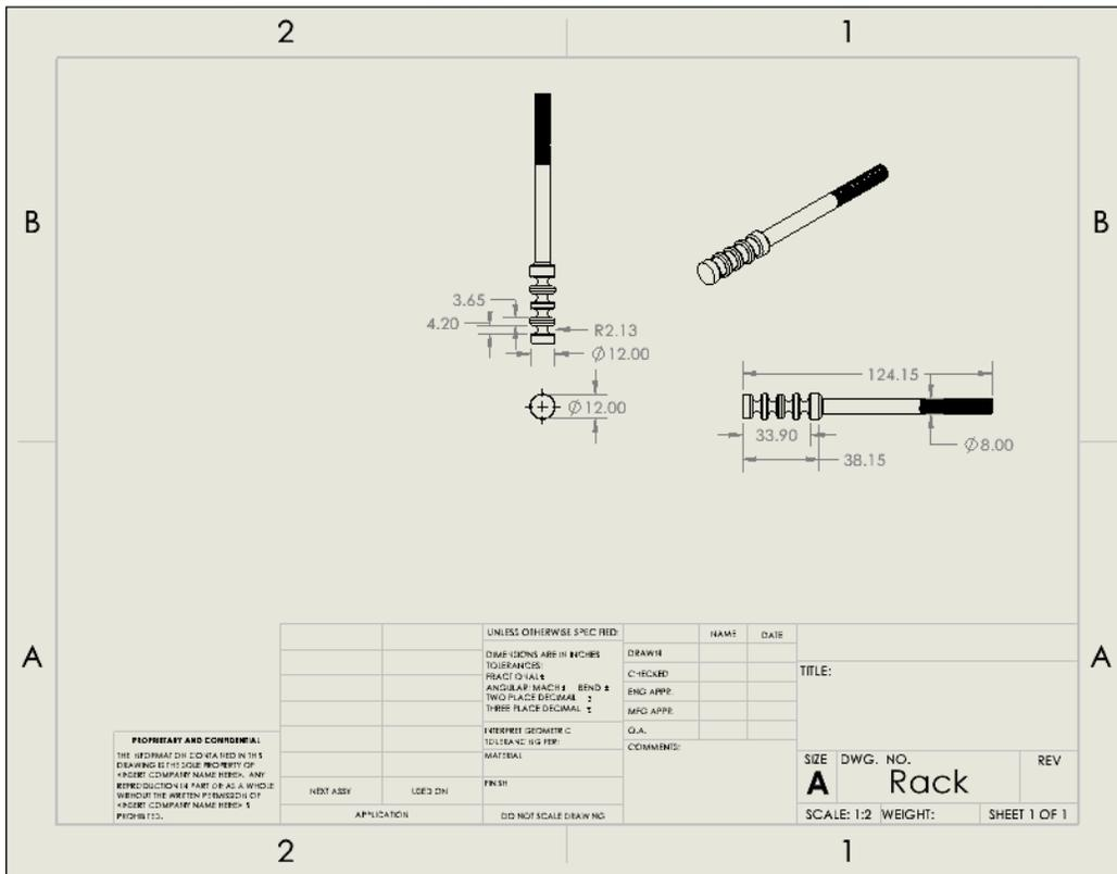
Figure 8: Threaded Bolt drawing
