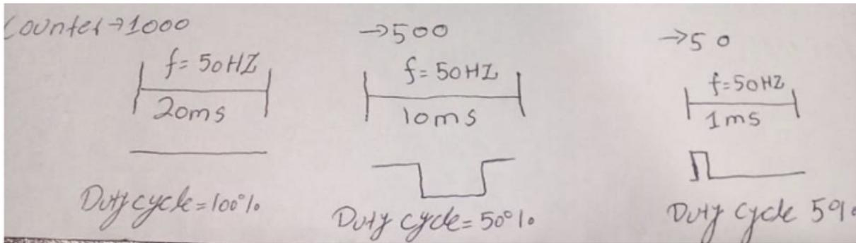
**Figure:** The relationship between counter period, frequency, time, and duty cycle.
