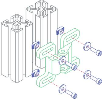
**Figure 11:** Details on how to attach catch and latch
