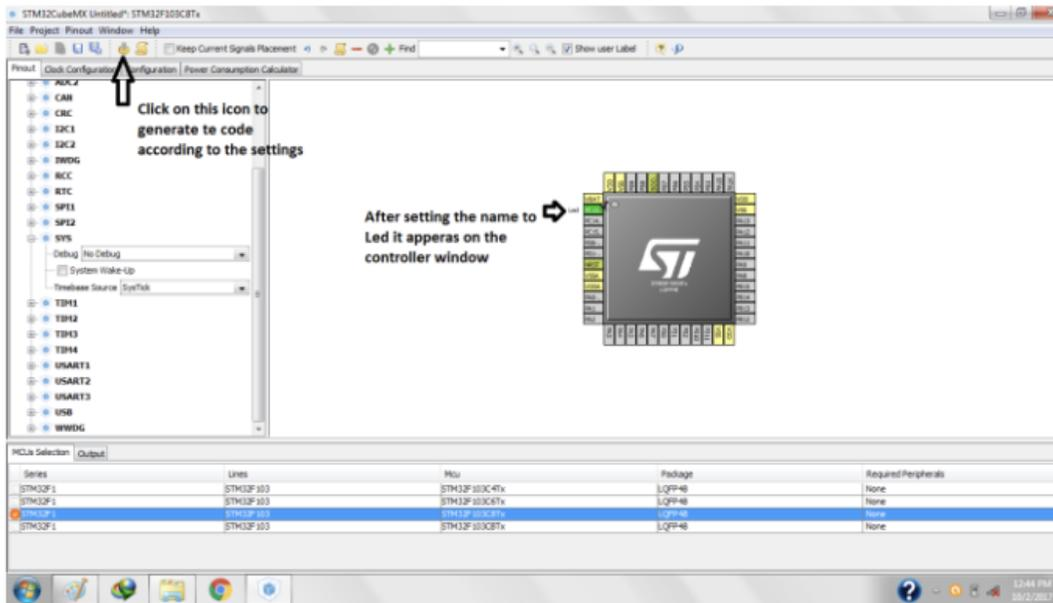
**Figure:** The name that we set now appears on the pin that was changed. We can use the gpio in code with this name. Next, click on the gear icon to generate code.
