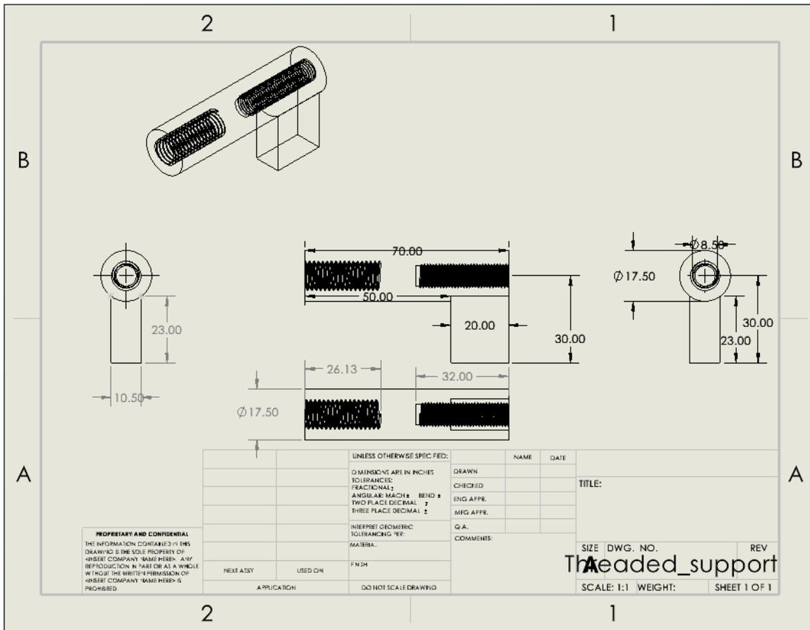
Figure 10: Threaded support drawing
