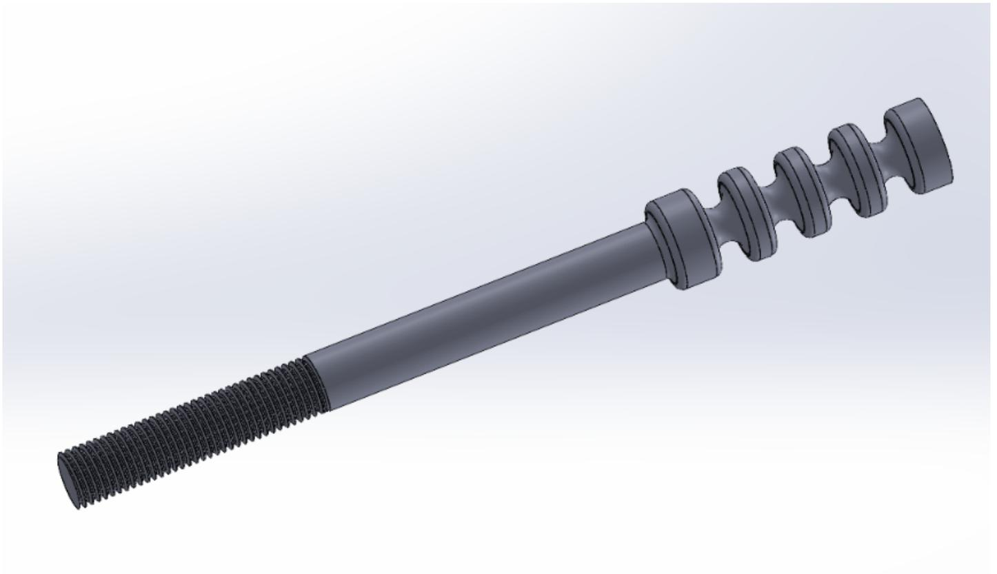
The threaded bolt is responsible for moving the support arms by threading or unthreading into the box's support. The grooves on the upper region of the threaded bolt function as the rack for the rack and pinion system.
