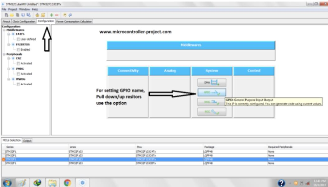
Figure: To configure the GPIO, click the configuration tab and then GPIO button.
