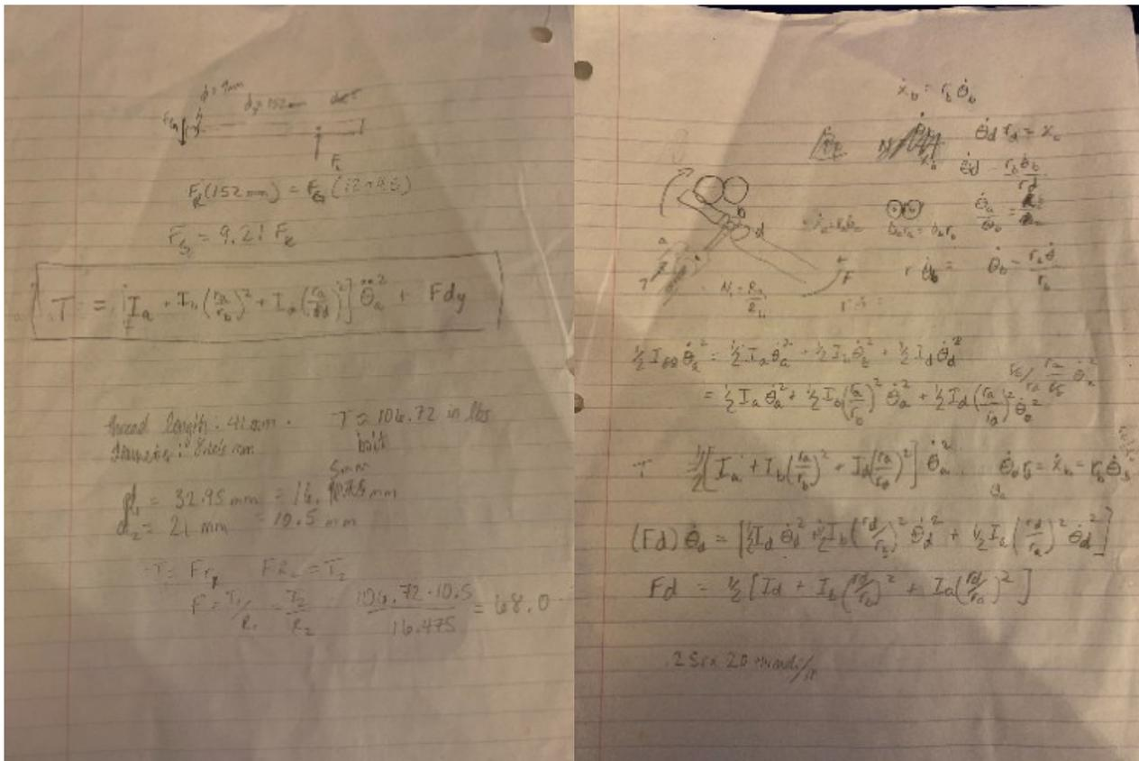
Friction and torque due to friction at leg restraint pin calculations
