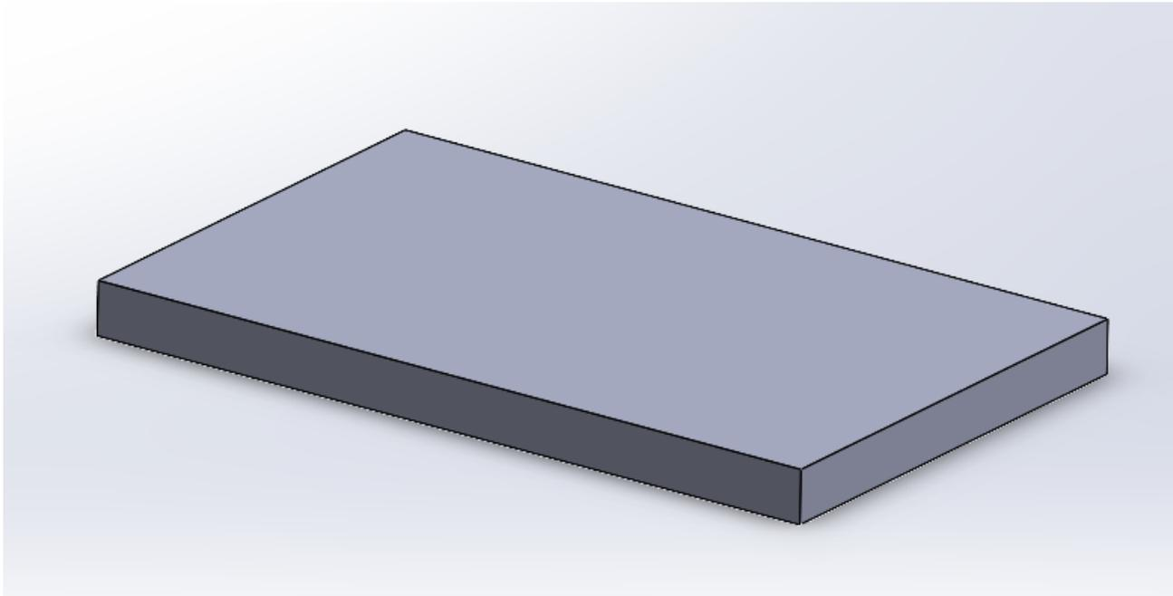
The bottom face plate is the base of the leg support box and a number of components are welded to it for ease of fabrication. The front, back, and one side plate, along with the support rod are all welded onto the base plate as seen in the solidworks model below of the welded components.
