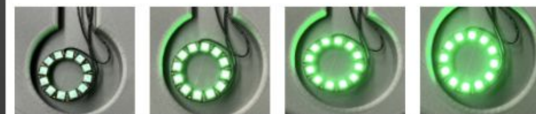
Figure 6: Depiction of the ring LED to represent increased oxygen by increasing brightness
