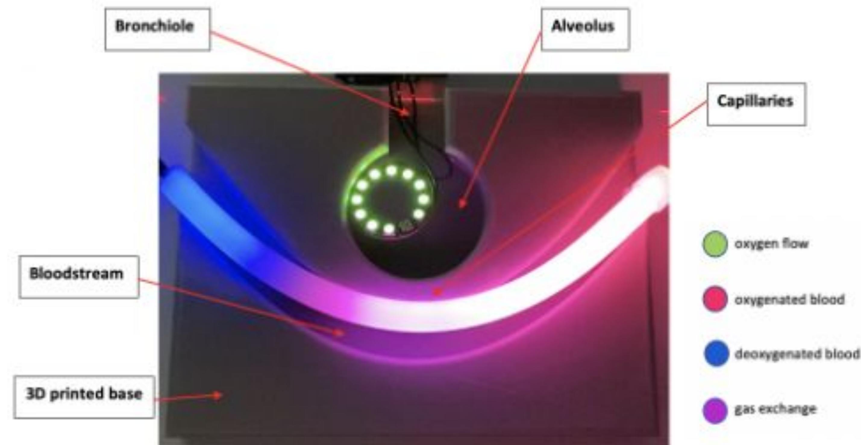
Figure 5: The 3D printed base including a single alveolus and the bloodstream with LEDs to represent V/Q ratios.
