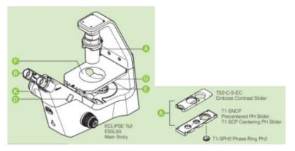
Above part A, we will add threads or an extension to change the vertical height of the condenser in reference to the middle plate, F
