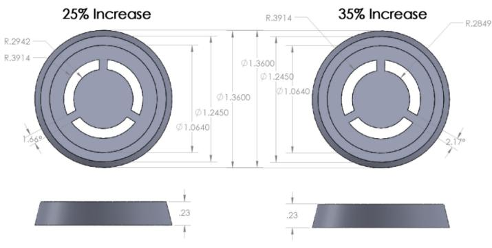
The printed parts were measured for tolerance on the following critical dimensions: Inside Ring Radius (0.294 in and 0.285 in), Outside Ring Radius (0.391 in), Outside Diameter (1.36 in), and Part Thickness (0.23 in). These dimensions were compared to the printed parts and were within the preset 5% tolerance.
