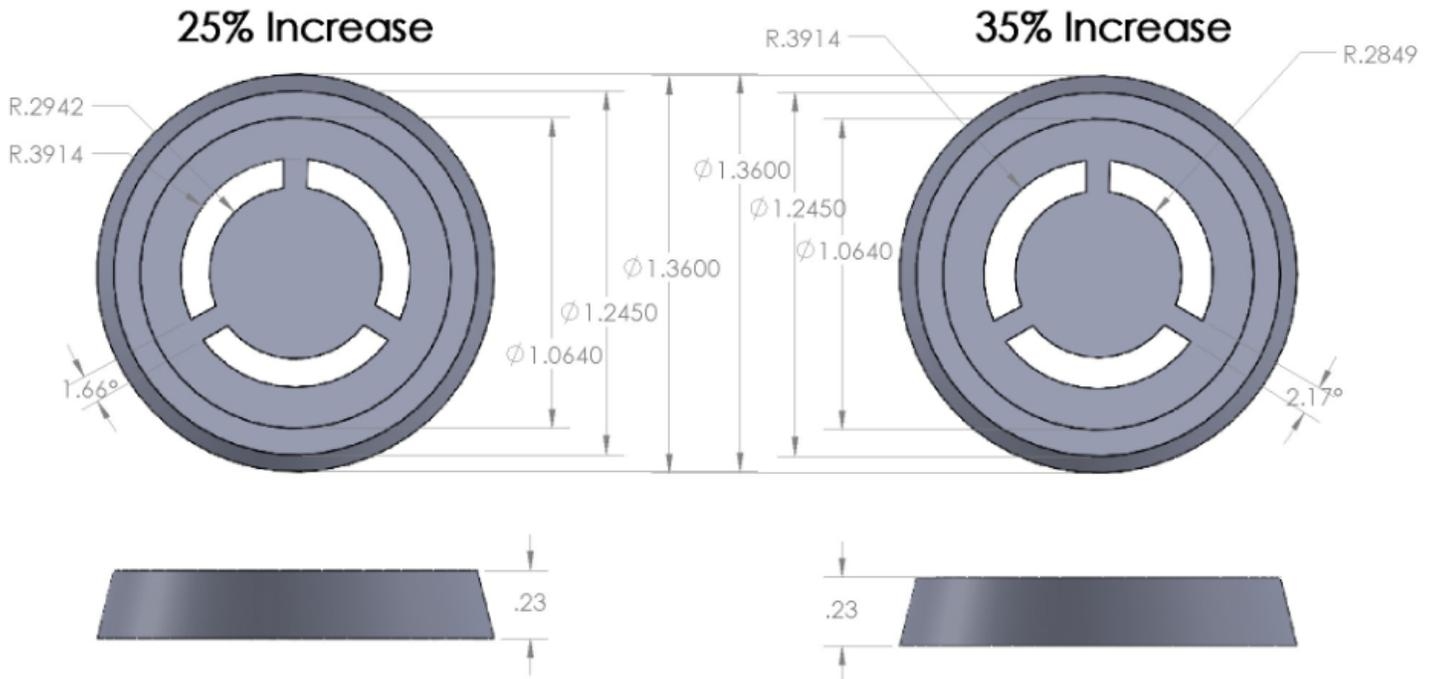
The printed parts were measured for tolerance on the following critical dimensions: Inside Ring Radius (0.294 in and 0.285 in), Outside Ring Radius (0.391 in), Outside Diameter (1.36 in), and Part Thickness (0.23 in). These dimensions were compared to the printed parts and were within the preset 5% tolerance.
