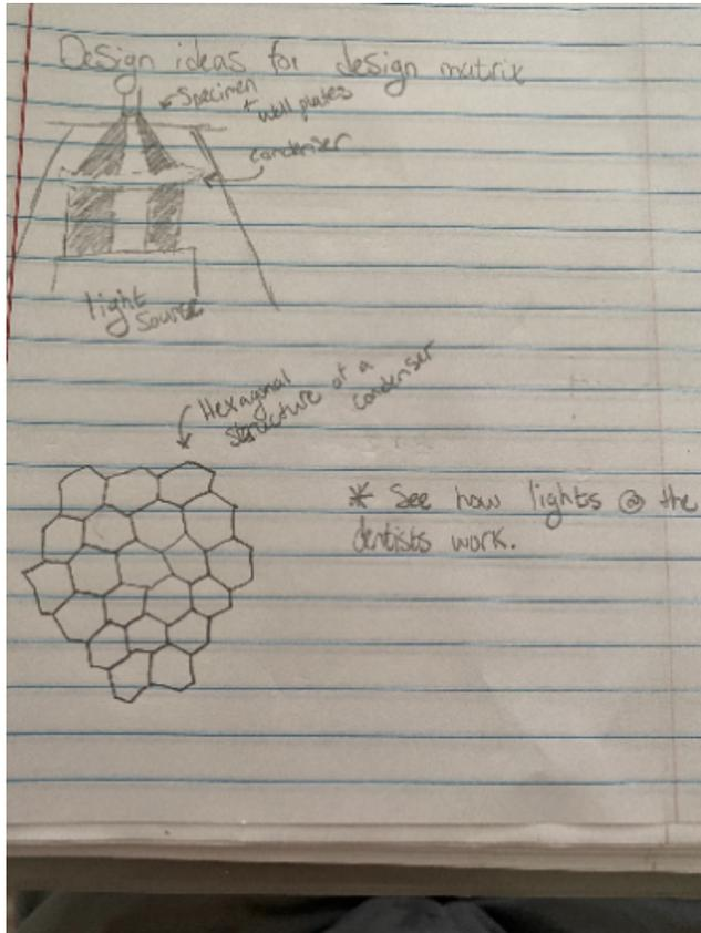
In the top image, I have a slightly thinner condenser than one seen on the microscopes currently. In the bottom image, I have a hexagonal structure that might be better at illuminating the specimen. The light source is supposed to concentrate the light cone better to a more confined area. This will solve the solution to our hypothesis: the light is being clipped by the edge of the well plate.
