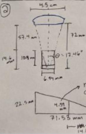
We need an in-between lens to narrow the NA before the top of the well plate.
