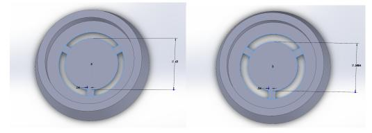
Following the design of the 25% increased annulus, the identical mathematical process was done to create an annulus with a 35% increased area as well. The engineering drawings for both of these parts can be seen below:
