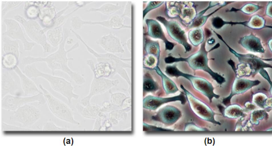
Above is an example of transparent cells in a light-field microscope (a) compared to a phase contrast microscope (b).
