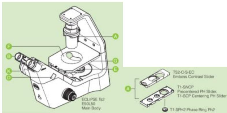
Above part A, we will add threads or an extension to change the vertical height of the condenser in reference to the middle plate, F
