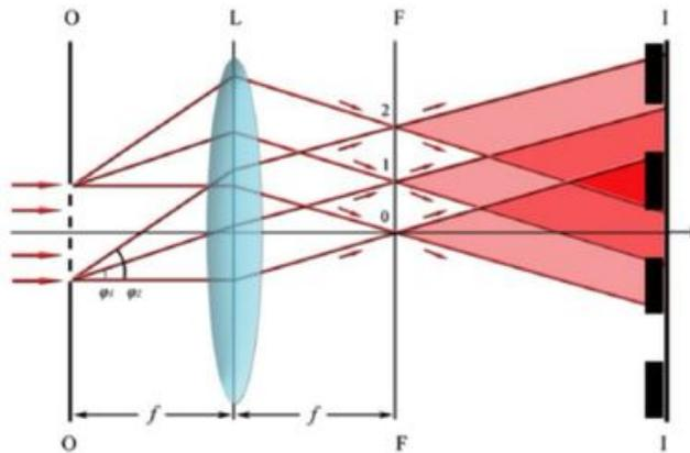
BME\_300.JPG(33.5 KB) - [download](#) Optics and lenses. O=Object L=Objective F=Focal Plane I=Image Plane f=focal distance of objective
