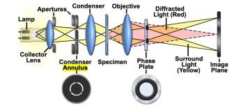
• This figure shows how the annulus is oriented in a phase-contrast microscope.
