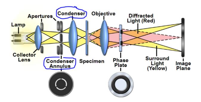
Above is the optical train of a phase contrast microscope. The condenser and condenser annulus are located directly below the specimen and server the function of redirecting the light into the specimen to be phase-shifted.
