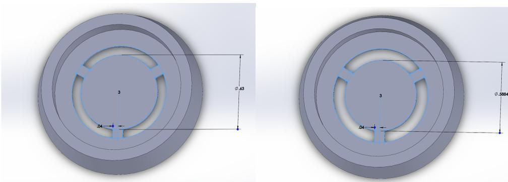
Following the design of the 25% increased annulus, the identical mathematical process was done to create an annulus with a 35% increased area as well. The engineering drawings for both of these parts can be seen below:
