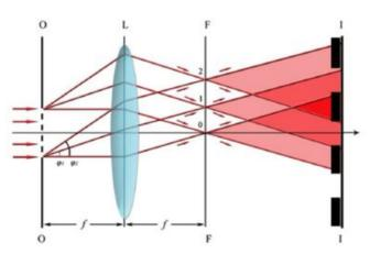
BME\_300.JPG(33.5 KB) - download Optics and lenses. O=Object L=Objective F=Focal Plane I-Image Plane f=focal distance of objective
