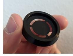
In order to replicate then subsequently modify the annulus in CAD, we took measurements of the current annulus using a digital caliper. These measurements can be seen in the image below, which also contains the calculations done to modify the inner diameter of the "negative space ring" to allow 25% more light through.
