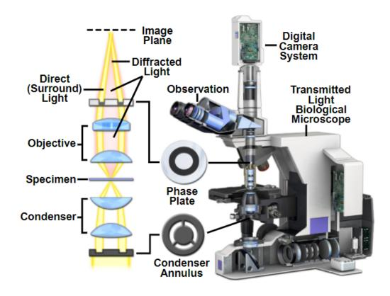
Shown above is a typical phase contrast microscope, with the different components shown. The part of the microscope that we will be working with is the condenser. We want to modify that part to allow the viewing of multiple specimens at once.
