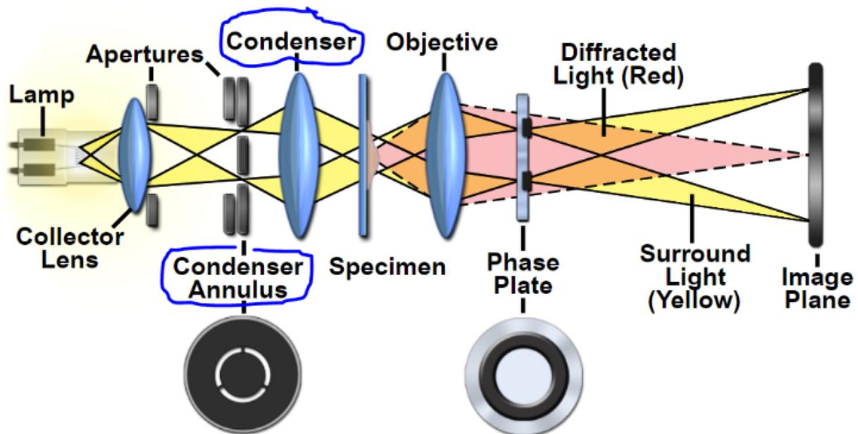
Above is the optical train of a phase contrast microscope. The condenser and condenser annulus are located directly below the specimen and serve the function of redirecting the light into the specimen to be phase-shifted.
