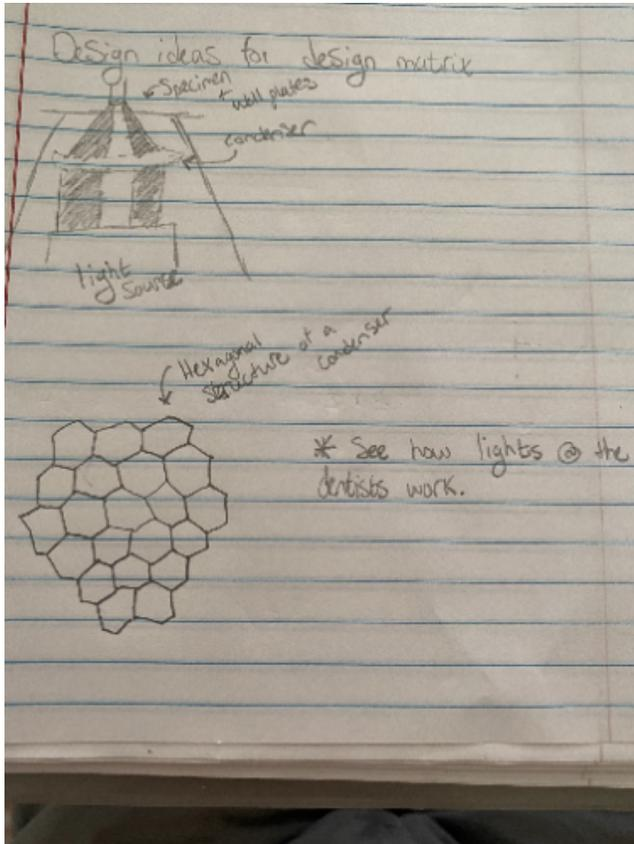
In the top image, I have a slightly thinner condenser than one seen on the microscopes currently. In the bottom image, I have a hexagonal structure that might be better at illuminating the specimen. When I had my wisdom teeth removed, the light source had this background structure and seemed to concentrate on my mouth nicely and did not bother my eyes when I looked at it.
