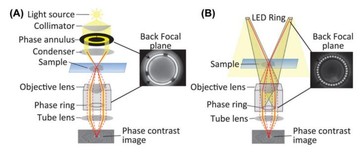
• Shows the difference between the Zernike phase contrast and the condenser free phase contrast (Above)
