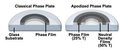
This figure shows a neutral density film placed along the phase film to reduce the intensity of the light diffracted
