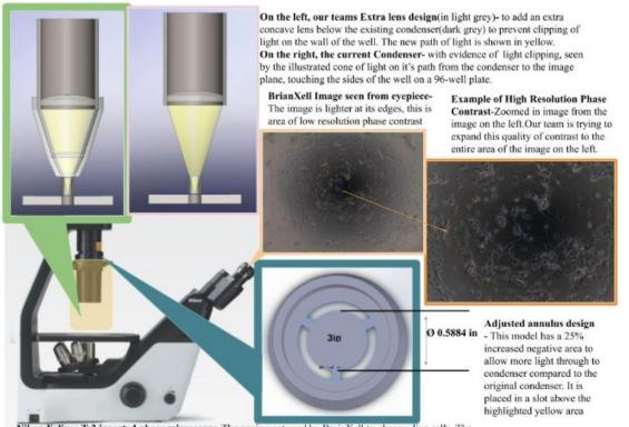
Nikon Eclipse Ts2 inverted phase microscope. The equipment used by BrainXell to observe live cells. The highlighted yellow area is the removable and deconstructable condenser which our team is focused on redesigning
