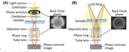
• Allows for the object's back focal plane to light up the image (b)
