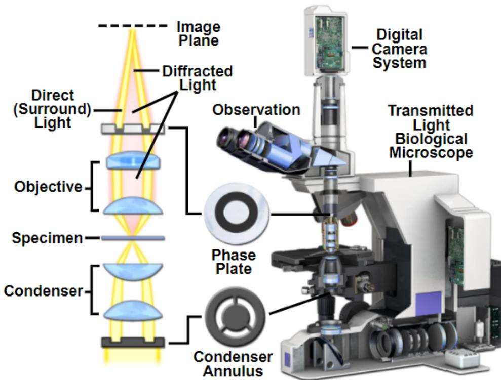
Shown above is a typical phase contrast microscope, with the different components shown. The part of the microscope that we will be working with is the condenser. We want to modify that part to allow the viewing of multiple specimens at once.
