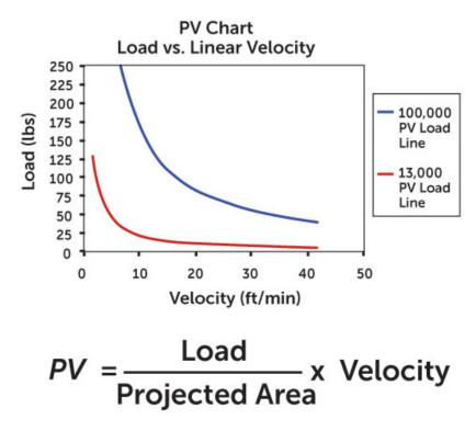
Figure 1. An image relating pressure and velocity to highlight the pressure velocity factor.
