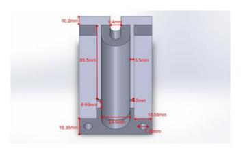
Syringe\_Housing\_Drawing.jpg(32.4 KB) - download The picture above is the front half of our structural design with dimensions.
