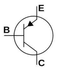
Figure 1.2 An image of a typical PNP Transistor.
