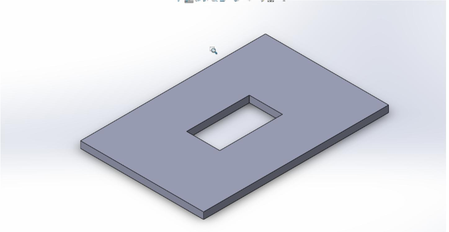
**Shown Above:** Top Cover for the remote control, will be glued on top of the **Bottom Piece** (Shown below)
