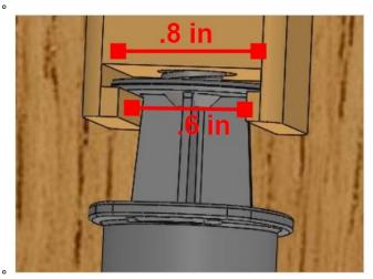
The above images showcase a top and side view of the Lead Screw Plunge Design as well as a closeup view of the interface between the plunger of the syringe and t cap. The leadscrew is fed through the holding cap so it is still able to interface with the plunger to depress it upon controller activation.
