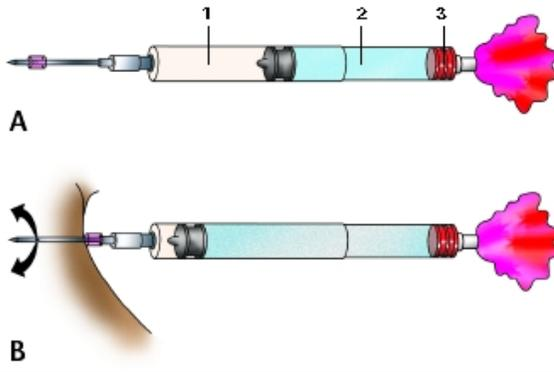
▲ Air-pressurized blow dart in flight (A) and following skin penetration (B). Note the different components: (1) drug chamber, (2) pressurization chamber, and (3) one-way valve.
