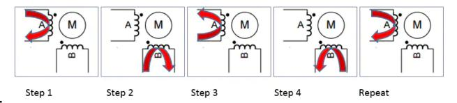
Figure 1. This figures summarizes how a Bipolar Motor functions. It will initially align the magnet with the first coil. It will next rotate the magnet 90 degrees. Opposite coils are connected, but generate opposing magnetic fields relative to the central magnet.
