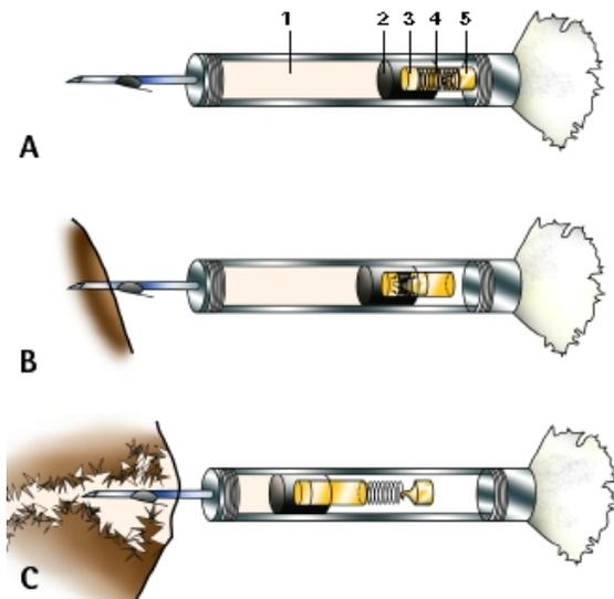
▲ Dart with a powder charge injection system. Note the components: (1) Drug chamber; (2) plunger; (3) explosive charge; (4) spring; (5) firing pin. (A) Dart in flight. (B) Dart impacting skin with firing pin compressing the spring and detonating the charge. (C) Dart during the last stage of injection. Note the tissue damage that is possible with this type of dart system.
