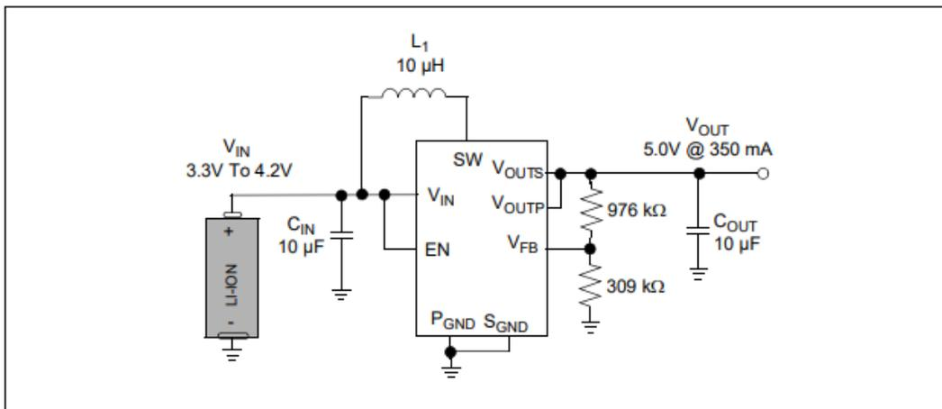
**FIGURE 6-2:** USB On-The-Go Powered by Li-Ion.
