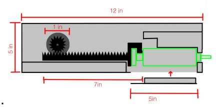
Figure 1: A side view of the Rack and Pinion design with dimensions labeled in inches
