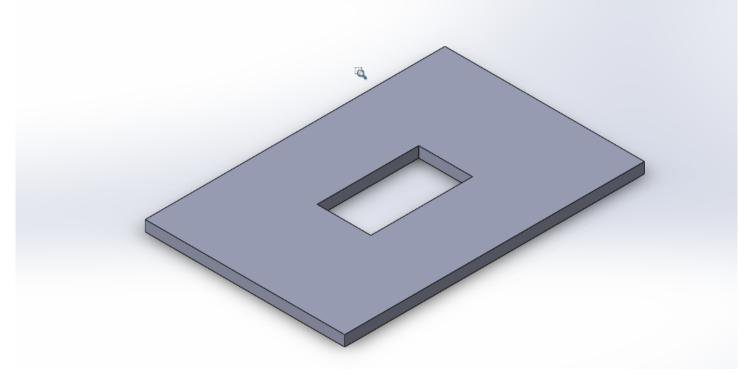
Shown Above: Top Cover for the remote control, will be glued on top of the Bottom Piece (Shown below)
