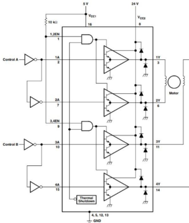
Figure 3. Two-Phase Motor Driver (L293D)
