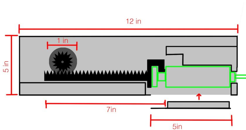
This design is beneficial because it has only 2 moving parts, as well as having the lowest power draw of the three designs, but it is plastic and therefore may not hold up under pressure or continuous use.
