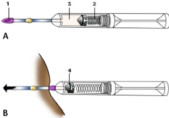
▲ Spring-pressurized dart. (A) The dart is ready for firing, with (1) a tight-fitting cap occluding the dart's needle while (2) the coiled spring pressurizes (3) the agent. (B) Dart in the final stage of injection. The needle's cap slides backward as the needle penetrates the skin, allowing the spring to push (4) the plunger forward, injecting the agent.
