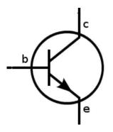
Figure 1.1 An image of a typical NPN Transistor.
