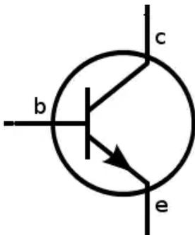
**Figure 1.1** An image of a typical NPN Transistor.
