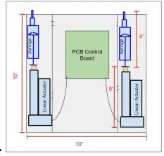
Figure 2: A top view of the Linear Actuator design with dimensions labeled in inches
