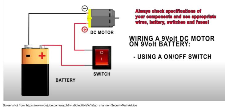
This video is very important as it shows the way to wire in a switch in a way so the switch controls the flow of power from the power source by acting as a toggle in the circuit. This can aid us as it will help us to draw circuit diagrams for our device.
