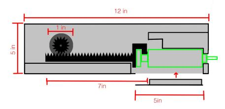
This design is beneficial because it has only 2 moving parts, as well as having the lowest power draw of the three designs, but it is plastic and therefore may not hold up under pressure or continuous use.
