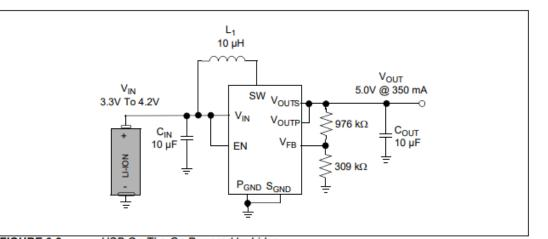
FIGURE 6-2: USB On-The-Go Powered by Li-lon.
