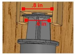
• *Figure 4*: A closeup view of the interface between the plunger of the syringe and the slot in the holding cap with dimensions labeled in inches. The leadscrew is fed through the holding cap so it is still able to interface with the plunger to depress it upon controller activation.
