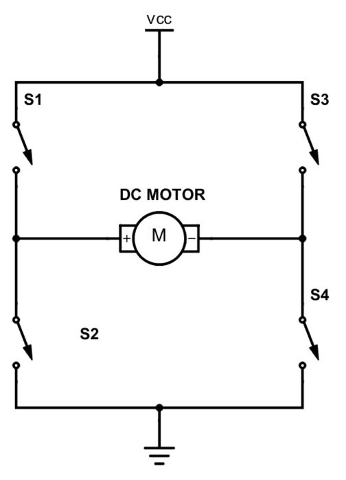
Figure 1. The topology of a typical H-Bridge.
