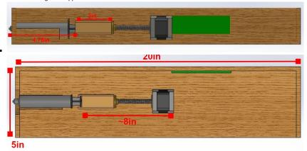
• Figure 3: A side and top view of the Lead Screw Plunge design with dimensions labeled in inches.
