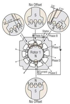
This diagram shows how the phases of the magnetic field unalign and realign and how it
