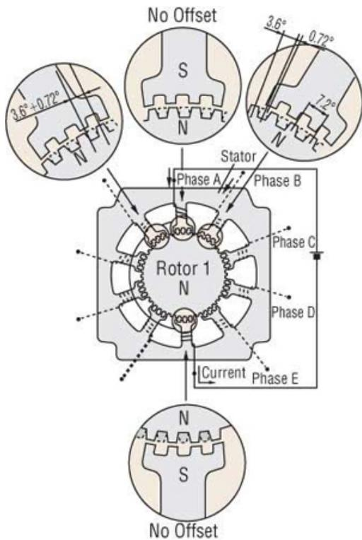
This diagram shows how the phases of the magnetic field unalign and realign and how it forces the rod in the middle to move.
