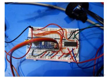
Arterial\_Line\_Poster.pptx.jpg(401 KB) - download Circuitry implemented on a breadboard. Includes the Arduino, stepper motor driver, and the lead outs for the potentiometer.
