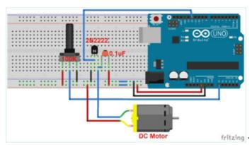
DC-Motor-Speed-Control-circuit-diagram-using-Arduino-and-Potentiometer\_0.png(64.2 KB) - download
