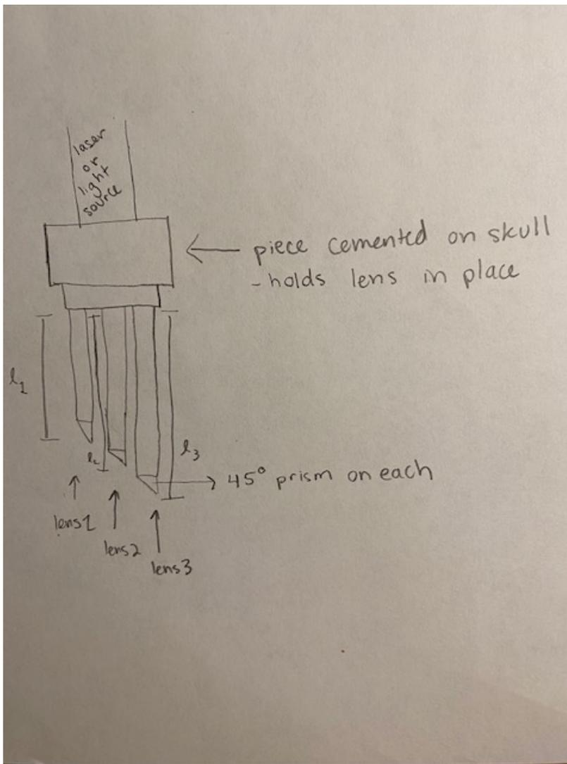
The final design I came up with was to have three separate length GRIN lens all placed in the ventricle at different depths. Again these designs would incorporate the prism to turn the field of view 90 degrees for longitudinal tracking.
