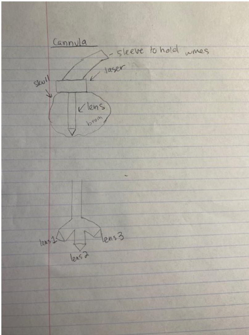
The ideas above all consist of a different cannula. The first image provides a visualization of what the current design looks like. The second image provides a different design for the cannula consisting of three separate slots for three separate lenses. Each lens would have a beveled structure to ensure no damage was inflicted on the surrounding tissue.
