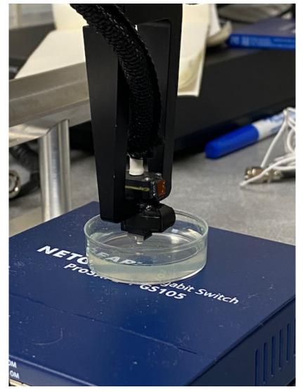
Figure 2: A close up of the miniscope over the top of the matrix. The petri dish is 35x10mm and the miniscope looks small next to it.
