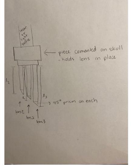
The final design I came up with was to have three separate length GRIN lens all placed in the vetricle at different depths. Again these designs would incorporate the prism to turn the field of view 90 degrees for longitudinal tracking.
