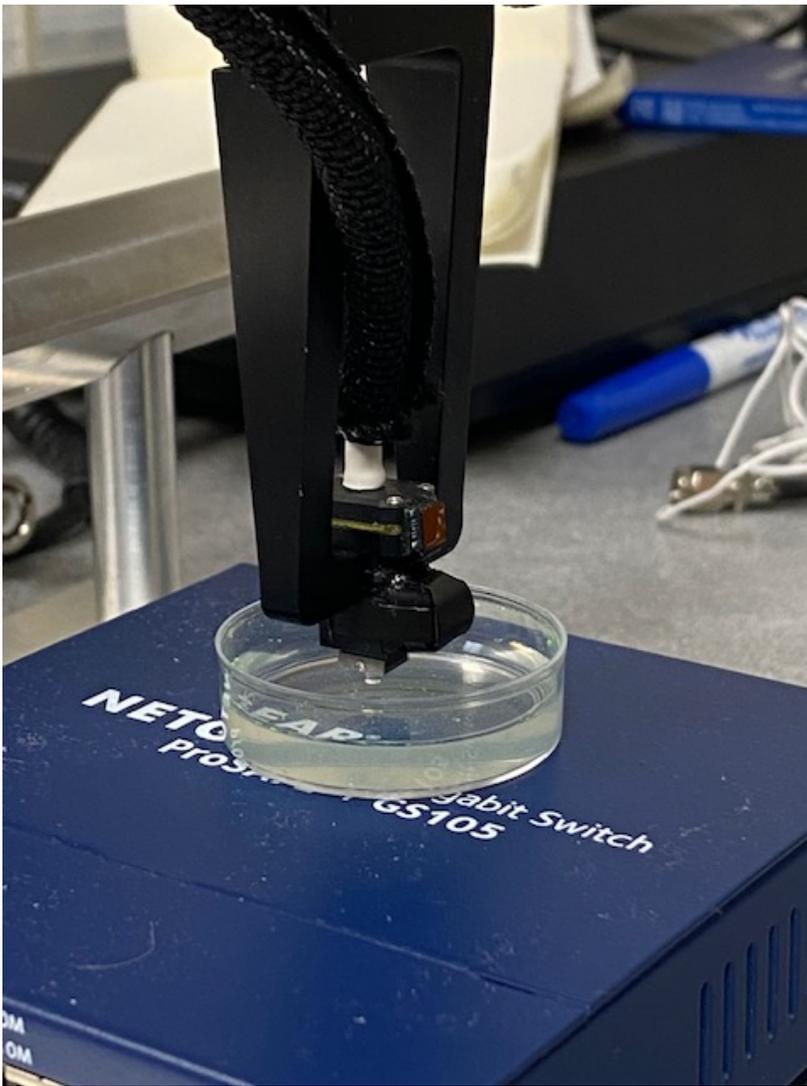
Figure 2: A close up of the miniscope over the top of the matrix. The petri dish is 35x10mm and the miniscope looks small next to it.
