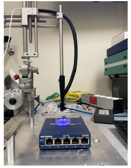
Figure 1: This image shows the setup as testing was running. The nVoke miniscope was used. It emits a blue light and records a green fluorescence.
