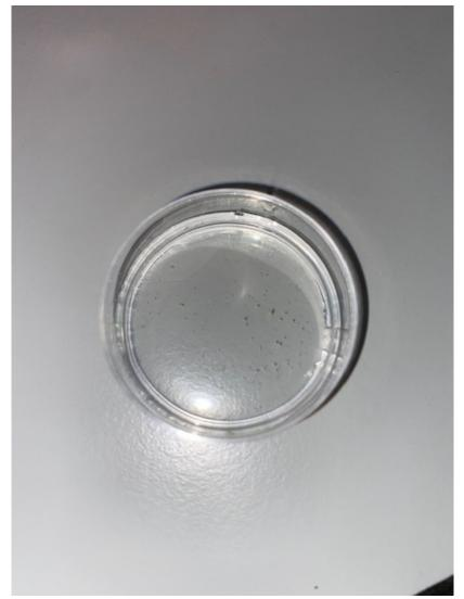
Figure 2: Pictured here is an image of a gel that has set overnight. The little green dots are the microspheres.
