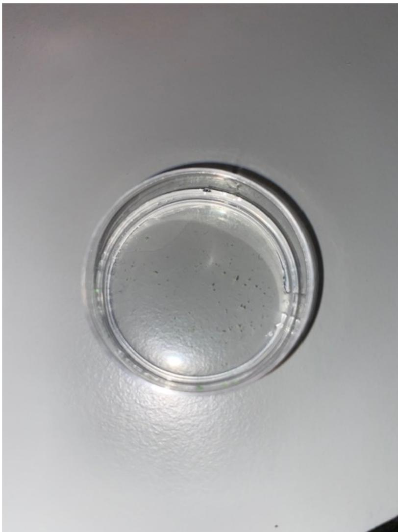
Figure 2: Pictured here is an image of a gel that has set overnight. The little green dots are the microspheres.
