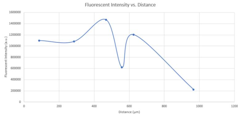
Figure 2: This graph shows the fluorescent intensity versus the distance from the left edge of the field of view. It is clear that at the center of the field of view (around 500 µm) the fluorescent intensity is the greatest. The intensity varies away from the center of the field of view with an outlier at 557 µm.
