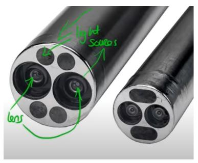
This model illustrates a traditional endoscope that is used commonly in medical practices. With this endoscope, there are light sources on both ends of the endoscope, with two lenses between the light sources. When the sources emit the light, they bounce back off the surface and back through the lenses for viewing. By modifying these concepts and making it both mini and implantable, it would be fairly feasible to design.
