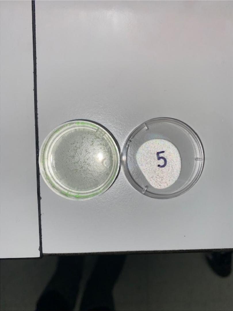
Figure 3: Pictured is gel 5 which contained the most amount of the spheres. This is apparent as more green dots can be seen without
