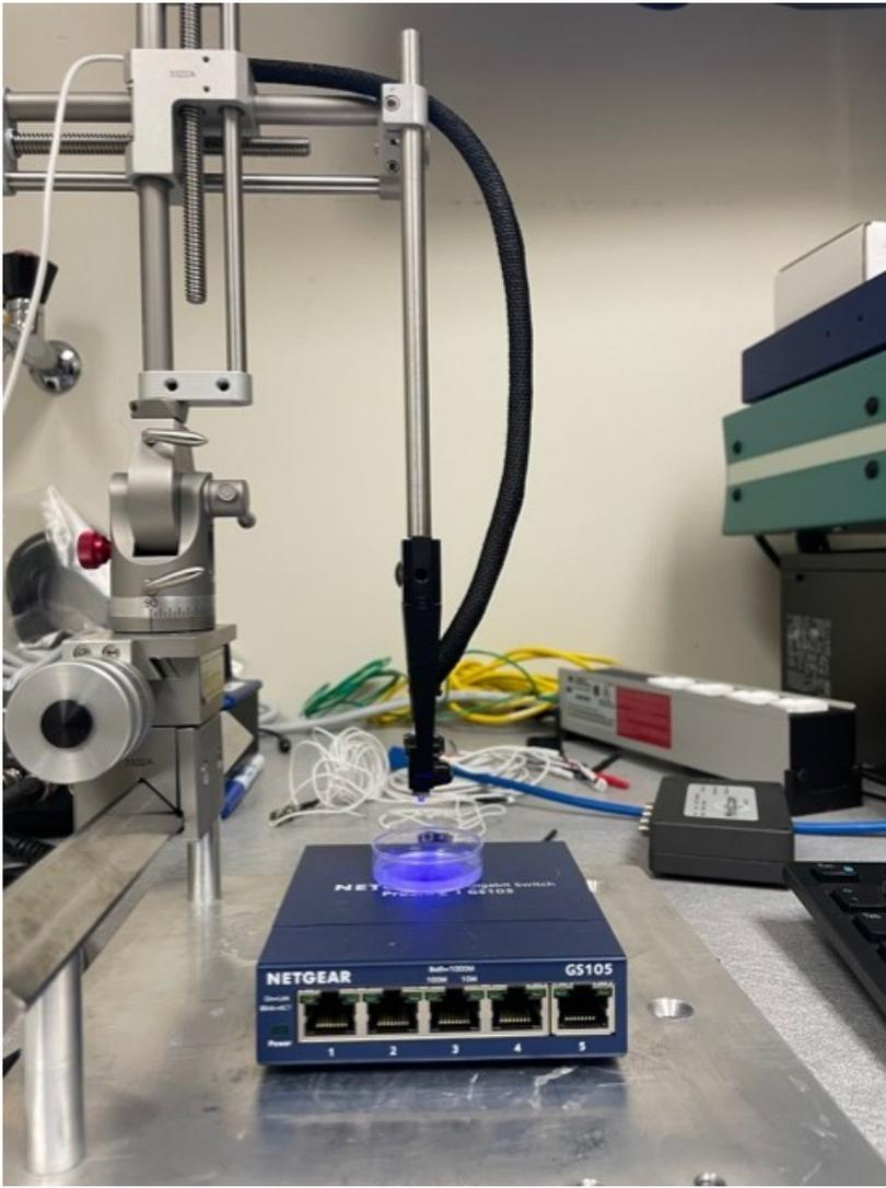
Figure 1: This image shows the setup as testing was running. The nVoke miniscope was used. It emits a blue light and records a green fluorescence.
