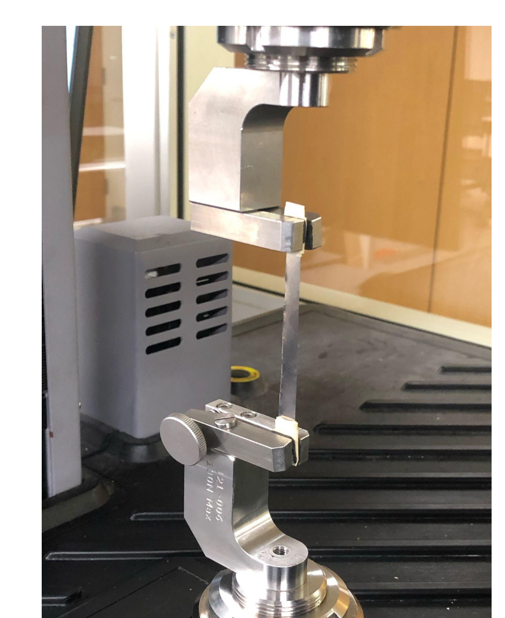
Figure 8: Sample being loaded into the MTS machine for tensile testing
