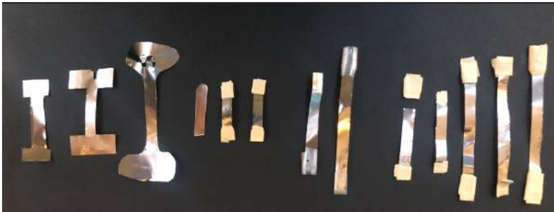
Figure 1: Samples that were used in the MTS Machine. A variety of methods above are shown that were used in attempts to avoid slippage such as the tape and dog bone cutouts.
