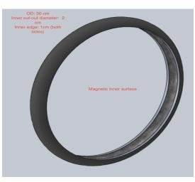
Figure 5: Guidewire Hoop. Dimensions: Outer Diameter: 30cm. Inner Diameter: 29 cm.
