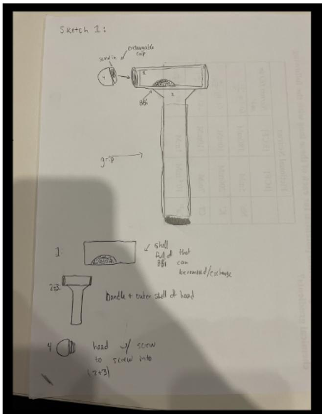
Figure 1: Sketch of my initial design idea. The image shows 4 images. 1: the total combined hammer with a screw in head and complete body. 2: is labeled 1 and shows a capsule of pellets that will slide into the hollow head of the hammer. 3: which is labeled 2+3 in the image shows the hollow head and the handle that is connected. 4: is the tip of the hammer that screws into the head and the handle.
