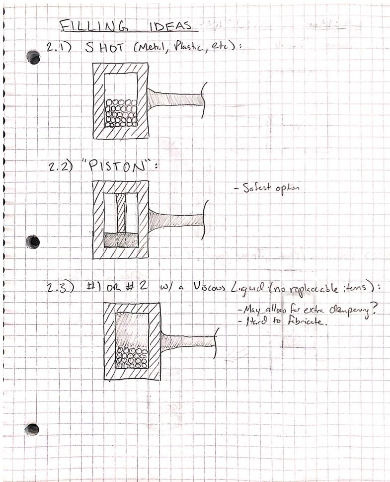
Figure 2: Three preliminary ideas for the filling of the hammer for the energy distribution (dead-blow effect).
