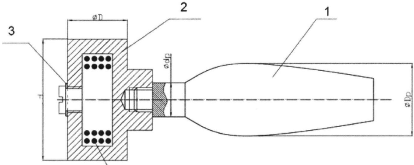
Figure 1: Drawings of the patent of interest for the design of a Dead-Blow Hammer.
