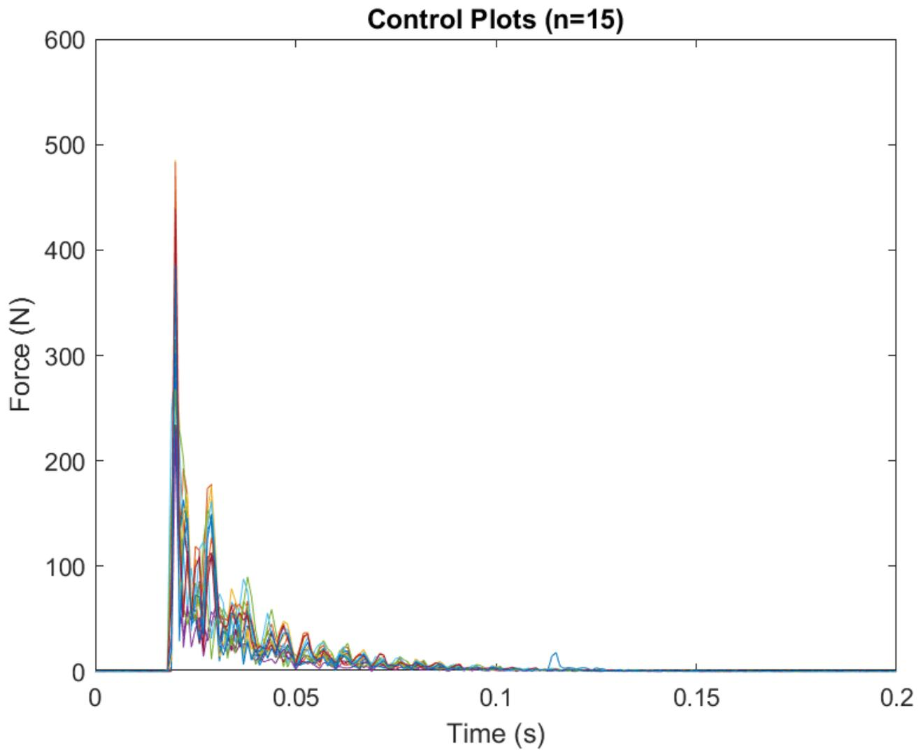
Figure 1: Force-time plot for the control mallet.
