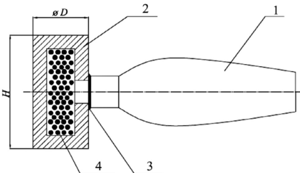
Figure 1: The low-inertia impact hammer studied in the paper [1]. This resembles a dead blow hammer.
