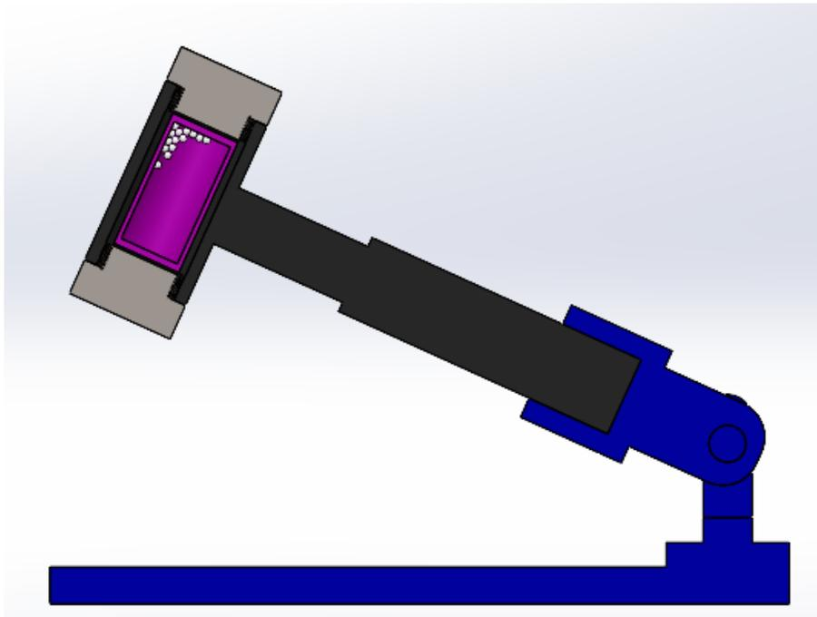
Figure 1: Screen shot of a frame of the motion study when the mallet is on a downward swing. The beads are visible in the chamber.
