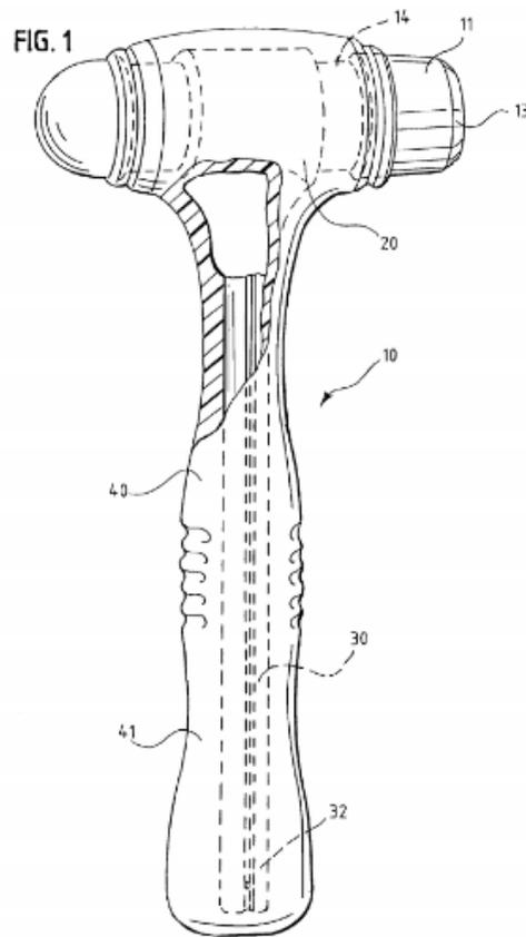
Figure 1: This complete dead blow hammer is shown with the outer casing that is used to provide grip and comfort for the person using it. The hammer has a tubular head with a cylindrical collar. (Figure is taken from the patent attached).
