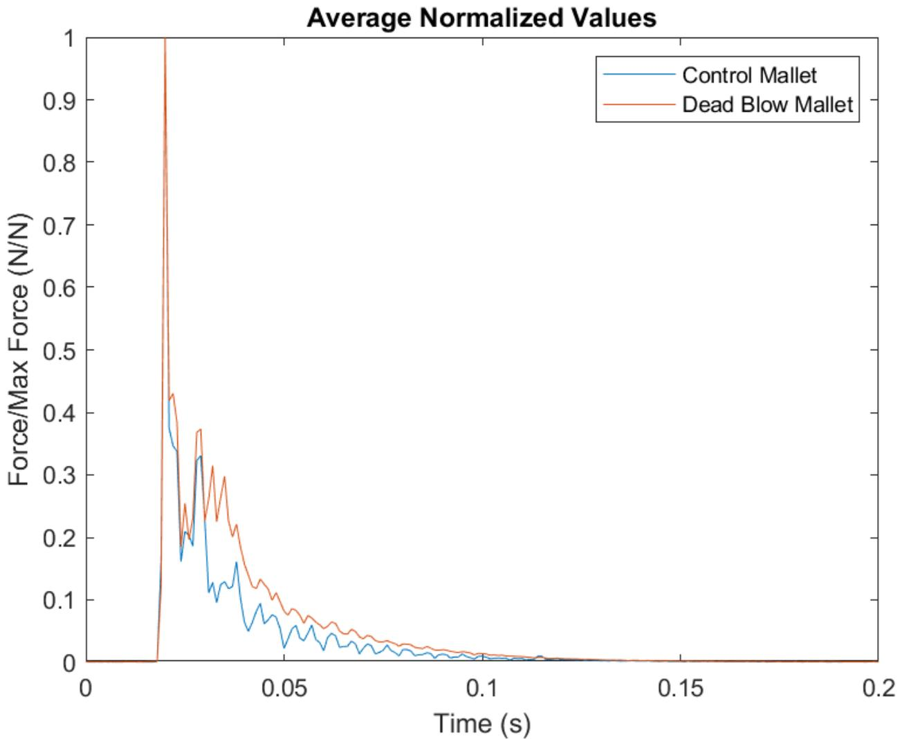
Figure 4: Force-time plot for the average normalized force characteristics of both the dead blow and control mallets.
