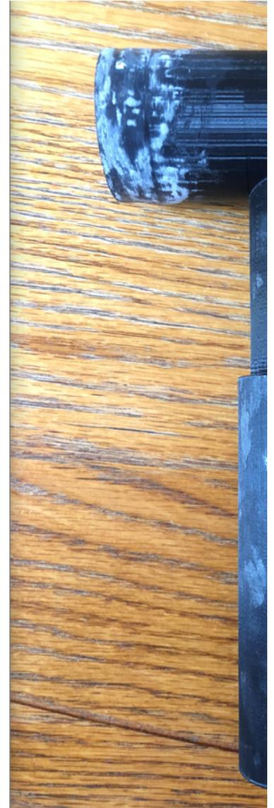
Figure 1: Images of the dead blow mallet. The end caps are sealed with epoxy to ensure they do not come apart during testing.
