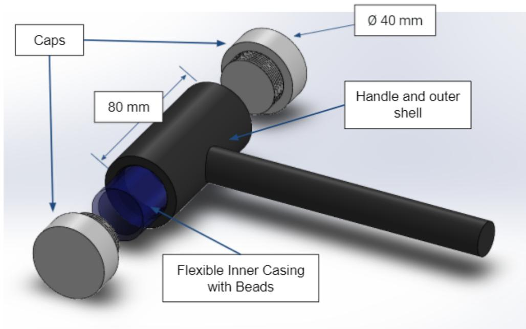
Figure 1: Solidworks design of the hammer.
