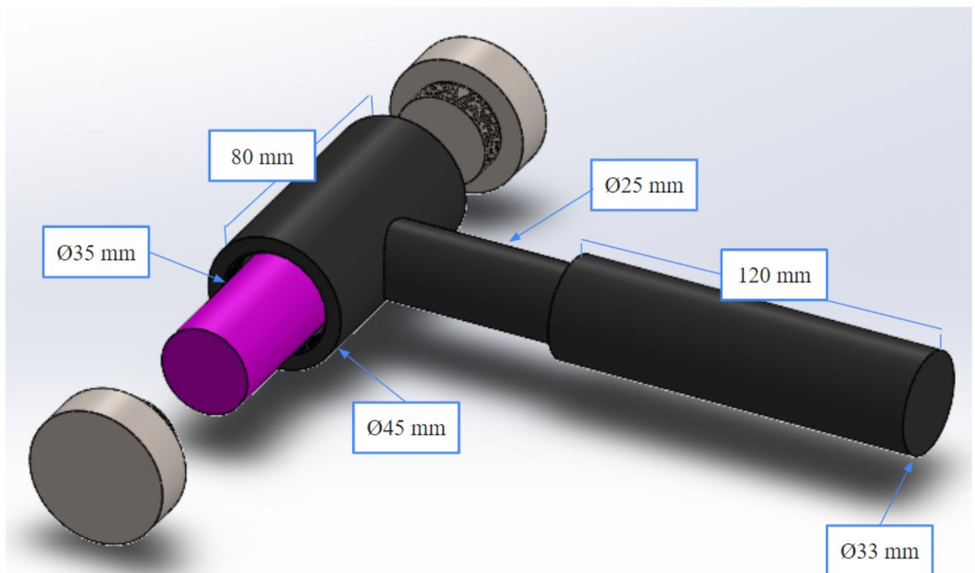
Figure 1: Redesign of the mallet. This takes into consideration maximizing ergonomic comfort for the surgeon.
