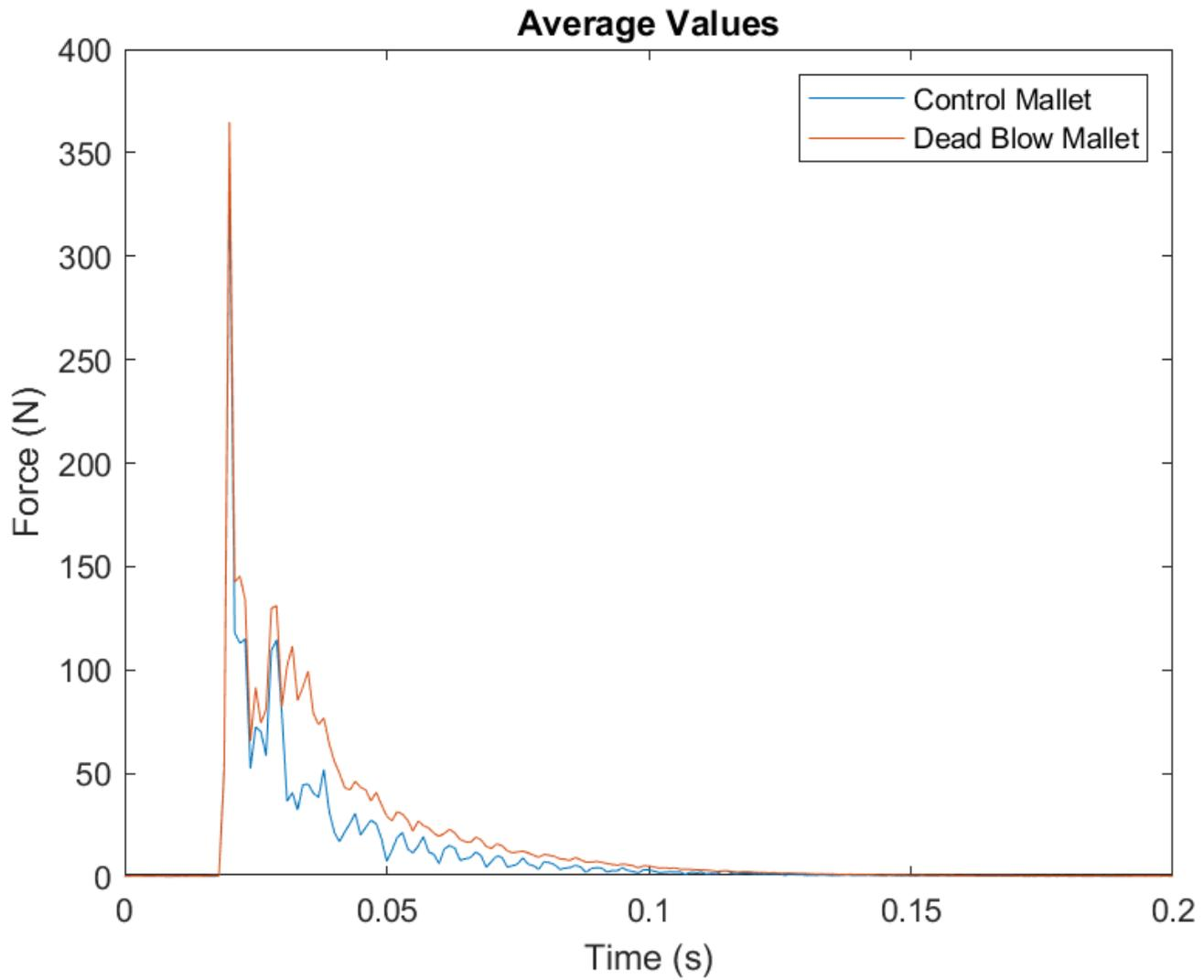
Figure 3: Force-time plot for the average force characteristics of both the dead blow and control mallets during testing
