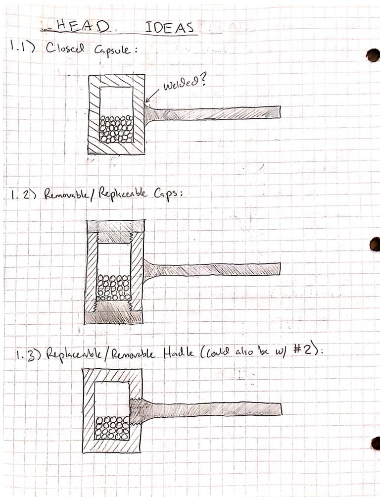
Figure 1: Three preliminary ideas for the head of the hammer. Drawn/conceptualized on 9/17/2021.
