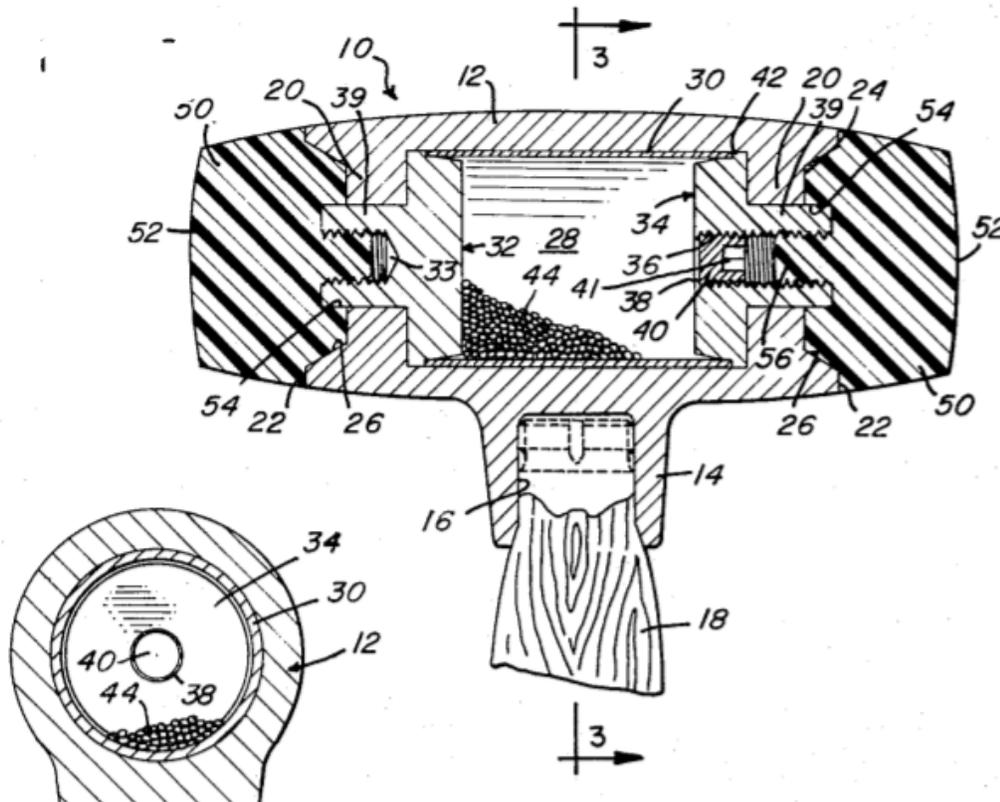
Figure 1: Image in the patent of interest detailing a dead-blow hammer design for the head of the mallet. Includes removable caps.
