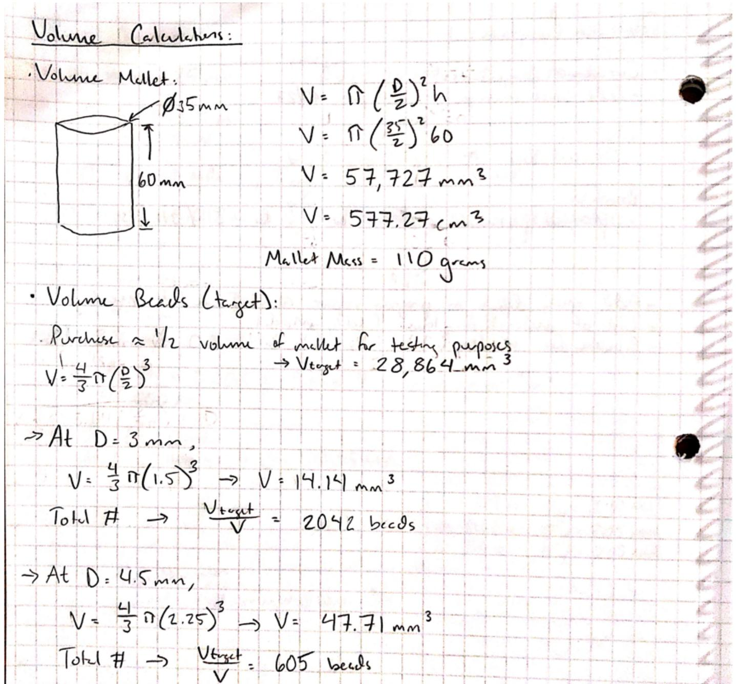
Figure 1: Calculations for the volume of the inner chamber and beads.
