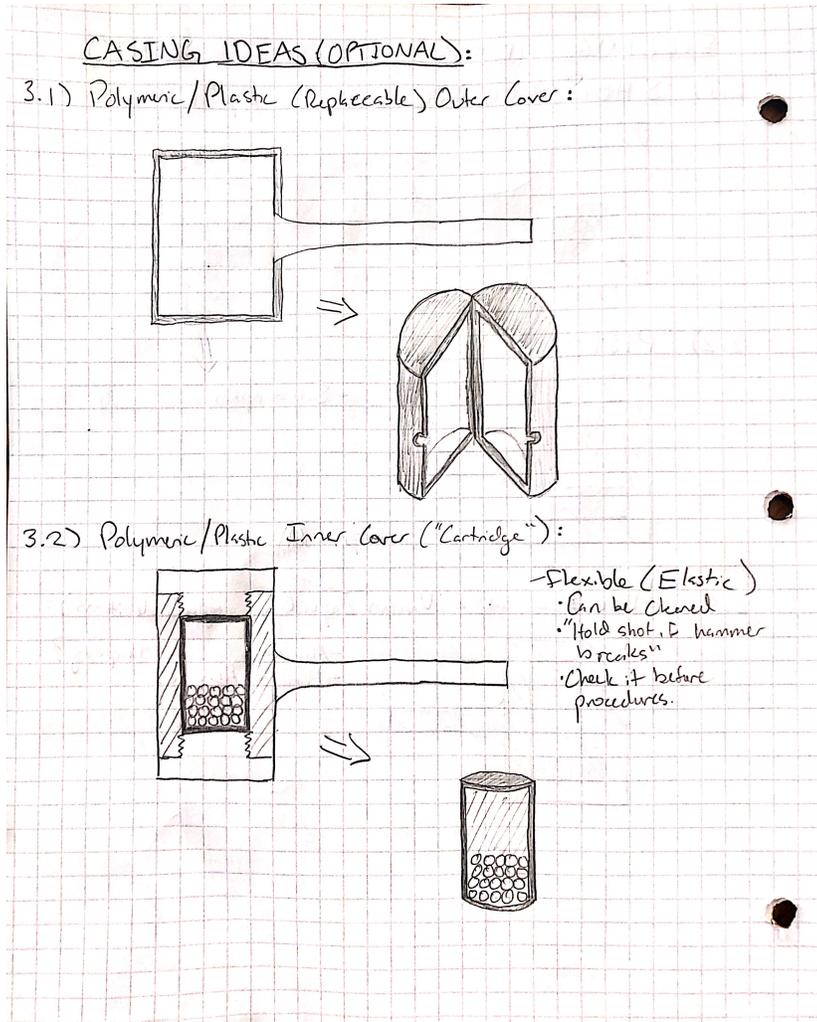
Figure 3: Three preliminary ideas for the optional casing of the hammer. The goal behind the casing is to provide an extra layer and protect the patient from the bead filling. Drawn/conceptualized on 9/17/2021.
