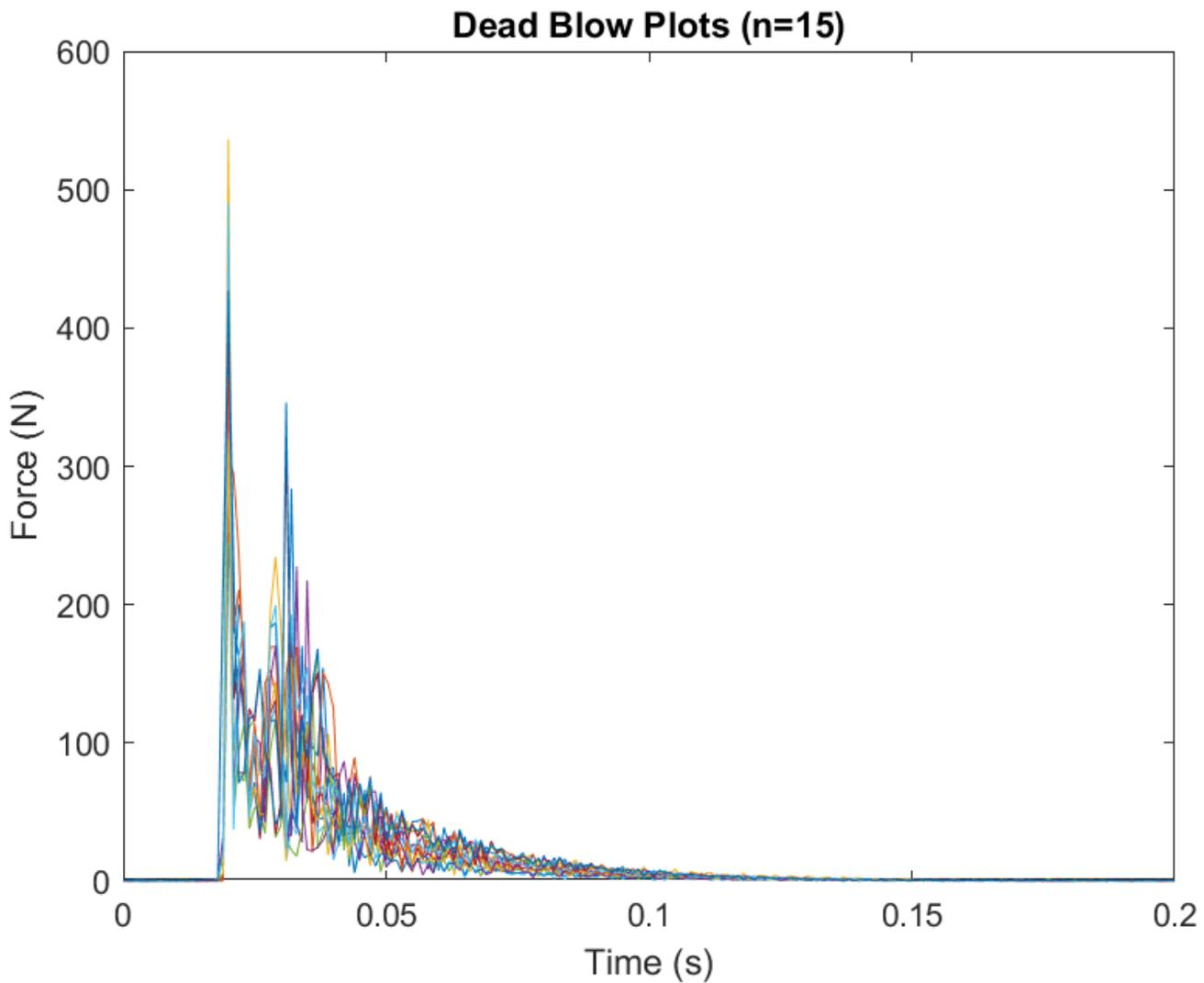
Figure 2: Force-time plot for the dead blow mallet.
