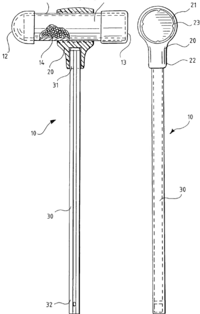
Figure 1: Drawings of the patent of interest for the design of a Dead-Blow Hammer.
