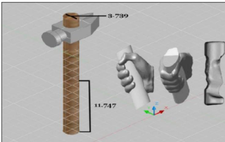
**Fig 8: CAD design of newly designed hammer**
