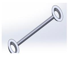
Figure 3: Assembly of the initial ring and support bridge
