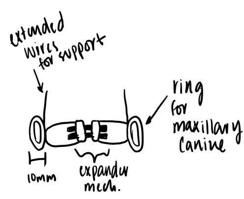
Figure [2]: The ring design integrated with a palate expander
