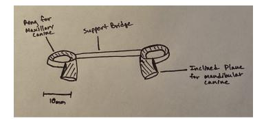
This design is similar to the expired patent researched on 9/24/21. It features two rings to be mounted onto the upper maxillary canines, two inclined planes on each ring, and a support bridge. This design minimized variables and ultimately the need for software as our client can simply take measurements of the inside of the patient's mouth and alter the dimensions in solidworks.
