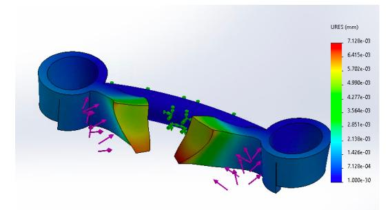
Figure 3: Demonstration of deformation from forces implied on the product during solidworks stress testing.
