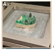
Figure 2: The mold being vacuum sealed
