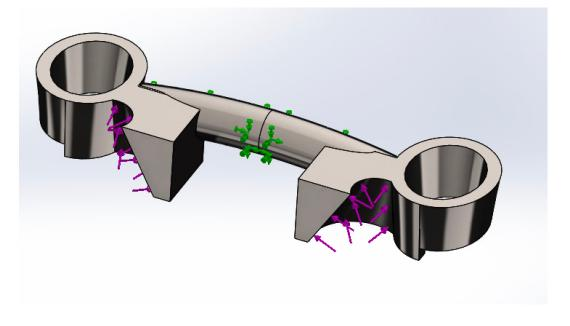
Figure 2: Demonstration of the forces on our device. The purple arrows show the applied force, and the green arrows show what is fixed.
