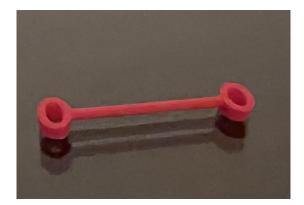
Figure 4: 3D printed PLA version of the initial design of the ring and support bridge.
