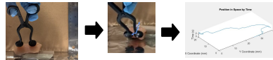
Figure 7: Simulated surgical displacement of one lobe of the thyroid gland, using a tissue analog(left). The video file is analyzed in motion capture software Kinovea (center) and exported to Matlab to determine maximum acceleration and forces
