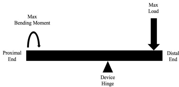
**Conclusions/action items:** Add a safety factor of at least 2 to determine the appropriate cross-sections of both ends.
