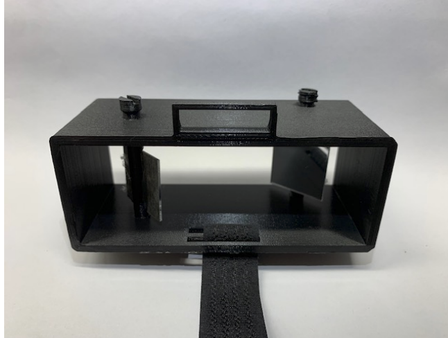
Figure 10. The 3D printed mirror array final design. The two pins can be turned to adjust the angle of the mirrors for calibration. A velcro strap can be wrapped around the smartphone, fed through the plastic loop shown at the top of the array, and folded onto itself to secure the smartphone.
