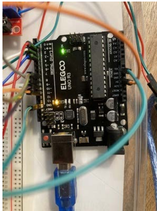
IMG_6142.jpeg (3.13 MB) Closeup of Arduino for 3 limit switches with interrupt.
