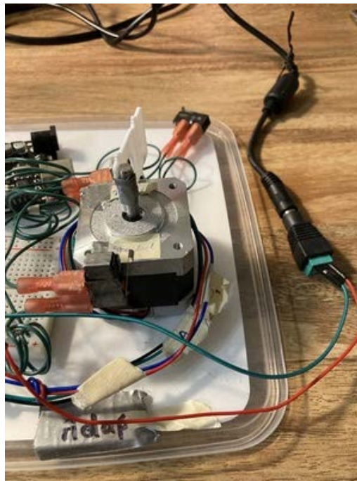
IMG_6265.jpeg (3.49 MB) An image showing the stepper motor and limit switches. Also off to the side is the 12V power supply connector.
