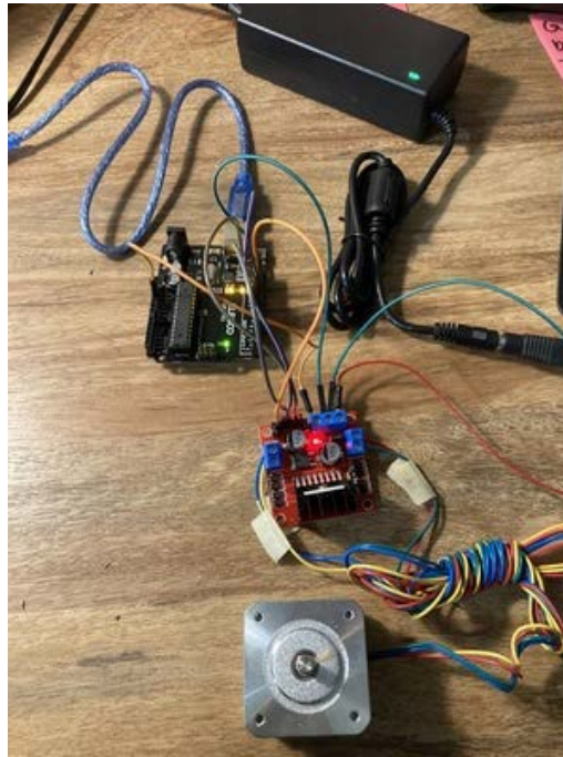
IMG_6127.jpeg (4.28 MB) Overall circuit for example stepper code using L298N.
