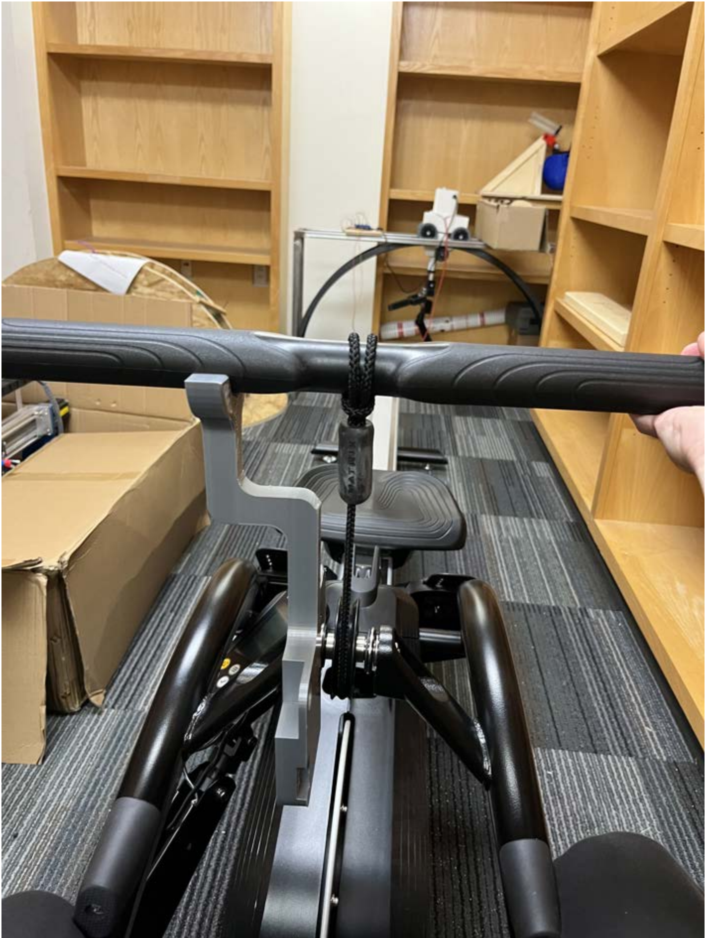
The above image shows the antler holding the handle bar, and the bar being too thick to fit well in the cavity.
