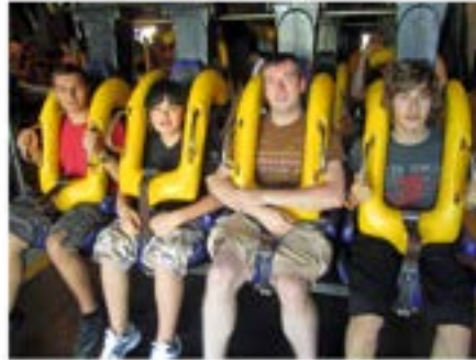
The OTSR secures a rider into their seat, preventing them from falling out on slow inversions or high-negative-G moments.
