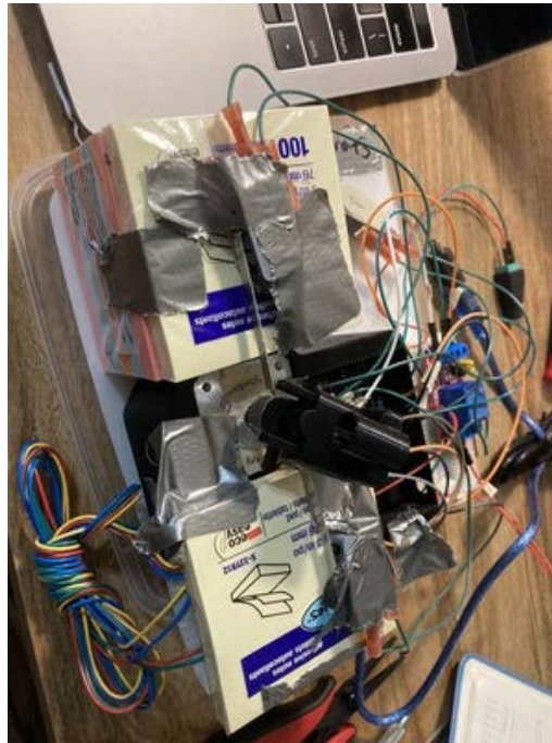
IMG_6228.jpeg (3.48 MB) Image showing the standard and adaptive position limit switches relative to the console flag.
