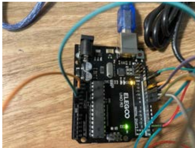
IMG_6135.jpeg (4.19 MB) Closeup of Arduino for 1 limit switch with polling.
