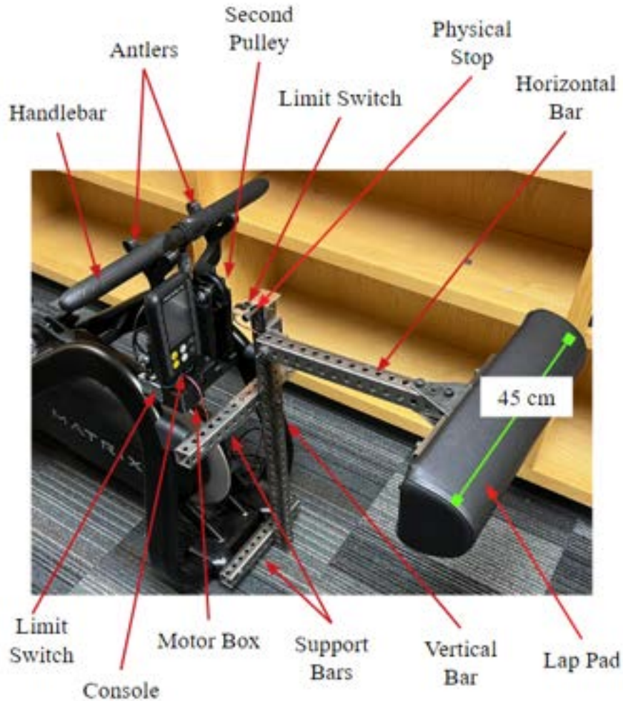
Figure #. Full Assembly. The full assembly includes the pulley support plates with antlers, the console rotator and electronics box, and the metal adjustable stabilization frame. The wheelchair is held fixed using the downward pressure from the lap pad.
