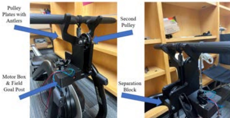
Figure #. Full Physical Assembly. The pulley plates with antlers, console rotation field goal posts, and motor box of the full rower assembly are shown in a front (left) and back (right) view.
