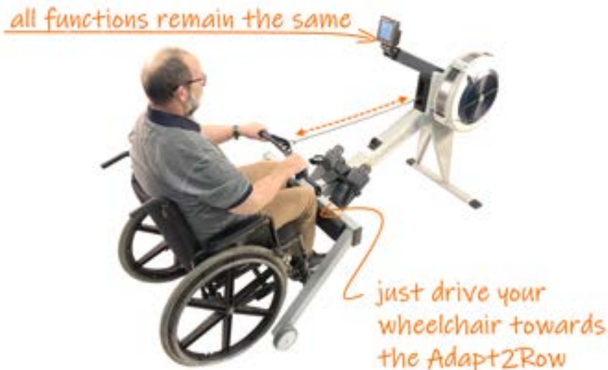
Figure 2. Adapt2Row on a Concept2 Rowing Machine. Adapt2Row allows for both standard and adaptive rowing on the Concept2 rowing machine but still requires outside assistance to transition between both states [9].
