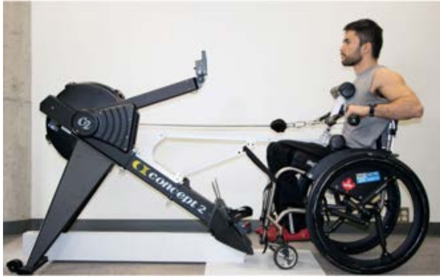
Figure 1. AROW adaptations to Concept 2. Adaptations for the Concept 2 include a support bar extending to the user's chest and a rigid attachment to the frame of the rower [7].
