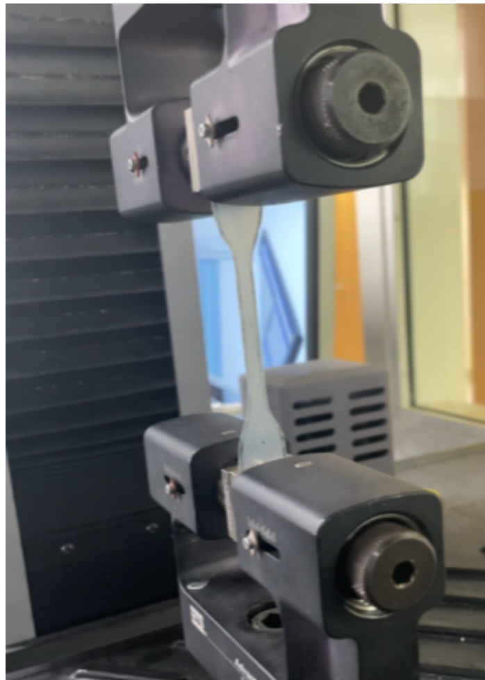
Figure 9: MTS testing setup for hydrocolloid bandage.
