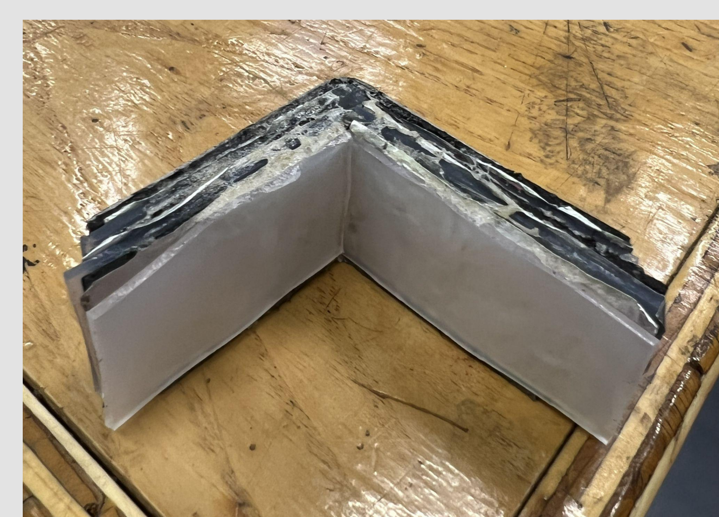
Fig. 7: The layers of the corner damper, organized in the order of foam, foil, gel, foil, repeated three times. The layers were secured using a spray adhesive.
