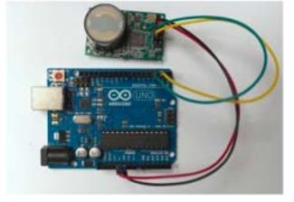
Figure (2): CO2 Sensor and Arduino Control
