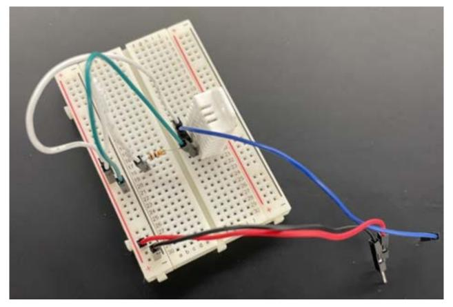
Figure 2: DHT22 sensor hardware set up
