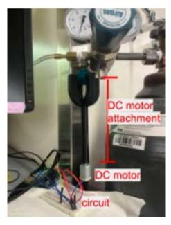
FIGURE 1: CO2 Testing Setup
