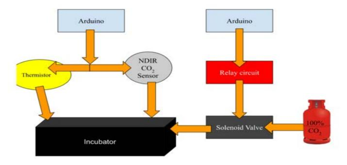
Description of Code: Approximately every minute, the temperature, humidity, and CO2 values are read and outputted onto serial monitor. The Solenoid valve opens if CO2 value is <4.5% and closes when CO2 is >5.5%.
