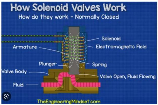
TheEngineeringMidset, How Solenoid Valves Work - Basics actuator control valve working principle. YouTube, 2019.
