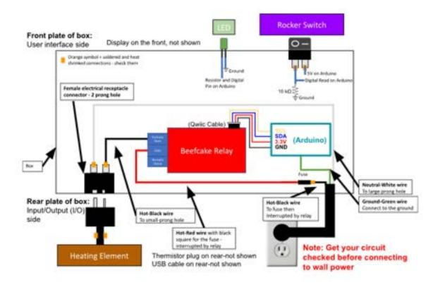
Figure 15. Connections between the Beefcake Relay, wall power, Rocker switch and Arduino.
