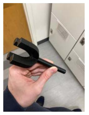
FIGURE 5: Final 3D Printed PLA Plastic Valve holder:
