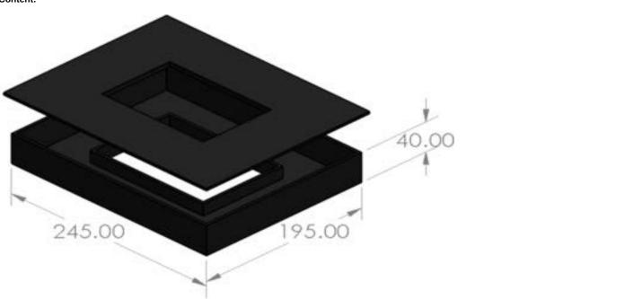
Figure 1: Hinge Top Acrylic Incubator drawing with dimensions in millimeters.
