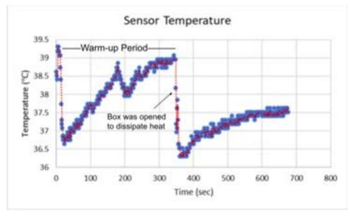
FIGURE 1: Full Incubator Temperature Testing results
