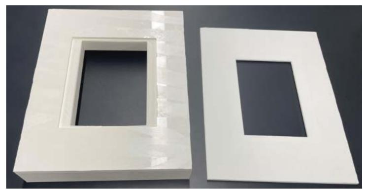
Team activities/Project Files/Spring 2022/Design Process/Previous Semester's Work/Team activities/Fabrication/11/29/2021 Box Fabrication: 3D Print186 of 685 Figure 2: Bottom view of incubator box and crown 3D prints
