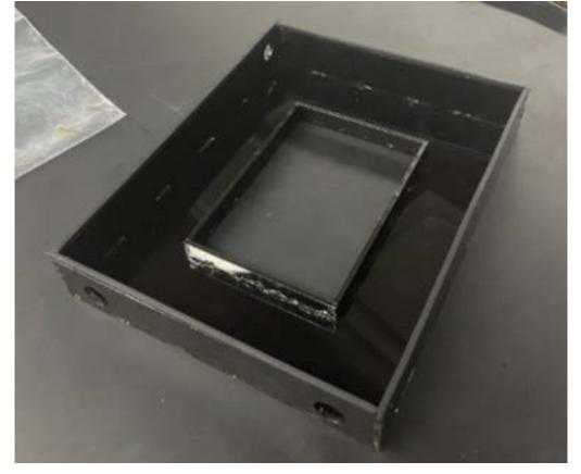
Figure 2: Assembled black acrylic box after being laser cut.
