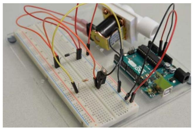
Figure 4: Final Solenoid Valve Arduino Setup
