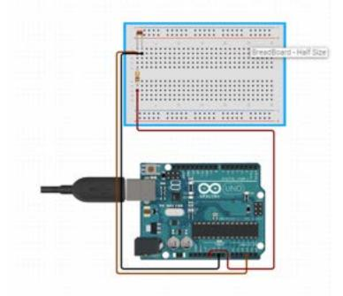
Figure 1: Thermistor hardware set up.
