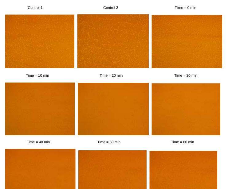
**Conclusion:** Upon visual examination of the glass, one could see that condensation had formed after 10 minutes of running the system, and optics slowly deteriorated. 8 pumps are not enough to prevent the formation of condensation. Will quantify this data soon.
