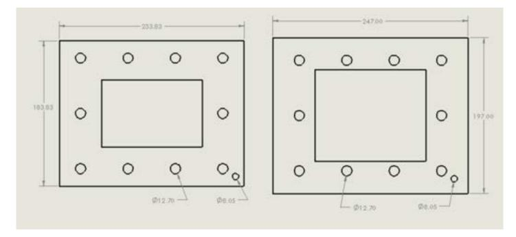
Figure 1: Incubator test lid drawing
