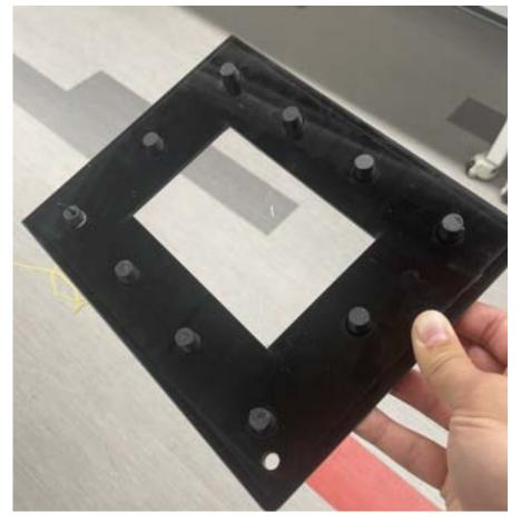
Figure 3: Incubator test lid bottom with plugs and thermistor in.
