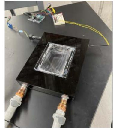
Figure 2: Final design fabrication with an closed lid.
