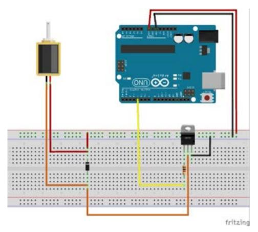
Figure 2: Solenoid Valve Schematic Diagram
