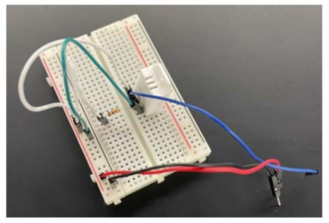
Figure 2: DHT22 sensor hardware set up
