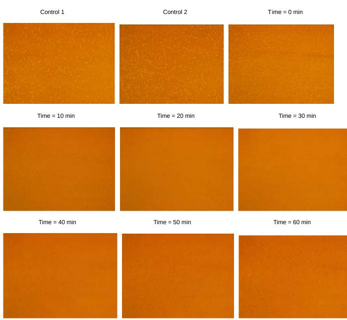
**Conclusion:** Upon visual examination of the glass, one could see that condensation had formed after 10 minutes of running the system, and optics slowly deteriorated. 12 pumps are not enough to prevent the formation of condensation. Will quantify this data soon.
