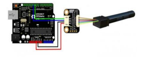
Figure 3: CO2 sensor hardware set up
