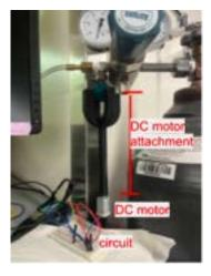
Figure 3: Testing setup with motor, valve holder, and circuits all attached to the CO2 tank
