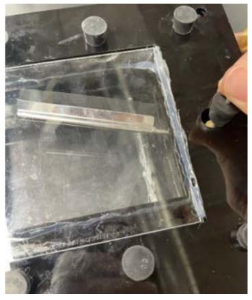
Figure: Wiper fabrication with rubber stopper as knob.
