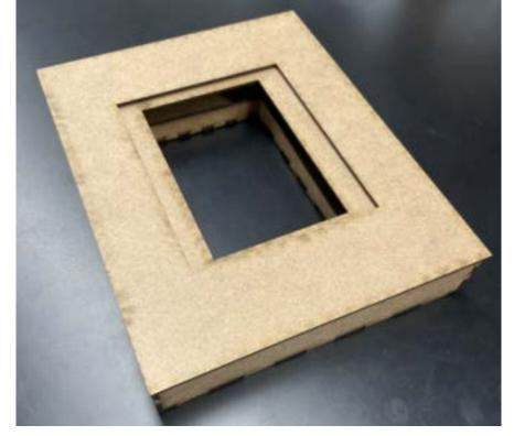
Figure 2: Photo of the laser cut HDF prototype with all the pieces assembled together.
