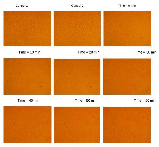
**Conclusion:** Upon visual examination of the glass, one could see that condensation had formed after 10 minutes of running the system, and optics slowly deteriorated. 4 pumps are not enough to prevent the formation of condensation. Will quantify this data soon.
