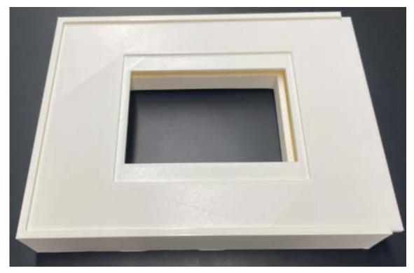
Figure 3: Assembled 3D printed incubator box.
