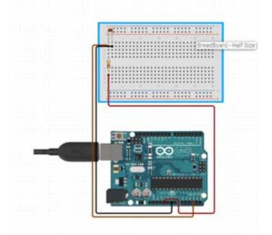
Figure 1: Thermistor hardware set up.
