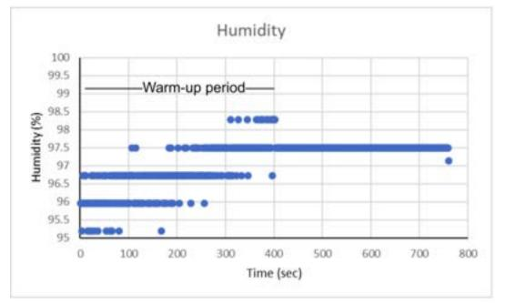
FIGURE 2: Full Incubator Humidity Testing results
