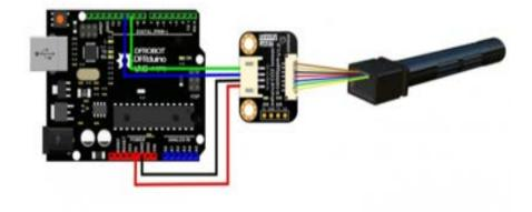
Figure 3: CO2 sensor hardware set up
