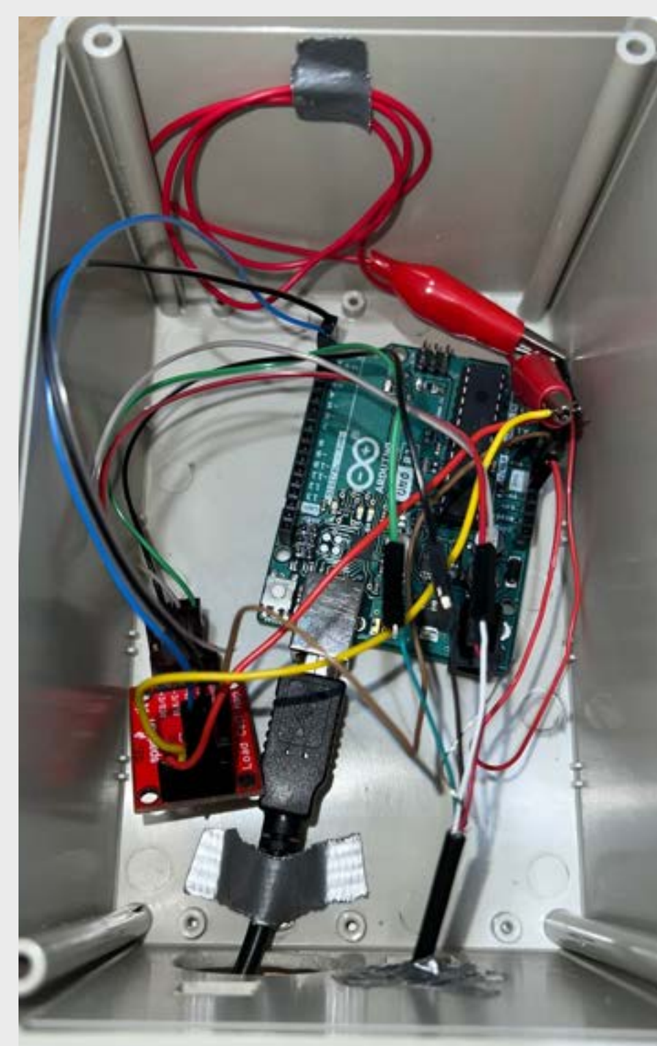
Figure 2. Load cell and Arduino circuit.
