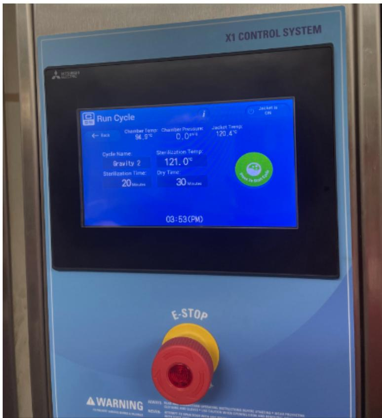
Figure 1: these are the specs we used to run the autoclave, they were already pre-populated when we arrived
