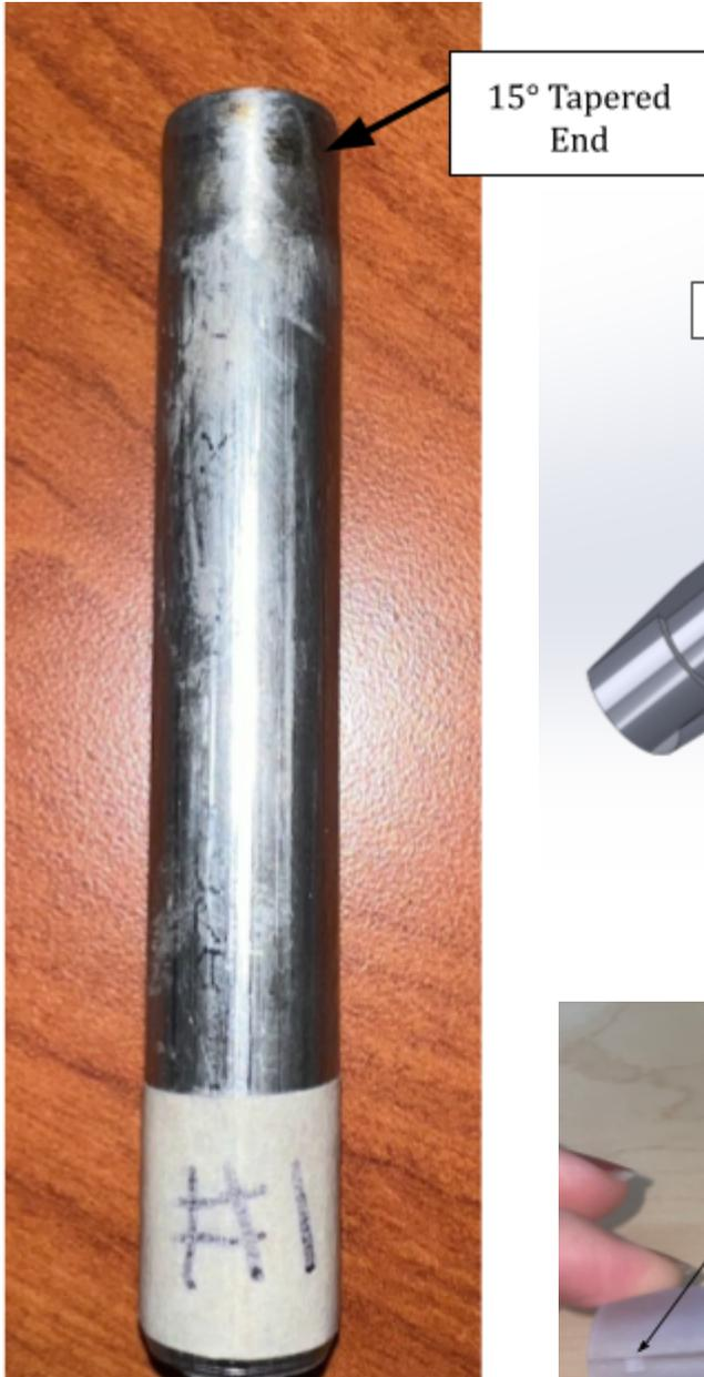
**Figure 12:** Stainless steel "Punch Biopsy" blade made in UW TEAM Lab.
