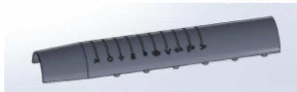
**Figure 21:** SolidWorks model of the tube with icon markers: 10 slits 1.5cm each, 0.5cm apart with accompanying icons.
