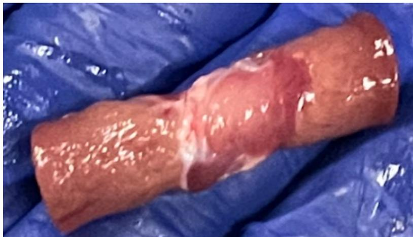
**Figure 19:** Image of staircase damage within internal tissue caused by Blade #3.
