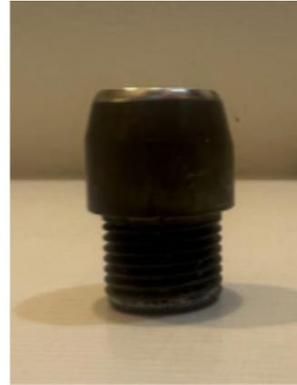
**Figure 3:** Previous group's prototype of the stainless steel blade with a 1.59cm outer diameter.
