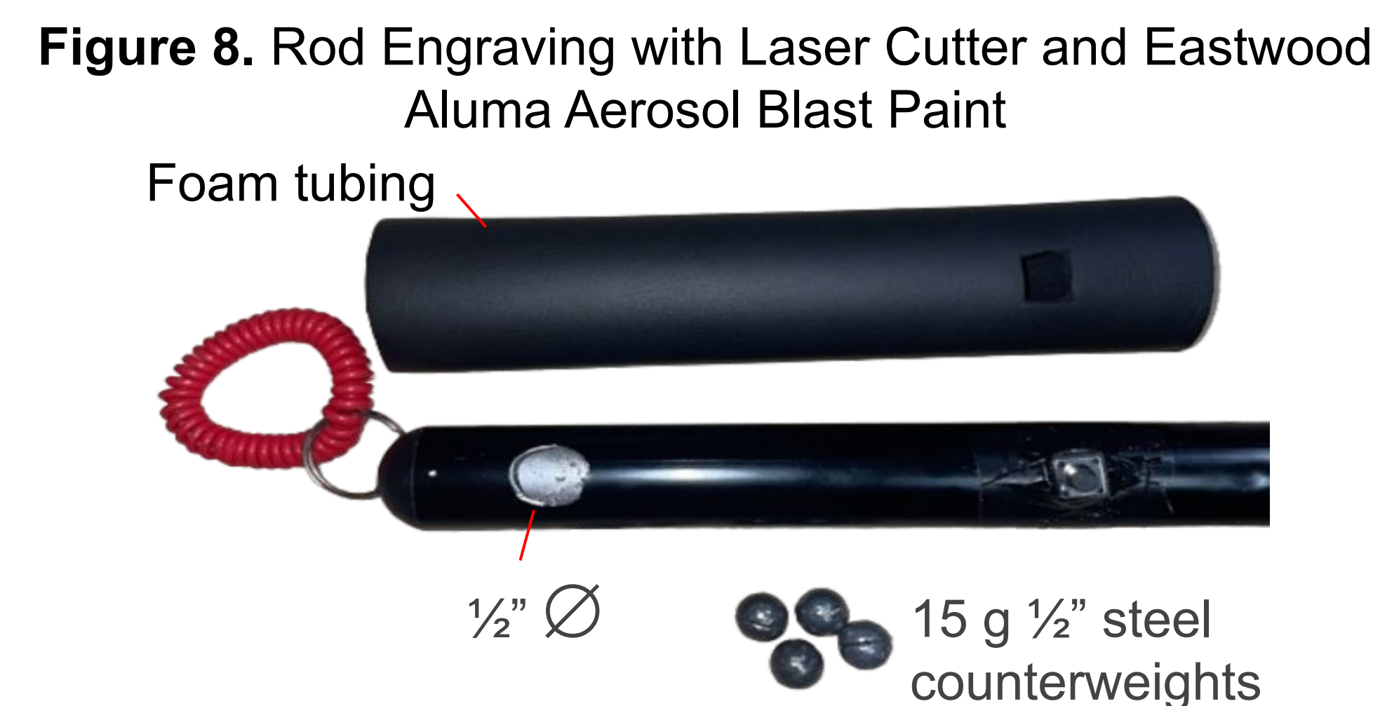
Figure 8. Rod Engraving with Laser Cutter and Eastwood Alumina Aerosol Blast Paint
