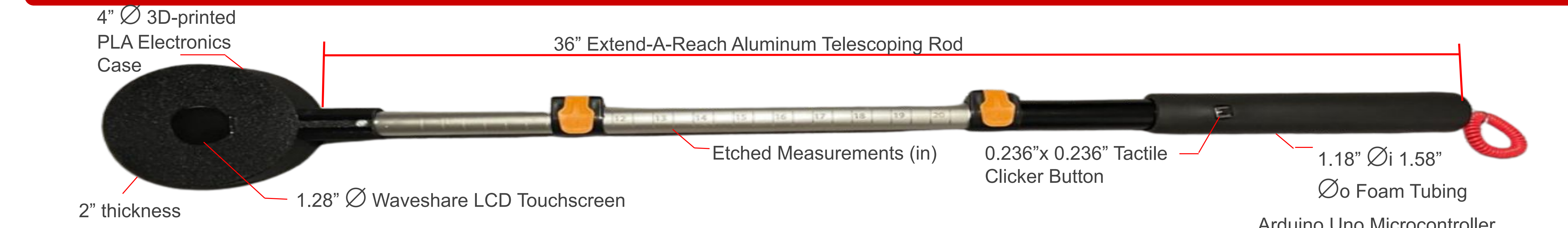
Figure 6. Final Prototype: Display Case, Telescoping Rod, Foam Handle, and Electronics
