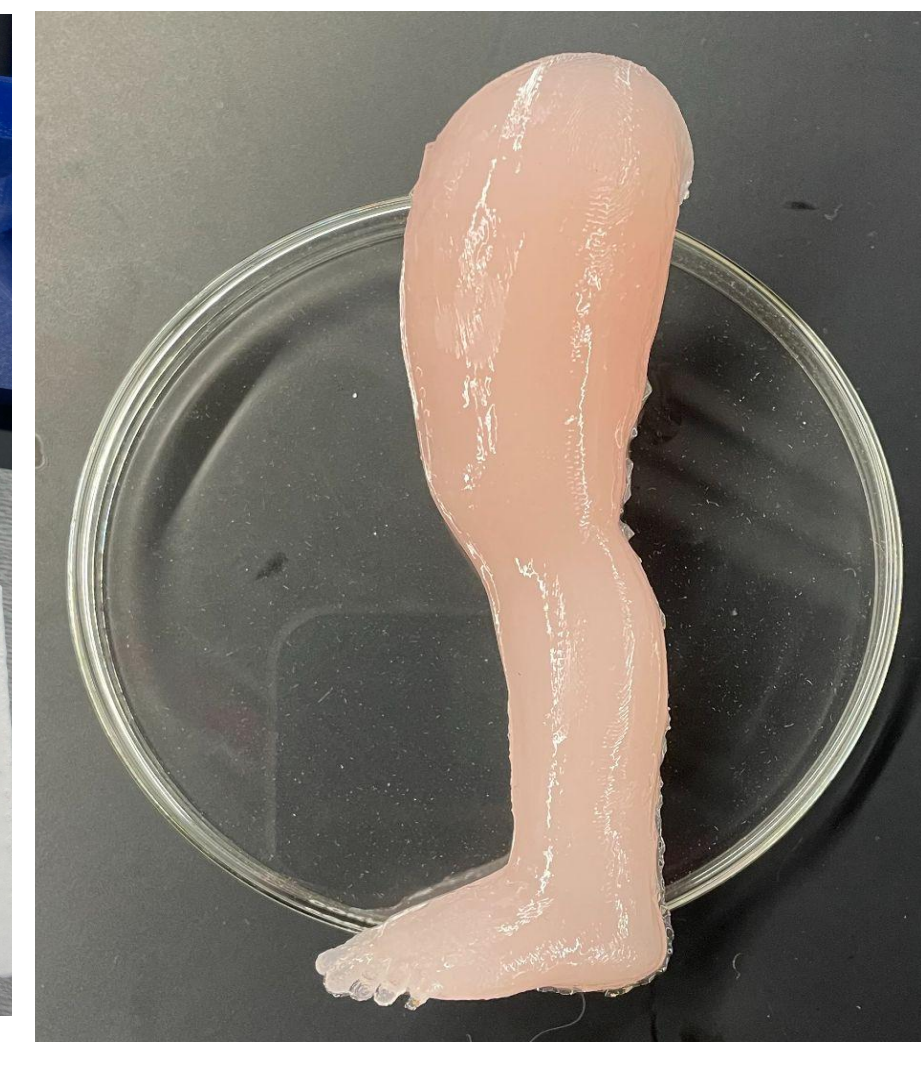
Figure 6: Leg Coated in PDMS Skin Material
