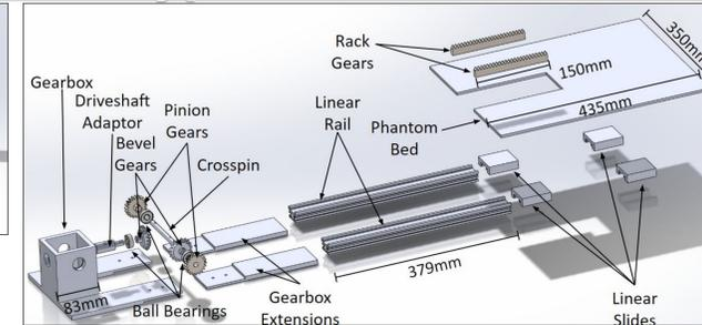
Figure 4. Gearbox and Platform Assembly
