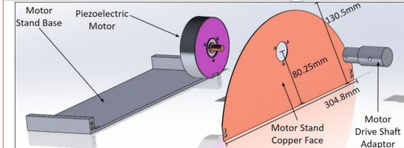
Figure 3. Motor Stand Assembly
