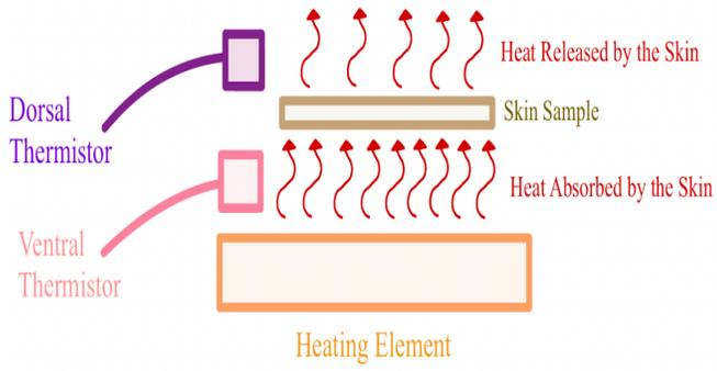
This image provides an illustration of the overall idea of the design and how the thermistors and heating element interact with the skin sample.
