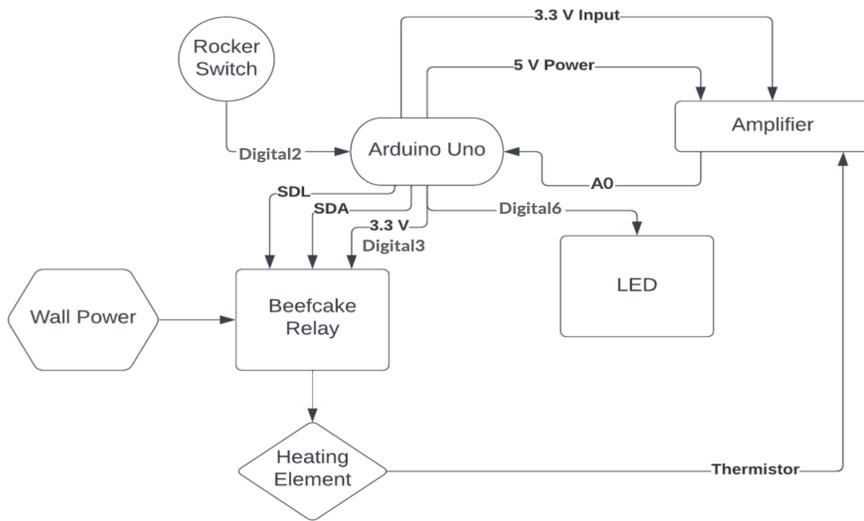
A hardware block diagram of the proposed thermistor circuit
