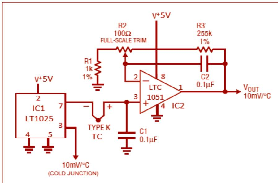
Circuit schematic for the use of a K-type thermocouple
