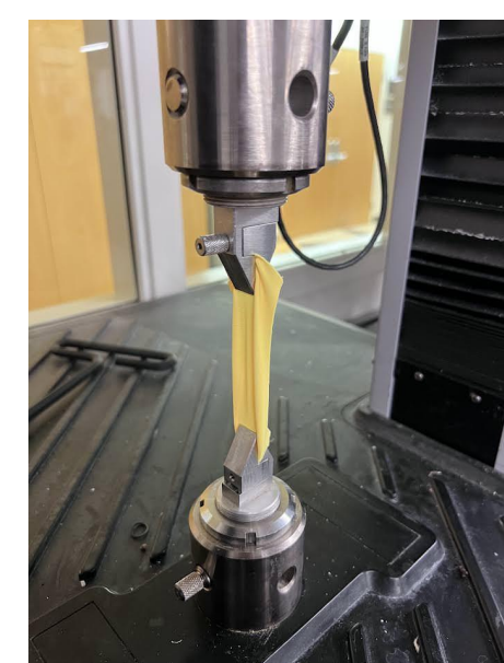
Figure 7: Full muscle model including muscle, muscle fabric, and tendon sewed on, stress vs strain curve.
