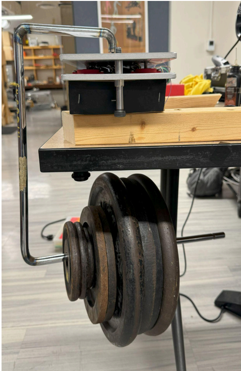
Figure 31. Accuracy testing setup using point load application mechanism.
