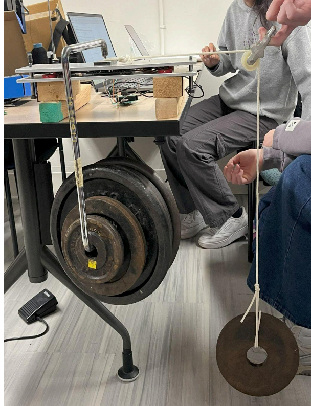
Figure 33. Shear loading test setup.
