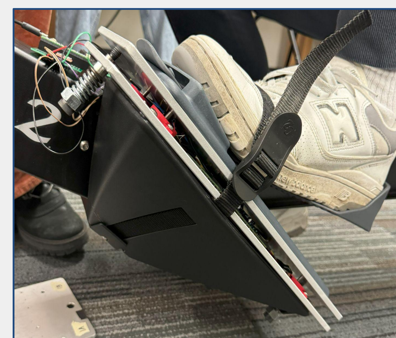
Figure 3. Side view of left foot plate assembly attached to the Ergometer.
