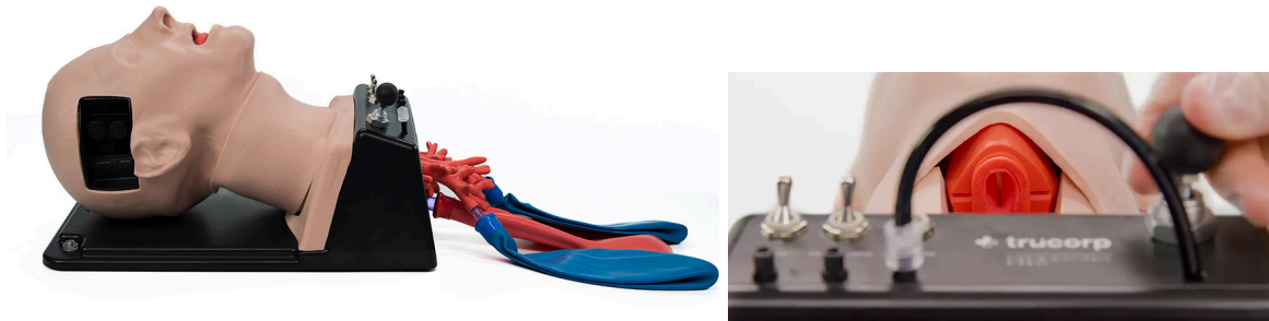
Figures 2 and 3: TruCorp Airsim Difficult Airway Trainer and the simulated laryngospasm it can produce [5]
