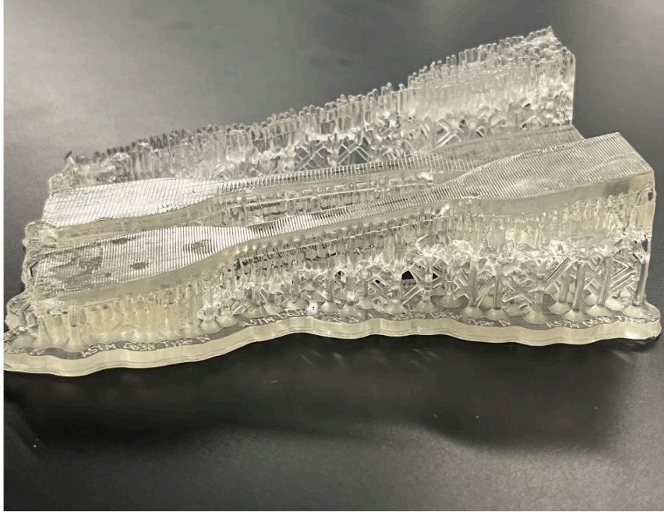
Figure 17: Type IV dogbones with 3D-printed support structures still attached
