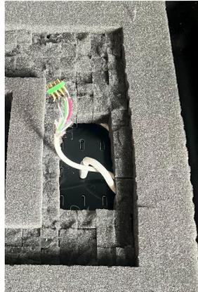
*Figure 22: Charging System with USB-C to Pogo Pins Connection*
