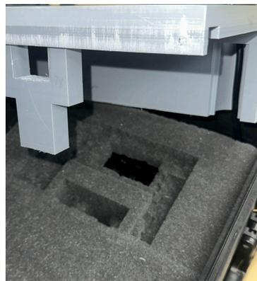
*Figure 23: Altered Foam Inserts Under the Tray*
