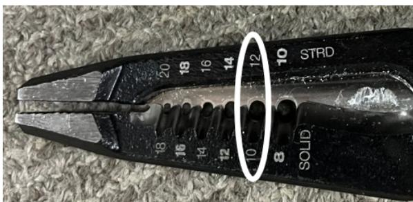
**Figure 16:** Wire Cutter with Correct Hole Size
