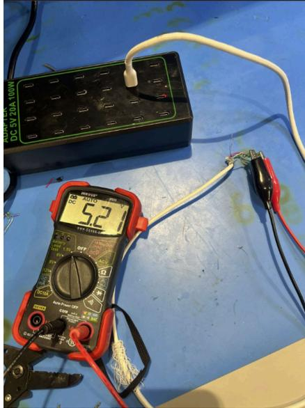
*Figure 27: Reading of 5.21 V on multimeter when connected to fully soldered pogo pins and USB*
