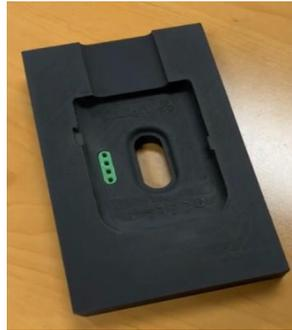
**Figure 14:** Unit Cell Design with Pogo Pin Holder
