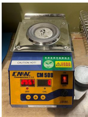
*Figure 18: Lead-Free Soldering Pot*
