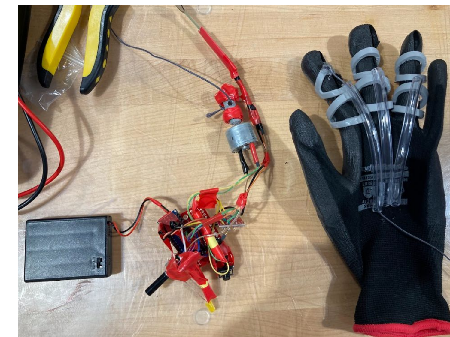
Fig 6. Final design components. Soldered electronics, 3.4V DC motor, and threaded glove.
