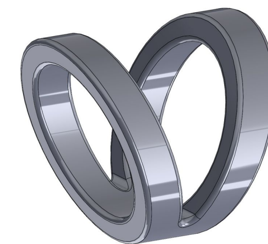
Fig. 4 SolidWorks rendering of finger braces. Used in duplicates to prevent over extension of the finger.
