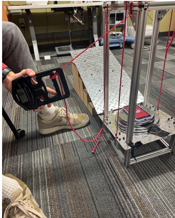
Figure 8: Required Force Testing with Load of 7.5 kg with Inclusion of Nylon
