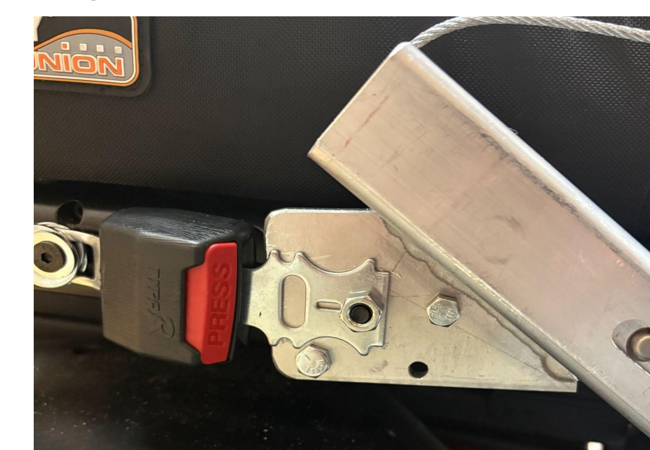
Figure 5: Side view of the wheelchair with the telescoping rod attachment and locking mechanism
