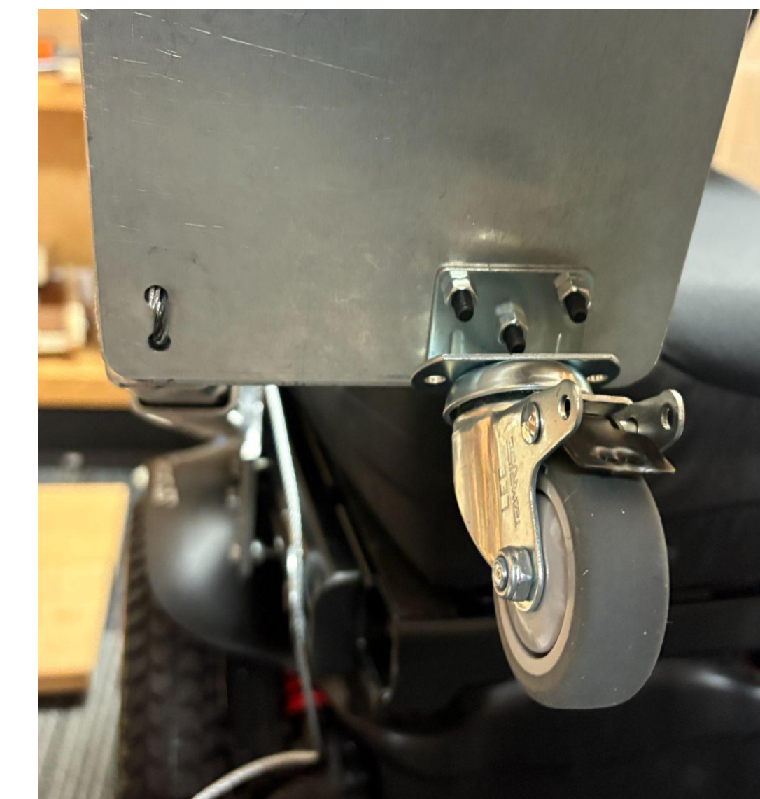
Figure 3: A bottom view of the footrest with the wheel attached.
